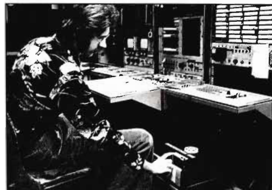
A director at WTAP-TV prepares to run some super 8 news film for the 6 o'clock news show. The videoplayer shown here, accepts up to 400 feet of film on standard super 8 reels or in Supermatic cassettes and delivers an electronic signal compatible with the station's switcher.
