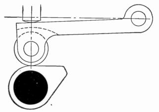
FIG. 7,031.—Valve cam device with roller mounted on cam. This design is frequently used to reduce the side-thrust upon the push rod.
