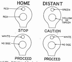
FIGS. 6,551 to 6,554 .- Indications of disc signals.
