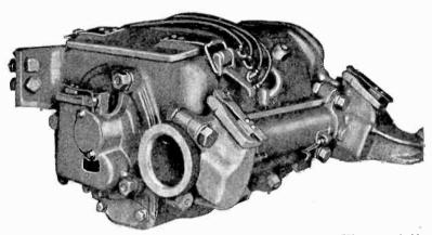
FIG. 6,161.—Westinghouse railway motor, 60 h.p.; 600 volts; 87 amperes, 770 r.p.m. suitable for light weight interurban cars where high running speeds are necessary, in double equipments on modern city cars and in quadruple requirements for trailer hauling. It is adaptable to all conditions requiring a 60 h.p. motor with 26 in. or 28 in. wheels.
