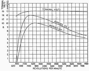
FIG. 7,101.-Typical charging curve with 3rd brush regulation.
