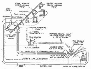
FIG. 6,667.—Diagram of complete switch control, indication and locking circuits; switch and lever in the normal position. The indicating system is in corresponding condition and the switch is unoccupied by trains and it; lever free to be operated.
