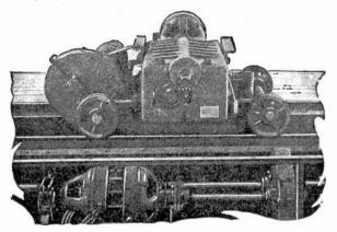
FIG. 6,885.—Euclid crane construction 12. Another view of moderate duty trolley. The illustration also shows the disc type electric brake that is located on the end of the motor shaft.
