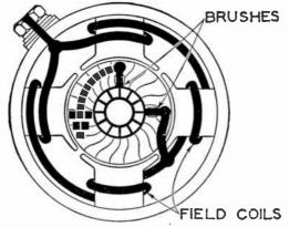
FIG. 7,093.-North East internal circuit of the starting motor shown in fig. 7,092.
