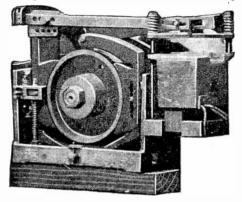
FIG. 6,870 .- Novo automatic set solenoid brake.
