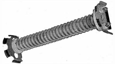
FIG. 6,485.—Consolidated heating unit for cross seat heater showing coil mounted upon porcelain spindle, the terminals for making connections and the steel end.
