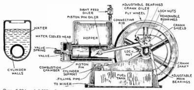
FIGS. 6,994 and 6,995.—Sectional views of Fuller and Johnson gas engine cylinder showing open jacket or "hopper" method of cooling. The hopper consists of a large vessel surrounding the cylinder, which holds a sufficient quantity of water to adequately cool the cylinder. The water circulation is by gravity.
