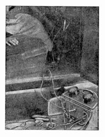
FIG. 7,067.-Testing ammeter with Allen trouble shooter.
