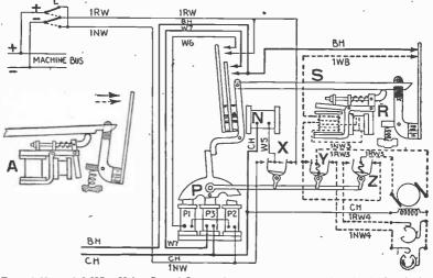
FIGS. 6,634 and 6,635.—Union S. and S. complete control and operating circuit for single switch.
