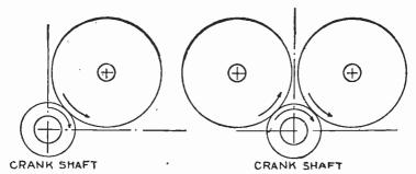
FIGS. 7,024 and 7,025 .- Diagram showing rotation of cam shafts with a direct gear device.
