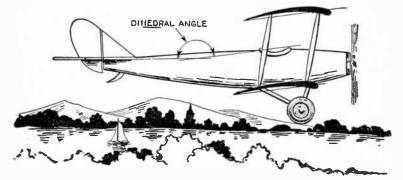
FIG. 7,144.—The dihedral angle. By definition a dihedral angle is that angle made by the intersection of two planes, as appued to the aeroplane it means the difference in angle of inclination of the wing and the stabilizer, that is the angle formed by the intersection of the wing and stabilizer surfaces projected along the axes.
