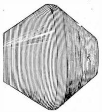
FIG. 6,871.—Allis-Chalmers cone drum. A development of the single cylindrical drum with two ropes is the double cone drum. This is another way of counter balancing the variable weight of the hoisting rope. The theory of this construction is that as the weight of the rope increases, the radius at which it acts correspondingly decreases, thus equalizing the work of the engine.
