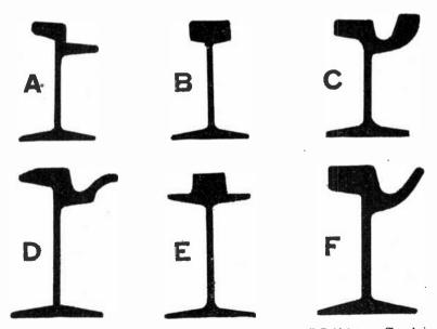
FIGS. 6,353 to 6,358.—Various girder rail sections. A, plain girder rail; B, high tee, or Shanghai rail; C, grooved girder rail; D, Trilby girder rail: E, center bearing girder; F, deep flange girder
