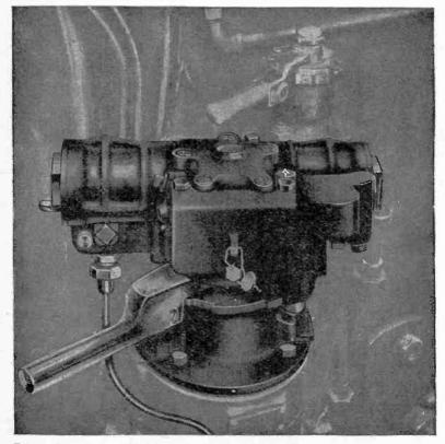
FIG. 6,722 .- Actuator applied to engineer's brake valve.
