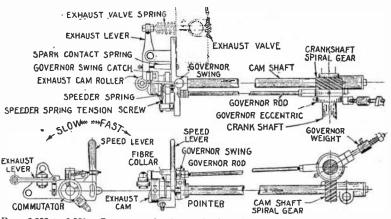
FIGS. 6,989 to 6,991 .-- Governor and valve mechanism of Domestic, type F, engine.
