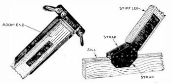
FIGS. 6,939 and 6,940.-Derrick fittings: 3. boom end for general work and stiff leg connection to sill with stiff leg straps.
