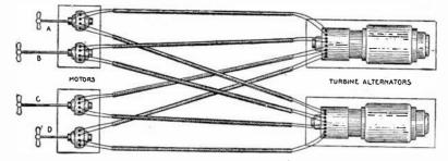
FIG. 7,154—Elementary diagram illustrating the essentials of electric ship propulsion. Two turbine alternator units are shown on the right which are wired for various connections with the motors; the latter operates the propellers A,B,C and D.
