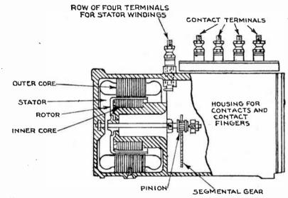
FIG. 6,610.—Polyphase relay. The motor windings are designed and connected so as to produce, with *a.c.* applied, a rotating magnetic field, which in turn induces currents in the nonmagnetic rotor causing it to operate. The rotor is ordinarily connected to operate the contact fingers through the medium of a pinion and sector arrangement, thereby multiplying the effect of the rotor and permitting the operation of a large number of contacts with a very small amount of energy applied.
