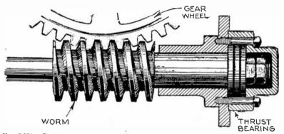
FIG. 6,771.—Single worm drive with ball bearing end thrust. The shaft on which the worm is cut is direct connected to the motor through a coupling with pulley shaped flange which is used as a braking surface. The single worm drive is suitable for relatively slow car speed and light loads. In construction worm drives are arranged to run in oil, accordingly the worm is placed below the gear wheel.
