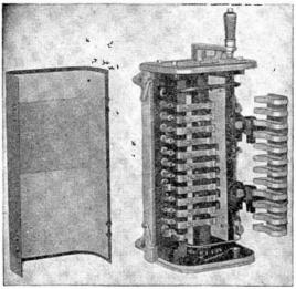
FIG. 6,893 and 6,894.—Euclid crane construction 18. Controller. It is of the drum type with fingers of the non-stubbing type. Both finger tips and contact segments are reversible. D.c. controllers are provided with powerful blow out coils to prevent injurious arcing.
