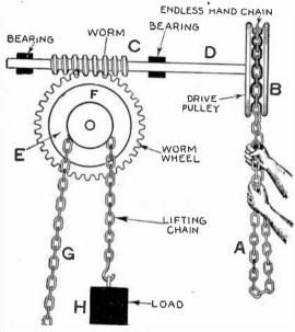
FIG. 6,848.—Evenentary worm gear hoist. The hand chain A, is used for rotating the drive pulley B, which is connected to the worm by a shaft. The worm meshes with the worm wheel E, whose shaft is attached to a pulley over which passes the lifting chain G. The pulley F, has pockets for receiving the chain links so that the chain cannot slip in lifting the load H.
