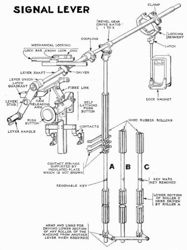
FIG, 6.629—Perspective diagram of signal lever showing relation of the various parts of a complete signal lever unit. The push button shown immediately under the lever handle provides for the operation of calling on signals.
