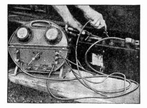
FIG. 7,065 .- Making battery test with Allen trouble shooter.
