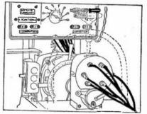
FIG. 7,079 .- Magneto test connections.
