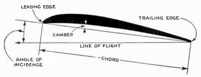
FIG. 7,109.-Wing main rib illustrating the terms camber, chord, angle of incidence.
