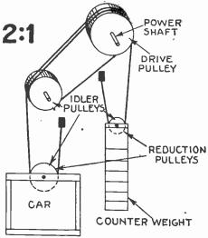
due to the weight of the car and counter-weight. The advantage of this system is its simplicity, and long rope life is claimed for it, due to the reduced number of bends and the absence of slippage between the ropes and the sheave. The disadvantage lies in the tendency of the sides of the grooves to wear down and reduce the grip on the ropes.
