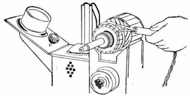
FIG. 7,061.—*Test for reversed current*. A reversed coil will give the same reading as a correctly connected coil, when read from bar to bar. To test for a reversed coil, place fingers on every other bar, adjust rheostat and test around. A reversed coil will neutralize the reading of a good coil and together they will give a very *low* reading.
