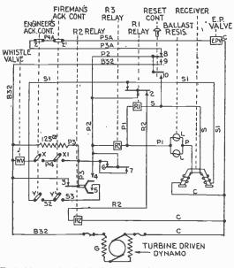
FIG. 6,731.—Typical locomotive circuit, forward running only, requiring acknowledgment by engineer and fireman.
