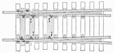
FIG. 6,360 .- Racor three throw split switch with adjustable rods.
