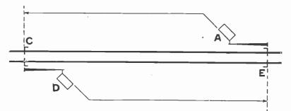
FIG. 6,585.—Signal arrangement which will alford certain protection for following movements, but not for opposing movements.
