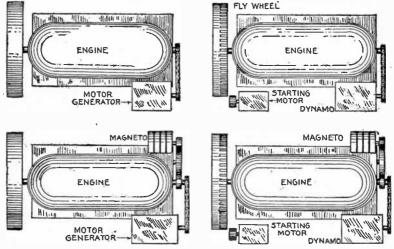
FIGS. 7,081 to 7,084.—Classes of starter systems. Fig. 7,081, one unit system; fig. 7,082, two unit system; fig. 7,083 so called two unit system; fig. 7,084, so called three unit system.
