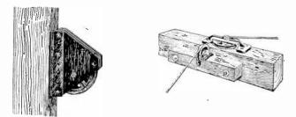
FIGS. 6,943 and 6,944.—Derrick fittings: 5. mast brackets used with derricks operating clam shell and orange peel buckets, and guide sheares for bull wheel line.
