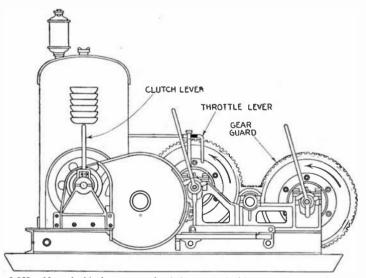
FIG. 6,869.—Novo double drum gas engine hoist powered with tour cylinder radiator cooled engine. It will handle two large material elevators. Some contractors have this hoist fitted with an 18 in. or 22 in. diameter drum to handle concrete tower bucket with high speed and a standard drum to handle "Chicago" derrick or miscellaneous steel or platform elevators.
