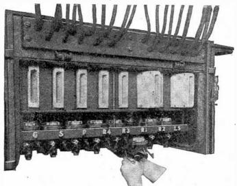
FIG. 6,280.-Westinghouse control operation 6. Taking out a cylinder and magnet valve.
