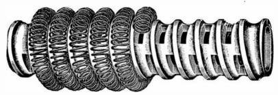
FIG. 6,487.—Ventilated porcelain core partially wound with resistance wire. The perforations in the porcelain core increase the radiating surface of the support, therefore the air passing through the supports and coils as well as around them give an efficiency not found where solid supports are employed. rod, on which are strung porcelain tubes which are so designed and fitted that a helical groove extends from end to end.
