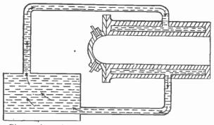
FIG. 6,993.—Diagram of a gravity water circulation system for a gas engine cylinder. As indicated by the arrows, the water from the tank enters the jacket of the cylinder at the lowest point, and being there subjected to the heat of the cylinder walls, rises to the level of the tank water; thus maintaining a continuous circulation.
