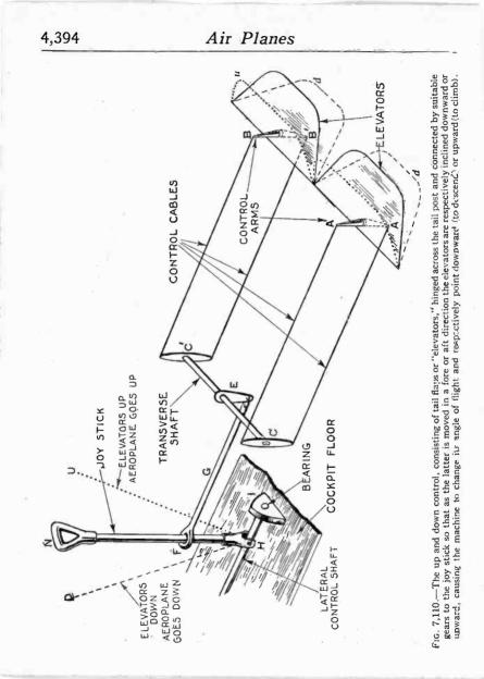
Each elevator has two control arms AA' and BB', connected by cables to the arms C and C', the latter being attached to a transverse shaft. Keyed to the center of this shaft is an arm E, which is connected to the joy stick at F, by the rod G.
