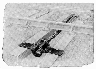
FIG. 6,415.—Racor retarding dash pot for use on spring switches. *This device*, working in non-freezing oil, retards the closing of switch points so that they will not snap shut between successive pairs of wheels when trailing through. Makes spring switches practical for steam roads, and is especially useful at passing sidings on electric railways. Saves wear and *ear* on switch points.
