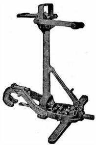
FIG. 6,420.—Moore track drill, for drilling holes in track rails, for bonds or splice plates. It is operated by worm gears and feeds the drill automatically; the advance of the drill being 1 in, for every 50 to 650 revolutions depending on the adjustment and the softness or hardness of the rail.
