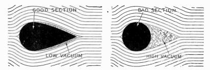
FIGS. 7,139 and 7,140.—Good and bad cross sectional shapes of struts. In fig. 7,139, the long easy curve permits the air to follow the surface, thus practically no vacuum is formed; while in fig. 7,140, the air cannot follow the abrupt curve resulting in a vacuum which acts as a drag or resistance opposing its advance.
