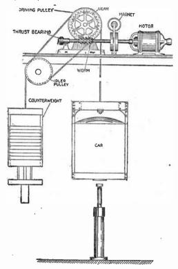
For higher speeds, over 500 f.p.m. and sometimes for speeds 500 f.p.m. and below, the hoist ropes lead around the traction sheave for another half wrap and so down to the counter weight, as in figs. 6,752 and 6,756.
