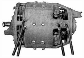
FIG. 6,123.-General Electric motor for gas electric double motor drive.
