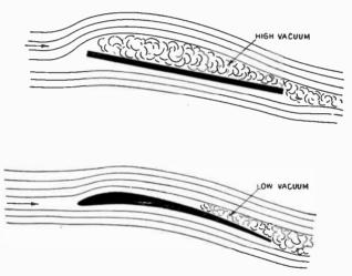
FIGS. 7,105 and 7,106 -Flat and curved wing surfaces and their effect on the air,
