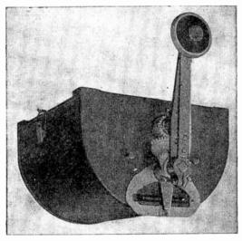
FrG. 6,800.—Westinghouse variable voltage control system 5. Car slow shows switch. This limit switch similar in construction to the landing switch is mounted on top of the car. An operating arm actuated by properly located cams, opens and closes the control circuits, causing the car to automatically slow down and stop at the extreme limits of travel. Where the power supply is alternating, the motor generator set of the variable voltage system has a direct connected exciter, to supply a source of
