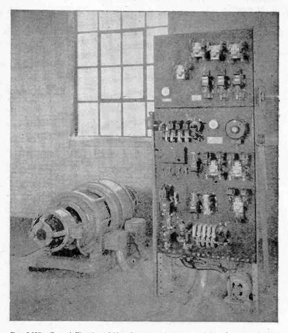
FIG. 6,807.—General Electric variable voltage control system consisting of a motor dyname set and controller for elevator having automatic leveling devices.
