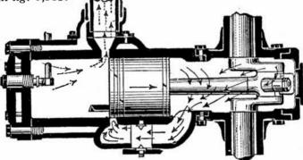
FIG. 6,986.—The two cycle engine: *first part of second stroke*. The outward stroke of the piston uncovers the exhaust port, thus releasing the burnt gases in the cylinder, and simultaneously compressing the previously admitted charge in the crank case.
