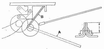
FIGS. 6,457 and 6,458.—Method of pulling on belt. To put on the belt, swing the dynamo toward the truck, with the dynamo pry A, and block in upper position by wood piece B (20 ins. by 3 ins. by  $\frac{7}{6}$  ins. standard width).
