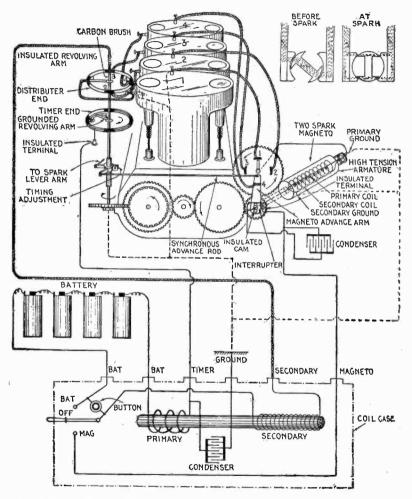
FIGS. 7,003 to 7,005.—Double ignition consisting of a two spark high tension magneto system and a battery synchronous ignition system with engine driven distributer. Fig. 7,003, elementary diagram of connections; fig. 7,004, position of magneto armature just before time of spark; fig. 7,005, position of armature at time of spark.
