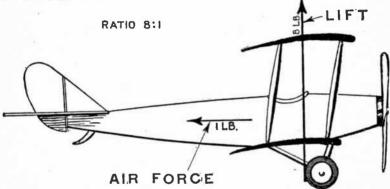
FIG. 7,143.—The lift, air force ratio. If for each 1 lb. of resistance (air force) overcome by the forward thrust of the propeller the upward pull or lift be, say 8 lbs., then the lift, air force ratio is 8:1.
