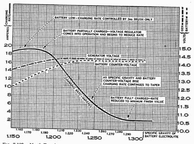
FIG. 7,102.—North East battery charging curves. When voltage regulation is used, the dynamo output gradually reduces as the battery becomes charged.
