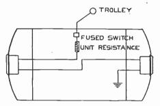
FIG. 6,483.—Head light wiring diagram for mine locomotives. 2, double end equipment, both head lights burn at same time, circuit voltage greater than that of combined lamps.
