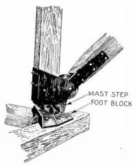
FIG. 6,936.—Derrick fittings: 1. foot block and mast step irons, showing lock at the rear of the ball and socket joint. There are two sheaves in the foot block and one in the mast step. The sheave in the mast step is not required for stiff leg derricks. Special foot blocks and mast steps are required for handling clam shell or orange peel buckets and other three line work.
