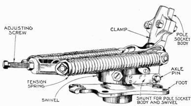
FIG. 6,194 — Nuttall roller bearing trolley base for interurban or city service. This base is supplied with copper shunts which connect the pole socket axle pin to the swivel casting and obviate the necessity of carrying current through the bearing. Its wheel pressure increases as the pole approaches the perpendicular.
