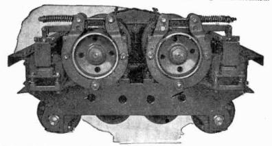
FIGS. 6,909 .- Milwaukee shoe type solenoid motor brake. The shoes are lined with astestos.
