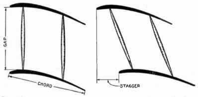
FIGS. 7,107 and 7,108.—Method of connecting wings by struts and diagonal bracing, illustrating the terms chord, gap and stagger.
