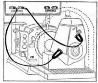
FIG. 7,072 .- Buick motor generator connections.
