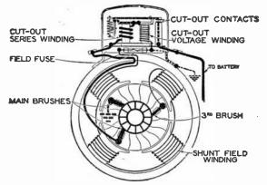
FIG. 7,091.—North East dynamo internal circuits; 6 volt, 4 pole, 3rd brush regulation, reaction type brushes, †CW, rotation. No binding posts. Grounded internally through main brushholder. Dynamo lead connected to cut-out on field frame. Fuse 6 amps; mounted on base of cut-out. Cuts in 7.5 volts, 450 r.p.m. Standard output setting 15 to 16 amps (hot) at 1,200 r.p.m. Rated capacity 125 watts. This shows the internal circuits of fig. 7,090.
