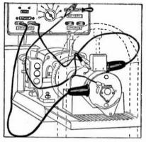
FIG. 7,074 .- Discriminating cut out or reverse current circuit breaker on generator.
