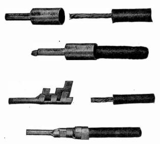
FIGS. 6,492 to 6,497.—Gold service wire tips. These prevent the open circuiting of the wire at the terminals due to vibration at the point of contact; also eliminates frayed edges of the insulation. In attaching type shown in figs. 6,492 to 6,494, the wire is sweated into the ferrule, allowing about  $\frac{1}{3}$  inch of the bare wire to extend beyond the end of the tip, which end is dipped in solder, making a positive connection. Figs. 6,495 to 6,497 show the clamp type.
