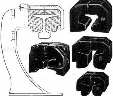
FIGS. 6,196 to 6,200.—Ohio Brass third rail support and insulator, for under contact operation. This is used in open roadways where snows may be heavy and it is necessary to have greater distance between the live rail and the ground. The shoe slides under the rail instead of on top of it as in subways or other protected places.
