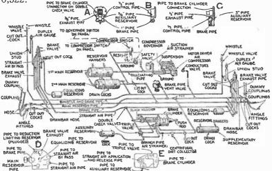
Fros. 6,317 to 6,322.—Westinghouse combined automatic and straight air brake equipment diagrams showing parts and pipe connections. Figs. A, B, C, show pipe connections to brake cylinder pressure head; fig. D, pipe bracket of brake valve; fig. E, pipe double check valve.
