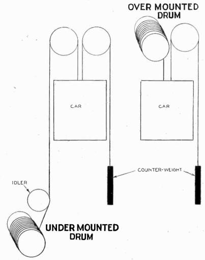
FIG. 6,747.—Under mounted drum elevator. FIG. 6.748.—Over mounted drum elevator. With respect to location, there are two types of machine, known as:
