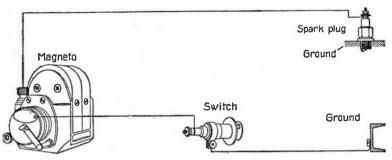
FIG. 7.053.—Bosch high tension magneto for one cylinder engine. For this service the revolving high tension magneto does not require a distributer because the high tension current is conducted directly to the spark plug from the secondary winding by way of a slip ring (collector) and a brush holder. A one cylinder magneto has only one cam in the interrupter housing.
