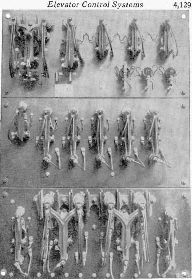
FIG. 6,792 -- Gurney d.c. rheostatic controller for the d.c. motor illustrated in fig. 6,791.
