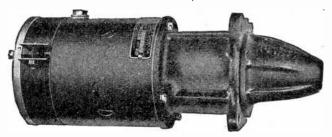
FIG. 7,092.—North East starting notor as used on Dodge Bros. cars, 6 volt, flange mounting. CW rotation, Bendix drive, right hand thread, 10 tooth pinion, 8-10 pitch, outboard bearing. 1 binding post only, located at commutator end of field frame, and milled flush with nut <sup>11</sup>/<sub>4</sub> " above frame. Grounded internally through brush holder. Maximum torque (stalled) 13.5 pd, ft, at 550 amps. and 3.2 volts.
