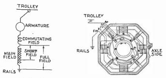
FIGS. 6,159 and 6,160.-Diagrams of field control motor.
