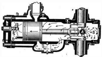
FIG. 6,985.—The two cycle engine: *first stroke*. The inward stroke of the piston induces a charge of the mixture at A into the crank case B, and compresses the previously admitted charge into the cylinder D; the subsequent ignition takes place at E.
