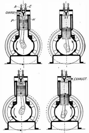
FIGS. 6,978 to 6,981.—The four cycle method of operation. Fig. 6 978, admission stroke; fig. 6,979, compression stroke; fig. 6,980, power stroke; fig. 6,981, exhaust stroke. A, is the admission valve: E. exhaust valve; N, negative electrode; P, positive electrode of igniter.
