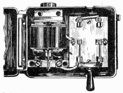
FIG. 6,437.—Consolidated relay and charging switch for emergency car lighting system The relay and charging switch is for automatically charging auxiliary car lighting battery from trolley and for automatically cutting in a group of lamps on a battery circuit
