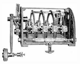
FIG. 6,839.—Westinghouse hoistway or terminal cam type limit switch. In construction the shaft carries moving cums that operate contacts located on a number of semi-circular supports inside the case. These contacts can be moved to allow adjustment of slow down and stopping position. The main operating shaft is actuated by an arm with a rubber tired roller which engages a cam suitably located in the hatchway. All movements of the switch are extremely quiet.
