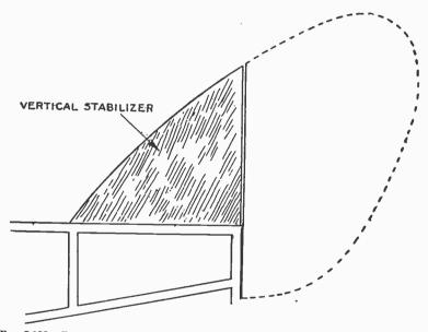
FIG. 7,126.—Rear vertical stabilizer or fin, to secure stability against skidding by resisting the skid, giving a banking effect, also to damp out the directional oscillations due to response to rudder, and to overcome centrifugal force, or tendency of the tail to skid outward in making a turn.
