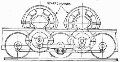
FIG. 6,168.—Method of mounting locomotive motors with both gears and connecting rode. The drive is through a form of Scotch yoke and side rods as shown.
