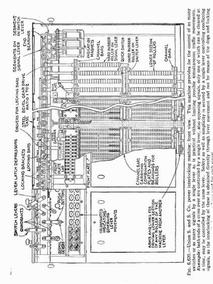
which the signal governs train movement, shall be in proper position and locked. To secure such protection for train movement it is desirable to concentrate the control of the various switches and signals at one point. The mechanism in which this concentration of control is secured is called an interlocking machine, as shown in figs. 6,619 and 6,620.
