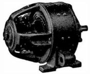
FIG. 6,778.—General Electric d.c. ball bearing elevator motor with cartridge type housing. The construction of the housing for oil lubrication differs somewhat from that employed for grease lubrication. The latter type is here shown.
