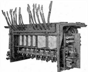
FIG. 6,276.—Westinghouse control box with covers removed showing overload trip relay and front side of switch group.
