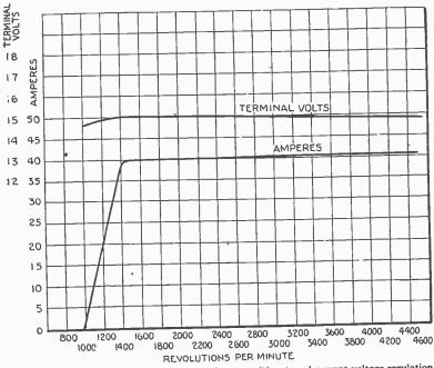
FIG. 7,103.—Charging curve of shunt wound dynamo with external current voltage regulation.
