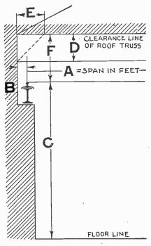
FIG. 6,922.—Section of shop showing information required in selecting a crane. Load, maximum in net tons; speed, if special for any function be preferred; style, outside or inside service; current data, whether d.c. or a.c., giving voltage cycle and phase; clearance dimensions, A, span; B, end clearance; C, distance from top of rúnway rail to floor; F, overhead clearance.
