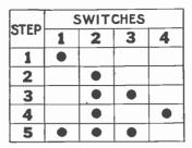
FIG. 6,234.—Diagram showing sequence of operation of the switches in the hook up shown in fig. 6,233.
