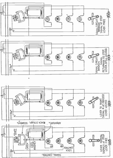
Fics. 6,677 to 6,680.-Diagram of signal lever and circuits for selecting opposing signals.
