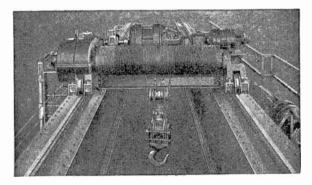
FIG. 6,877.—Euclid crane construction 4. Another view of mill type trolley showing track wheel bearings. The drum is scored right and left hand, so that the load is always equally distributed on both girders. This cut also shows the separator girt connecting the two side frames.
