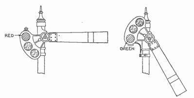
FIGS. 6,515 and 6,516.—Two position *home* signal. Note shape of arm or "blade." The front of it is usually painted red with a white stripe near its outer end and the back of it white with a black stripe near the end.
