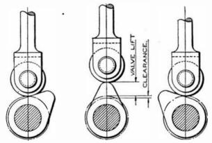
FIGS. 7,028 to 7,030.-The successive positions of a valve lifting cam.
