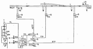
FIG. 6,653 .- Sectional route locking circuit.
