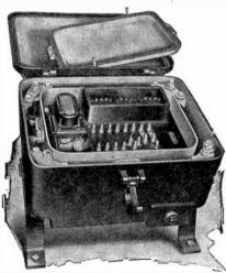
FIG. 6,726.—Locomotive relays and housing. It will be noted that the relays and lamps together with their terminals, are mounted in an inner case which is floated on heavy springs and equipment with snubbers. The three relays are mounted on one base and the contacts are protected by a cover which has a glass top. The ballast lamps are protected by a wire mesh cover shown to the left of relays.
