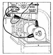
FIG. 7,073 .- Independent cut out connections.
