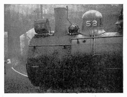
FIG. 6,469 .- Westinghouse 500 watt head light unit installed in locomotive.
