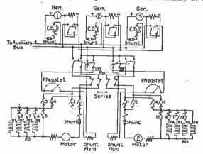
FIG. 7,176.-Typical rheostatic or armature control circuit diagram.
