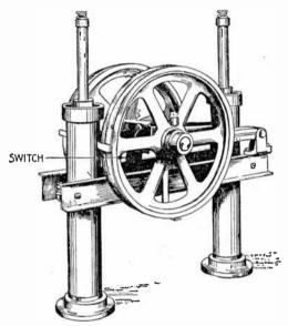
FIG. 6,842.—Elevator compensating rope sheaves with switch.
