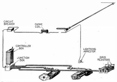
FIG. 6,256.—Westinghouse single end type K control equipment.
