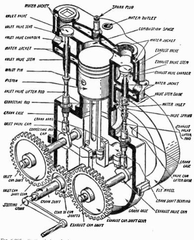
FIG. 6,965.—Sectional view of a four cycle gas engine, showing the valve gear and other working parts. Both inlet and exhaust valves are mechanically operated. The location of the valves diametrically opposite each other requires a separate cam shaft for each. These com shafts are geared to the engine crank shaft and they make one revolution to every two of the engine. When the inlet valve is operated by a spring and the engine suction, or (r) = can shaft is necessary, as shown in fig. 6,967.
