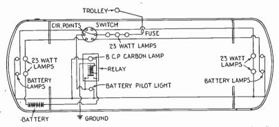
FIG. 6.442.—Electric S. S. Co. wiring diagram for double end car using relay having pilot light, indicating disconnection or failure of storage battery, for operating two rear end signal lamps with switch connections for double end operation.
