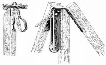
FIGS. 6,937 and 6,938.—Derrick fittings: 2. mast top irons. Fig. 6,937, irons with spider plate for guy derricks; fig. 6,938, irons with goose necks for stiff leg derricks. Iron cone complete with block, pin, shackles, back plate and bolts as shown.
