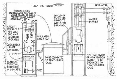
FIG. 6,432.—Subway lighting equipment showing the parts and the arrangement of the apparatus on the switchboards and the methods of connecting.
