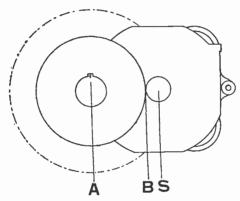
FIG. 6,169.-Diagram for laying out locomotive motor gears.
