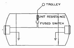
FIG. 6,482.—Head light wiring diagram for mine locomotives. 1, double end equipment, circuit voltage greater than head light lamp voltage; each lamp burns singly.
