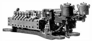
FIG. 6,183.-Westinghouse electro-pneumatically operated reverser for locomotives.
