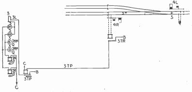
FIG. 6,651 .- Section locking circuit.
