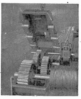
FIG. 6,878.—Euclid crane construction 5. Hoisting gear train. Wide face coarse pitch gears are used. The illustration also shows the shoe type electric brake mounted on the motor shaft and the Weston type mechanical load brake on the intermediate shaft.
