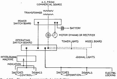
FIG. 6,618.-Diagram of power supply d.c. interlocking.
