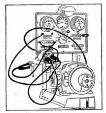
FIG. 7,076.-Coil testing connections.
