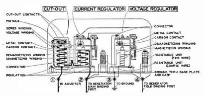
FIG. 7,088 .- North East three element control unit.
