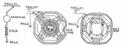
FIGS. 6,147 to 6,149.—Electric circuits of the simple series motor. As shown in these illustrations the motors have four poles and the armature winding is of the two circuit wave length which permits the use of only two sets of brushes, makes cross connections unnecessary, requires the fewest number of turns per coil, the largest and therefore strongest conductors, and the least voltage per coil. The majority of railway motors still in service are of this type.
