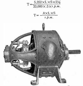
FIG. 6.777.—Exterior view of Westinghouse d.c. elevator motor. To secure good commutation and quiet running interpoles are used and the armature provided with a large number of slots; also the main poles are beveled.
