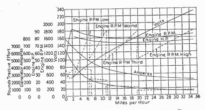
FIG. 6,118.—Comparison of characteristics of gas electric and mechanical drives. The curves show engine characteristics and tractive effort at the rim of the wheels, obtained with a typical gas electric drive application, compared with that of a mechanical drive bus equipped with a prime mover of the same capacity.
