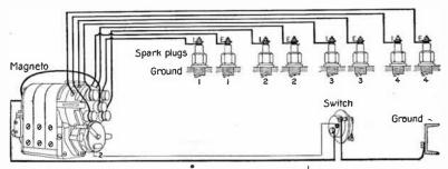
FIG. 7,056 .- Bosch high tension two spark magneto for four cylinder engine.
