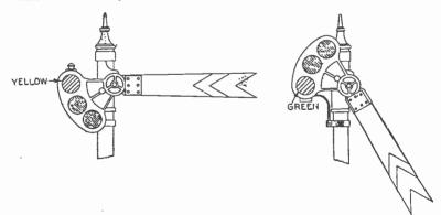
FIGS. 6,517 and 6,518.—Two position *distant* signal. The distant blade is made with a V shape or fish tail end. The front of it is generally painted yellow with a black stripe parallel with the end of the blade, or green with a white or red stripe. The back of the blade is painted white with a black stripe. A few roads that do not use this notation, paint the front of all blades yellow with a black stripe and the back black with or without a white stripe.
