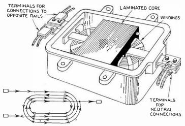
FIG. 6,599 .- Impedance bond with cover removed.
