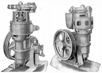
FIGS. 6,765 and 6,766.—A. B. Sce single wrap traction elevator machine. Fig. 6,765 for d.c. fig. 6,766 for a.c. It is designed especially for installation in locations where the space is limited. In order to obtain these small overall dimensions the driving motor has been placed in a vertical position and the brake placed above the outboard bearing of the motor instead of between the motor and the worm gear housing as in general practice.
