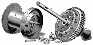
FIGS. 6,856 to 6,862.—Loose drum and friction control before assembly. The parts are: A, shaft; B, friction blocks; C, block retainers; D, drum; E and F, friction rings forming a V groove on drum flange; H, winch head or spool; I, collar; J. thrust collar; L, thrust pin; N, washers.
