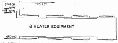
FIG. 6,503.—Connections of single unit heaters for seats running longitudinally in a car. Note staggered connections. Throwing in one switch sends current through one-half the number of heaters, but uniformly distributed.
