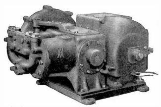
FIG. 6,188.-Westinghouse motor driven air compressor for locomotive.
