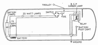
FIG. 6,440.—Electric S. S. Co. wiring diagram for single end car, using relay with pilot light, for operating two rear end signal lamps. Relay pilot light indicates disconnection or failure of battery.
