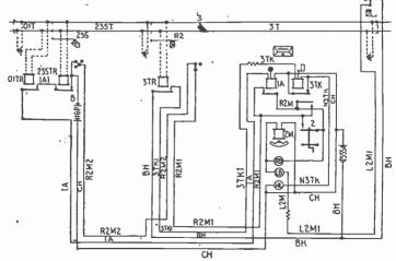
FIG. 6,654.-Approach locking circuit.
