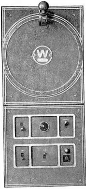
Car Operating Switch.—This switch, shown in fig. 6,834, usually has the automatic return or self centering feature so that if the operator's hands be removed from the lever it will return to the off position. It is also usually provided with a center latch so arranged that any accidental leaning against the switch will not move the lever to the running position.
