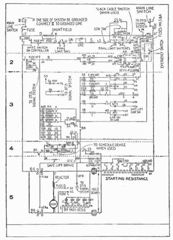
FIG. 6,829—Otis d.c. resistance controller for use with gearless traction machine, car switch operated with safe lift 1A, 2A, reversing switch; B, brake switch; C, potential switch; E, F, G, H, speed switches; 1D, 2D, 3D, 4D, accelerating sws; I, field switch; S, door contact relay; Q, load switch; AA, reversing sw. relay; EE, 1st speed sw. relay; GG, 3rd speed sw, relay, 01, overload relay; FF, 2nd speed sw. relay; BB, brake relay; DD, safe lift relay.
