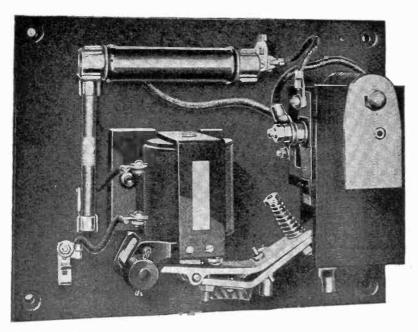
FIG. 6,512.—Gold automatic switch. It is magnetic and performs the two fold function of opening and closing the circuit through which the heating coils are supplied, and of controlling the circuit from the thermostat so as to enable the thermostat to operate without sparking or arcing.
