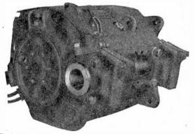
FIG. 6,175 .- Typical mine locomotive motor.
