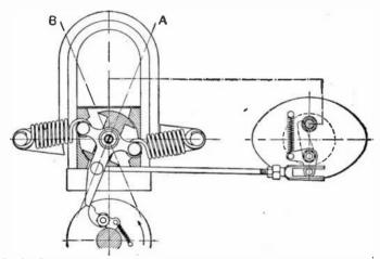
FIG. 7,043.—Timing diagram for oscillating type low tension magneto 2. Magneto trip lever near position of release.
