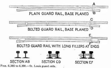
The curve guard rail is installed on the sharper curves to avoid derailment and to reduce side wear of rail and flanges. The bridge guard rail is intended to keep derailed wheels from running off the ties.
