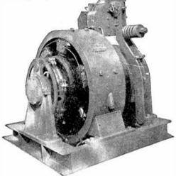
FIG. 6,790.—General Electric all steel roller bearing gearless elevator motor. In a gearless machine the traction sheave is mounted on the armature shaft or spider and turns at the same speed as the armature, which must develop full power at a low speed of revolution. For example, if the sheave be 36'' diameter and the elevator speed 700 f.p.m. the motor armature must run at approximately 75 r.p.m.
