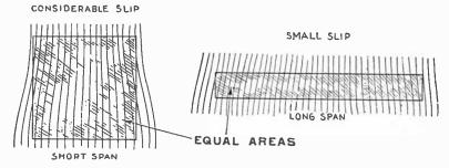
FIGS. 7,137 and 7,138.—Wings of short and long span (low and high aspect ratio) showing why the long wing is the more efficient. Wing tips are inefficient because they "spill," or allow the air to slip sideways past their ends, hence in a long span wing as in fig. 7,138 the end portion or tip is only a small percentage of the total area, and accordingly little air slips hy the tips as compared with a short span wing which has a wide tip.
