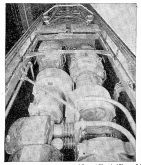
UIG. 6,164.—Auxiliary machinery compartment of General Electric 150 ton, 3,000 volt d.c. locomotive.
