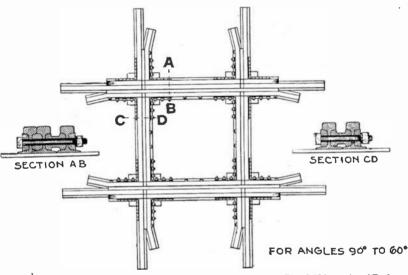
$F_{IGS},\,6,395$  to 6,397.—St. Louis crossing, three rail one track. Fig. 6,395, section AB; fig. 6,397, section CD.
