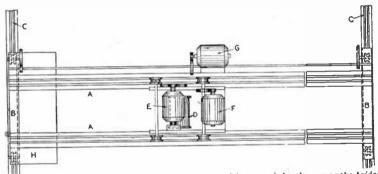
FIG. 6,895.—Electric traveling crane. The parts are: AA, cross girders known as the bridge; BB, end carriages; CC, elevated track structure or gautries; D, hoisting drum; E, hoisting motor: F, transverse propelling motor; G, longitudinal propelling motor; H, cage or operator's platform.
