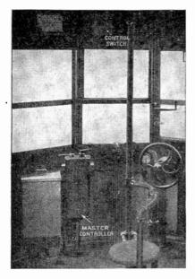
FIG. 6,282.—Interior of operator's cab showing Westinghouse master controller and control switch. The master control is for electro-pneumatic control of motors in modern heavy traction cars. Heavy Inspection. — A heavy inspection in general should be made about every three to six months where cars are regularly in service.
