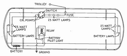
FIG. 6,441.—Electric S. S. Co. wiring diagram for double end car, using relay with emergency lighting circuit for operating two rear end signal lamps with proper switch connections for double end operation.
