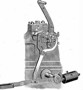
FIG. 6,867.—Lidgerwood brake and friction levers with safety attachment. When the friction lever A, is moved to throw the drum into gear, the pin I, on a projection of the friction lever presses against the curved part of the oscillating lever C, and releases the foot brake.
