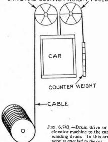
FIG. 6,743.—Drum drive or method of transmitting power from the elevator machine to the car by means of winding the hoist rope on a winding drum. In this arrangement the end of the counter weight rope is atlacked to the car.
