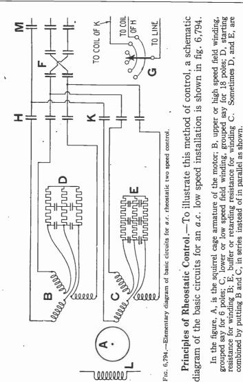
F, is a reversing device, usually two double pole magnetic switches, called direction switches, whose coils are energized by contacts (not shown) on car switch G; G, car switch with contacts for energizing the coils of the low speed switch, K, and the high speed switch H.
