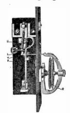
FIGS. 6,509 and 6,510.--Gold thermostat. Fig. 6,509, outside view; fig. 6,510, case and element guard removed.
