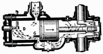
Fig. 6,987.—The two cycle engine. end of the second or outward stroke. The gases compressed in the crank case are admitted to the cyl nder space D, through the open inlet port, and sometimes past the screen or deflector, C. The passage between the cylinder and the crank case is controlled by a butterfly valve, which here, is shown open.
