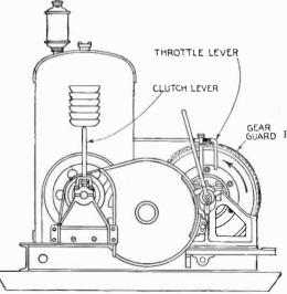
GUARD FIG. 6,852 .- Novo gas engine driven hoist powered with four cylinder engine, radiator cooled. The engine has two fly-wheels, which approximates steam engine flexibility. With an engine equipped with two flywheels, when handling a concrete tower elevator, the engine may be throttled and the load will float to the proper stopping point without stalling the engine. This makes faster and more efficient hoisting.
