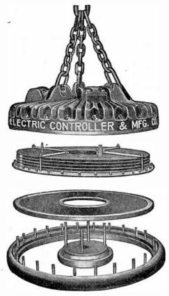
FIGS. 6,953 to 6,956.—Electric Controller lifting magnet disassembled showing coil wound on spider, outer bottom plate of manganese steel and renewable pole shoes held with through bolts.
