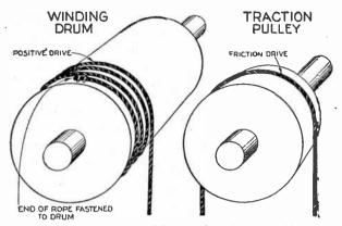
FIGS. 6,741 and 6,742.—The two types of drum used on elevator machines. In construction, grooves (not shown) are provided on both types of drum, the grooves being spiral for drum elevators and straight for traction elevators.
