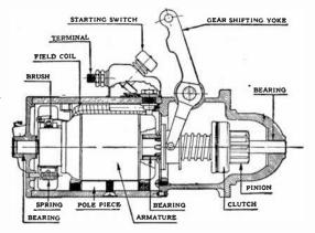
FIG. 7,087.-North East starter showing details.
