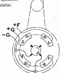
FIG. 6,461.-Diagram of field coil connections of safety C. H. & L. "axle" lighting system.
