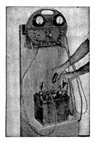
FIG. 7,064.-Allen trouble shooter installed for shop testing.
