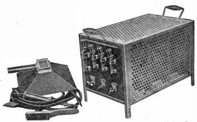
FIGS. 6,422 and 6,423.—Ohio electric arc welding machine designed for portable *d.e.* railway welding service. The resistance consists of individual units, so designed as to afford support and protection to the coils. The output is adjustable in 30 ampere steps. from 30 to 120 amperes.
