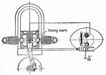
FIG. 7.042.—Timing diagram for oscillating type low tension magneto 1. Igniter shaft in contact with stationary pin.
