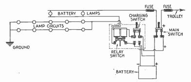
FIG. 6,436 .- Diagram of storage battery emergency car lighting system.
