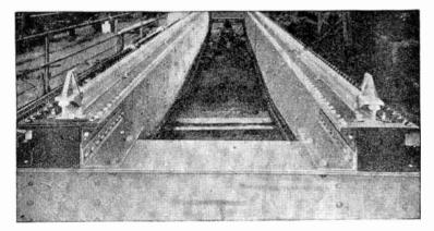
FIG. 6.874.-Euclid crane construction 1. Double web box girder bridges. The girders are reinforced by means of channel diaphragms at close intervals. The end trucks are of the box type, made up of heavy channels and plates. The illustration shows the way the girders are notched out and rest upon the top of the end trucks.
