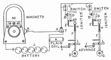
FIG. 6,997.—Method of low tension or make and break ignition. In operation, as the nose of the cam G, passes rod F, the latter suddenly drops by the action of spring H. The head of the rod, which has been raised by the cam somewhat above the arm of D, will in its descent strike D, a blow which abruptly breaks contact between D and B, thus producing an arc. When not acted upon by the head of the rod F, D, is held in contact with B, by the spring E. The system is explained in detail in the text.
