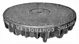
FIG. 6,958.—Electric Controller lifting magnet showing bottom plate to render the magnet moisture proof. The inner brass bottom plate hermetically seals the coil cavity.
