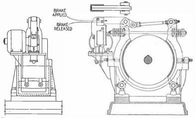
FIGS. 6,762 to 6,764.-American torque type brake.
