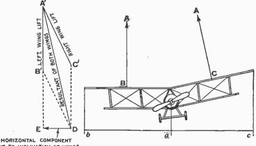
DUE TO INCLINATION OF WINGS
