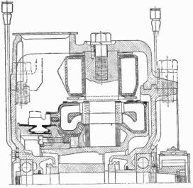
FIG. 6,176 .- Top half of extremely narrow gauge motor.
