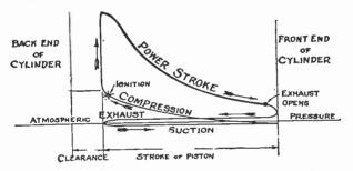
FIG. 7,013.—Charter oil engine indicator card or graphic representation of the pressures in the engine cylinder on the back end of piston. It is practically correct except that the exhaust and suction lines are shown at exaggerated differences from atmospheric pressure.
