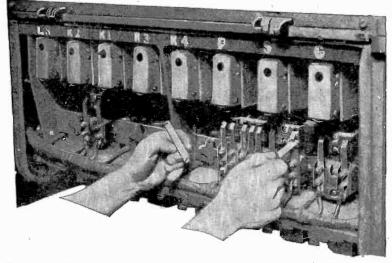
FIG. 6,296 .-- Westinghouse control operation 8. Adjusting interlock fingers.
