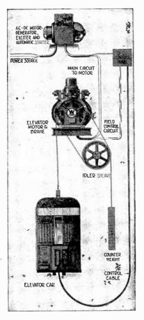
constant voltage direct current for the traction motor, the brake solenoid and the control magnet coils.
