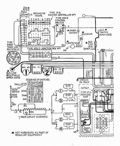
F1GS. 6,290 to 6,293,--Wiring diagram for Westinghouse standard 600 volt type HL unit
