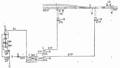
FIG. 6,652 .- Sectional route locking circuit.
