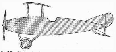
FIG. 7,124.—The side surface of an aeroplane, being the projected area of everything visible as viewed from the side, it is the effective surface upon which the wind may act from the side. The term keel surface is frequently and ill advisedly used for side surface.
