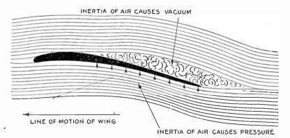
FIG. 7,133.—Section of wing illustrating *lift* as caused by *inertia* of the air in causing upward pressure on the lower surface, and partial vacuum on the upper surface of the wing.
