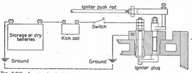
FIG. 7,040 .-- Low tension ignition system showing igniter and wiring connections.
