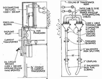
FIG. 6,429.—Subway lighting equipment. Side view of high tension switchboard showing cable connections to high tension knife switches, current transformer, oil circuit breaker, etc., and the mounting of the switchboard as related to the wall.
