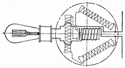
FIG. 6.433.—Lamp with compensating resistance relay. The line current goes through a solenoid which is in series with the lamp and energizes it and causes it to attract an armature. Removing the lamp or the lamp burning out, breaks the circuit and the armature drops onto two contacts, shunting the lamp and throwing its equivalent resistance into the circuit.
