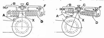
FIG. 6,447.—Position of dynamo with tension spring when distance between the axle pulley and suspension frame is shortened.
