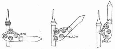
FIGS, 6.522 to 6.524.—Three position upper guadrant signal. Where both square and pointed blades are used, the pointed end blades indicate stop and proceed at low speed when the signal indicates stop. Stop and stay is always the stop indication at interlocking plants. Three position blades have the front side painted red with a white stripe parallel with the end or yellow with a black stripe. The back side is painted white with a black stripe, or black with or without a white stripe.
