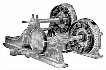
FIG. 6,853 .- Mead-Morrison arrangement of frictions and brake for gasoline or electric hoists.
