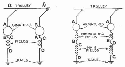
FIG. 6,246.—Diagram showing connections for forward and backward operation. At *a*, brush A, is connected to the trolley and brush B, to the positive side of the field. At b, the brush B, is connected to the trolley and A, to the positive side of the field. The negative side of the field is permanently connected to ground and the armature has been reversed. This is the standard method of reversing used with motors which do not have commutating poles.
