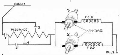
FIG. 6,233.—Diagram of two motor equipment showing series and parallel resistors. The sequence of operation of the switches in this case is indicated in fig. 6,234.
