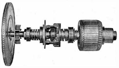
PiG. 6,473.—Keystone rotating element, showing wheel, bafile fan, governor, including oiling disc, safety spring, ball bearings and armature, mounted on the shaft.
