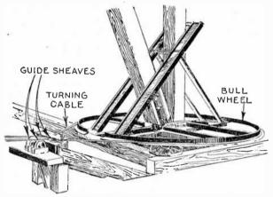
FIG. 6,945.—Derrick fittings: 6. bull wheel and guide sheaves. The wheel is made in halves and may be conveniently erected without unstepping the mast. The ring is a heavy angle iron with the vertical leg rolled with an appreciable outward flare which eliminates any tendency for the line to climb. An inverted movable section of the ring is placed under the boom which makes it a full circle. The braces which drive the boom are made of steel beams, and sills of heavy angles.
