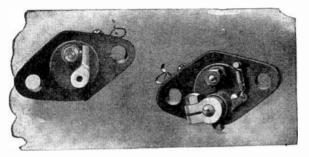
FIGS. 7,047 and 7,048.—Charter oil engine igniter. The igniter lever is operated from the cross head; a spark shifter permits of two ignition positions, one to produce a late spark when the operator is starting the engine, and the other for early or running spark.
