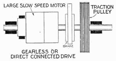
FIG. 6,739.—Elementary elevator machine with gearless or direct connected drive. A large slow speed motor is required.
