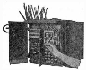
FIG. 6,272.-Westinghouse control operation 1. Cutting out motors.
