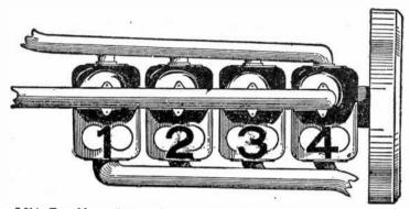
FIG. 7,014-Top of four cylinder engine showing numbering of cylinders.
