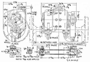
FIGS. 6,151 to 6,155.—Westinghouse box frame commutating pole direct current railway motor details.
