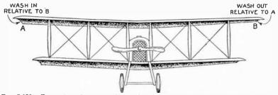
FIG. 7,130.—Front view of aeroplane illustrating the terms wash in and wash out which mean respectively the increase and decrease in the angle of incidence of the wings from the center toward the tips.
