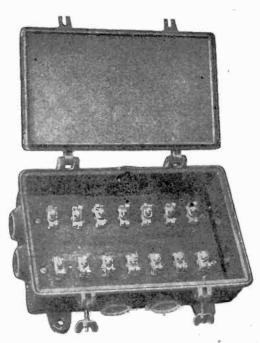
FIG. 6,268 .- Westinghouse train line junction box open.
