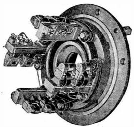
FIG. 6,460.—Safety C. H. & L. pole changer brush rigging. The direction of current from the dynamo is kept constant by rotating the brushes through an angle of 90° whenever the direction of rotation of the armature is changed. The pole changer may be taken off the head by springing out from its groove the snap ring which holds it on.
