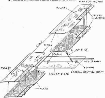
FIG. 7,113.—The lateral control. It consists of movable flaps, hinged to the trailing side of the wings at the ends as shown, and connected to the joy stick by suitable cable and pulley gearing. The gear is so arranged that the flaps on one side move in an opposite direction to those on the other side. On some machines only the top wing is provided with flaps.
