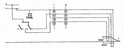
FIG. 6,640.-Signal control circuit for converging routes.
