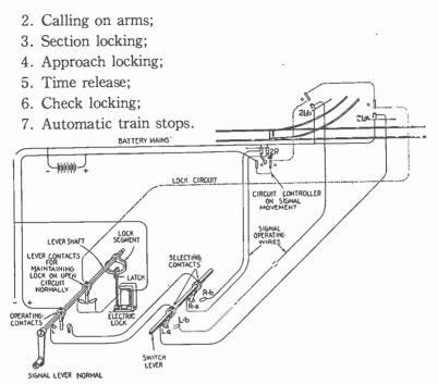
FIG. 6,675.—Diagram of complete signal control and indication circuits; lever and signals normal.
