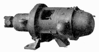
FIG. 6.479.—Westinghouse 32 volt, 500 watt locomotive head light unit. It consists of a single impulse steam turbine and an enclosed d.c. dynamo built together as a single unit. There are two self aligning ball bearings carried by the dynamo end brackets. The turbine rotor is mounted on the end of the dynamo shaft which is tapered and held in place by a lock nut and washer.
