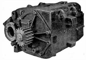
FIG. 6,136 .- General Electric truck mounted driving motor. suspension side.
