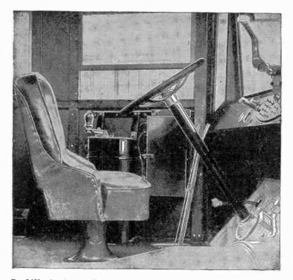
FIG. 6,128.—Interior view of General Electric gas electric drive bus showing dash and control. In addition to the regular pedal operated service brake and a hand lever emergency brake, this drive has an electric brake operated by a controller handle. On long, steep grades this method saves wear on brake bands and provides a positive uniform retarding force against which the bus cannot get out of control. It is also available as an emergency brake under any operating condition.
