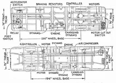
FIG. 6,126.—Equipment layout of 40 passenger single power plant gas electric coach. FIG. 6,127.—Equipment layout of 40 passenger dual power plant, gas electric coach.
