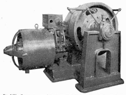
FIG. 6.791.—Gurney worm geared elevator machine with Gurney *d.c.* adjustable speed wide range field control motor. This type of motor is used for elevator speeds of from 200 to 450 r.p.m. with rheostatic control, where the source of current supply is *d.c.*
