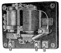
FIG. 6,462.—Safety C. H. & L. discriminating cut out or automatic switch. It is of the closed magnetic circuit type with pivoted armature. It has three voltage coils and one series coil, so arranged that when the dynamo voltage equals that of the battery the armature is lifted and the circuit closed.
