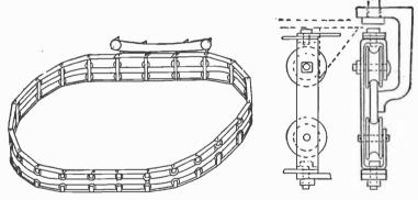
FIGS. 6,946 to 6,948 .- Delta continuous trolley system.
