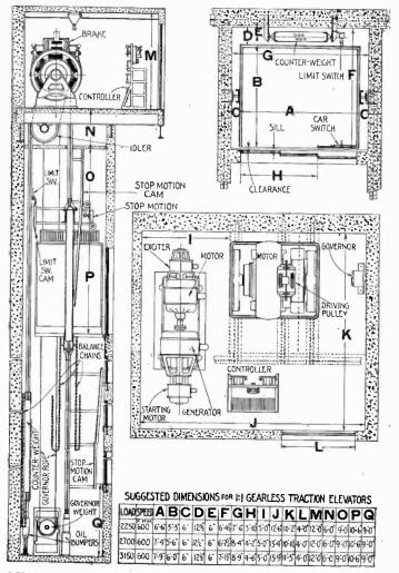
FIGS. 6,732 to 6,734.—A. B. See layout and recommended dimensions for 1:1 gearless traction elevators.
