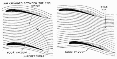
FIGS. 7,135 and 7,136.—Wings with, and without *stagger* showing effect of stagger in increasing the vacuum on the top surface of lower wing.
