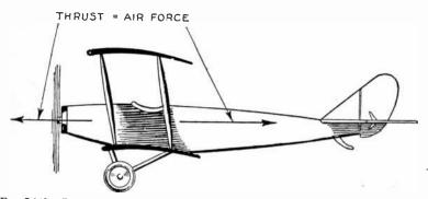
FIG. 7,142.—Relation between the thrust of the propeller and air force or resistance to the forward motion of the machine due to the air.
