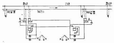
FIG. 6,657 .--- Check locking circuit.
