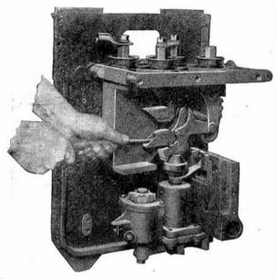
FIG. 6,278 .- Westinghouse contro. operation 5. Removing contact tips.
