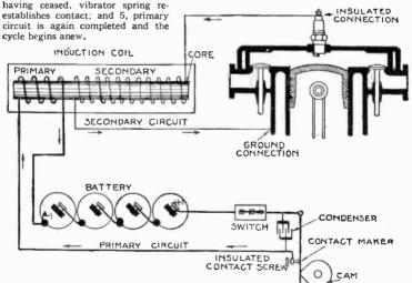
FIG. 7,001.—Diagram illustrating the principles of high tension or jump spark ignition. The nose of the cam in revolving engages the contact maker which completes the primary
