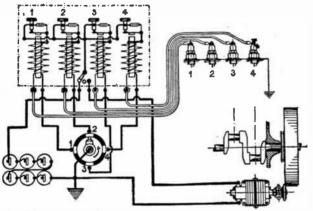
FIG. 7,002.—Wiring diagram of a dual jump spark ignition system for a four cylinder four cycle engine. A dry battery and low tension magneto form the two sources of current supply. The primary, or low tension circuit is shown by heavy lines, the secondary or high tension circuit by fine lines and the leads to spark plugs by the double lines. The dotted rectangle represents the outline of a four unit dash coil.
