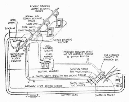
FIG. 6,670.—Diagram of complete *switch control*, indication and locking circuits; *lever partly reversed*, *switch in transit*. The lever is moved as far as the indicating segments and latches permit, the switch valve as having responded and the switch as responding, at midstroke. It shows the effect, the shurting of indicating wires, produced in the indicating system by the mechanical unlocking of the switch prior to and during its change of position.
