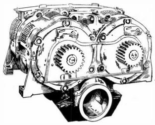
FIG. 6,150.—Westinghouse twin motor used on freight locomotives and high speed passenger locomotives. Note that two motors drive one pair of wheels. The same type motor in a suitable frame is used in multiple unit cars.
