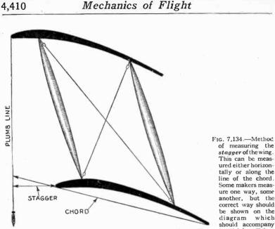
every wing. The two measurements may be as much as  $\frac{1}{2}$  inch difference, which is sufficient to make the machine nose, or tail heavy as the case may be.
