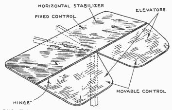
FIG. 7.112.—Horizontal stabilizer or fixed horizontal control surface to prevent sensitive response to the elevators. If the stabilizer be too large the machine becomes stiff and unduly resists the elevator control; if too small, it becomes tricky. In practice, it has been found that a stabilizer having an area of 6 to 8% of the wing area and placed from 2 to  $2\frac{1}{2}$  chord lengths back of the wing gives the best results.
