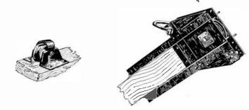
FIGS. 6,941 and 6,942.—Derrick fittings: 4. boom idler for guy derricks and boom end for operating clam shell or orange peel buckets. The hole on lower side is for a shackle pip which can be used to attach upper block for a fall with several parts.
