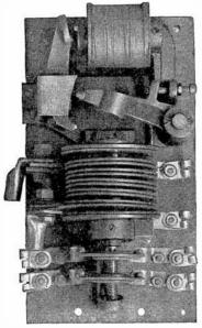
FIG. 6,182.—Westinghouse overload relay for locomotive.
