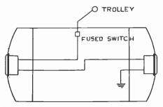
FIG. 6,484.—Head light wiring diagram for mine locomotives. 3. double end equipment, head light lamp voltage one-half that of circuit voltage; both lamps burn at same time.
