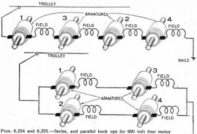
FIGS. 6,224 and 6,225.—Series, and parallel hook ups for 600 volt four motor equipment.
