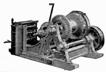
FIG. 6,851.—Mead-Morrison single drum *electric hoist*. This type is particularly adapted for hauling cars or hoisting elevators. It is found also on docks for hoisting and hauling of general cargo into warehouses, and in general huilding construction. It is equipped with slip ring motor and drum controller, but for many requirements the less expensive half high torque motor which has no
