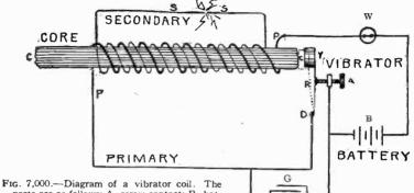
parts are as follows: A, screw contact; B, battery; C, core; D, vibrator terminal; G. condenser; P, primary winding; S, secondary winding; W. switch; Y, vibrator. When the switch
