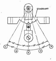
The final movement of the lever transfers the magnet which permitted such movement to the duty of locking the lever in its new position automatically when the track is occupied. Simultaneously with this action the other magnet is withdrawn from its section locking service and transferred to the indicating function required for the next operation of the switch.
