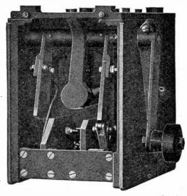
FIG. 6,798.—Westinghouse variable voltage control system 3. Landing switch. It has three contacts enclosed in an iron box. These contacts are closed by an operating arm with rubber tired roller that engages cams in the hatchway. A magnet with an exciting coil holds the operating arm away from the hatchway cams at all normal operating speeds of the car.
