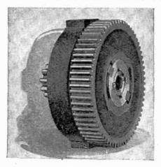
FIG. 6.886.—Euclid crane construction 13. Multiple disc automatic load brake. The center plate is stationary. The brake is fully released during the hoisting movement and automatically sets when the hoist motor comes to a stop. The load can be lowered only by reversing the motor.
