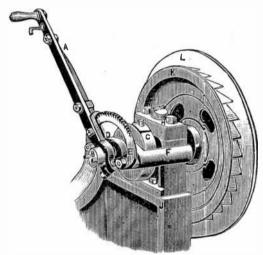
FIG. 6,868.—Lidgerwood friction lever on hoisting drum; a latch and quadrant hold the drum nny position.
