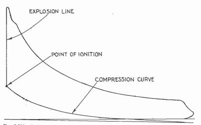
FIG. 6,996.—Indicator card for gas engine illustrating the *point of ignition*." It will be noted that compression continued to the end of the stroke, before the compression curve made an abrupt change into a nearly vertical line, the point of ignition, that is, the piston position at the instant of ignition, the nearly vertical "explosion" line with the high peak coming almost to a point, denotes a strong mixture and a quick explosion.
