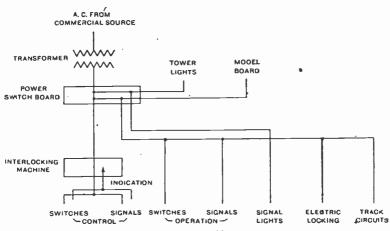
FIG. 6,644.-Diagram of power supply; a.c. interlocking.
