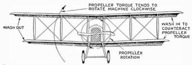
FIG. 7,131.—Front view of aeroplane illustrating how wash in opposes the turning over effect due to the propeller torque.
