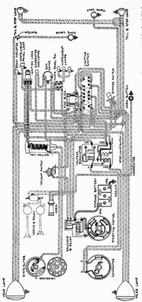
PLATE.-Wiring Diagram of electrical system as applied to Pontiac 8 cyl. 1936 (Delco-Remy). Generator: Current regulated by fixed third brušh. External voltage control, Rotation clockwise, viewing drive end, Starting Motor: Rotation clockwise, viewing pinion. Distributor: Rotation clockwise, viewing drive end.
