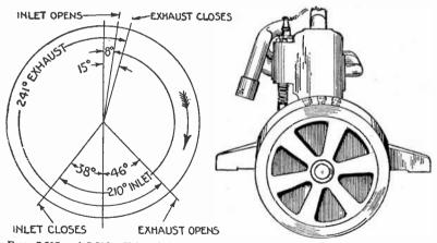
FIGS. 7,015 and 7,016.—Valve timing diagram and fly wheel markings. The timing of values is an operation which should be undertaken with caution and carried out with accuracy, and by a person competent to do such work. The usual markings on the rim of the fly wheel are as follows:
