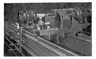
FIG. 6,888 — Euclid crane construction 15. Trolley drive mechanism used on small capacity cranes. The gear train for the trolley drive is housed in one oil tight compartment, revolving in an oil bath. The illustration also shows the method of mounting the controllers and rheostats on the trolley when the service conditions make such an arrangement desirable.
