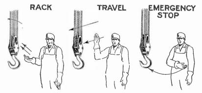
FIGS. 6,923 to 6.928 .-- Crane signals for operator's hoisting movements.
