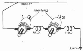
FIG. 6,218.-1,200 volt two motor equipment.
