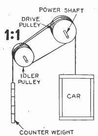
FIG. 6,752.—Direct (1:1) traction drive or method of transmitting power from the power unit to the car by means of frictional contact of the rope in passing one or more times around the drive pulley. This arrangement, since it does not employ a drum where size has to be considered, can be used for lifts of any height, and is the prevailing type today.
