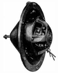
FIG. 6,134.—General Electric radiator fan motor equipped for vertical or horizontal mounting. Many car builders require a forced ventilated engine radiator to maintain proper cooling water temperatures. The motor is controlled by the motor car engine man, and turned on and off in accordance with the water temperature gauge on the engine.
