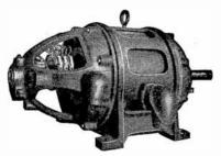
FIG. 6,788.—Westinghouse single speed, slip ring elevator motor. Designed for freight and passenger service where the elevator speeds are not too high to permit making satisfactory stops with a mechanical brake. Largely used for operating heavy elevators requiring motors larger than 25 horse power.
