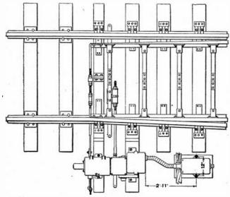
FIG. 6,630 .- Single switch layout.
