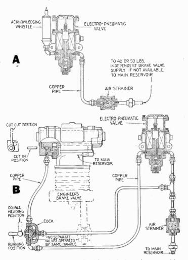
FIGS. 6,707 to 6,711.—General Railway Signal Co. air pipe layout for actuator giving unlimited brake pipe reduction. A, air pipe layout for acknowledging whistle; B, air pipe layout for actuator.
