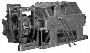
FIG. 6,900.—General Electric crane d.c. motors 2. For boom hoist. Series wound, totally enclosed, crane type motors with shoe type, series wound, spring set solenoid brakes and dynamic braking drum controller with low speed, heavy duty resistors are used.
