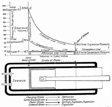
FIGS. 6.968 and 6.969.—*Theoretical indicator diagram* of a four cycle gas engine. The assumed values for temperature, volume, and pressure are a fair average of those occurring in the cylinder under actual working conditions.
