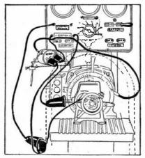
FIG. 7,078.-Testing a breaker.
