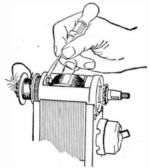
FIG. 7,062.—To test magneto armatures. A growler gives a very good magneto armature test. Place magneto armature in growler and with piece of wire arrange spark gap. If armature have make and break attached, operate this with finger and it should produce spark at the gap. If breaker be not attached, short the primary on and off with screw driver, as shown.
