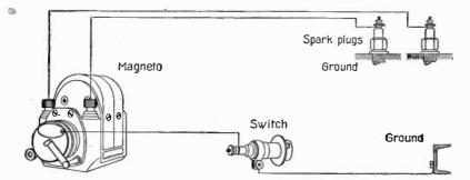
FIG. 7,054 —Bosch high tension magneto for *two* cylinder engine. Where the engine cranks are 180° apart, there is sometimes used what is called a half type magneto. This is a four cylinder magneto which has a distributer. Two of the distributer terminals are connected with the spark plugs. The other two, however, are either grounded or the current passing through them is allowed to jump the gap to ground.
