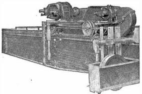
FIG. 6,884 —Euclid crane construction 11. Moderate duly trolley. All the hoist mechanism is located in a one piece housing. This housing rests upon two heavy saddle type steel castings. This entire trolley is machined to jigs and all parts are interchangeable. It is used regularly up to 5 tons capacity and intermittently up to 15 tons.
