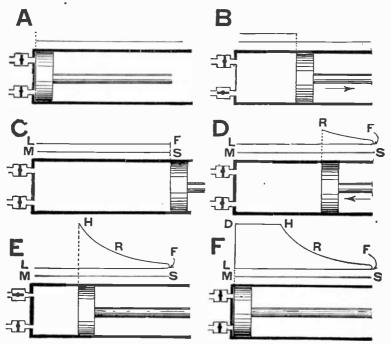
Figs. 8,932 to 8,937.—Compression cycle illustrated by indicator diagrams and elementary compressor. A, beginning of intake stroke; B, intermediate position of intake stroke; C, end of intake stroke, note atmospheric intake line LF, and vacuum line MS; D, intermediate position R, of compression stroke; E, point of maximum compression, note compression curve FRH; F, end of cycle, note horizontal discharge line HD, indicating discharge into receiver at constant pressure.
