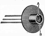
Fig. 8,993.—Cathode of Coolidge universal and therapy type tubes. It consists of a flat or slightly cone shaped spiral of tungsten wire A, mounted inside but close to the end of a metal tube B, to which it is electrically connected. The tungsten spiral or filament is heated from an external electrical circuit and becomes the source of cathode rays or electrons. The focusing depends largely on the shape of the spiral and its position in the metal tube.
