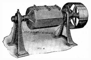
Fig. 8,278.—Hanson-Munning horizontal lumbling barrel. This type of barrel is to be preferred for large or long articles. The roll is nearer even and results nearer uniform. The horizontal barrel also has a larger capacity. The principal use of the horizontal type of barrel is for what the trade terms "rough work," such as grinding or smoothing up.
