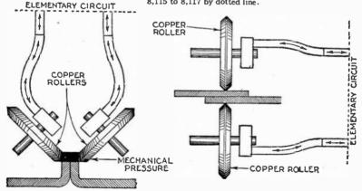
Figs. 8,115 and 8,116.—Circuit diagrams for seam welding. It consists of passing two or more metal sheets or bars, between the rollers of a seam welder. The electric current passing from roller to roller through the work heats up the parts to be joined in the nature of a spot welder and the mechanical pressure on the roller electrodes consummates the weld.
