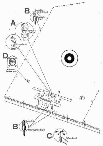
Fig. 8, 406 to 8, 412.—Minimum lighting facilities required for an air port to obtain an "A" rating A, air port beacon. Minimum candle power not less than 100,000 for long range, and in no case less than 15,000 candle power. Rotating or flashing with flashes not less than one-tenth
