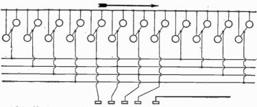
Fig. 8,595.—Number sockets 1-2-3-4. Connect all No. 1 to circuit No. 1 and to flasher brush No. 1. Nos. 2, 3, and 4 likewise. Keep in mind, that the direction of the numbering determines the direction of movement of the shadows.
