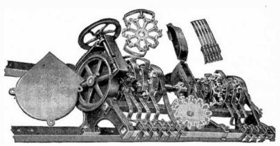
Fig. 8,583.—Betts & Betts combination flasher showing general construction.
