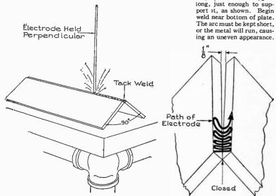
Figs. 8,083 and 8,084.—Lesson 6. Straight butt weld method of making right angle butt weld in horizontal position. Good appearing weld, even across the top without bumps, craters, or
