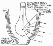
Fig. 8,381.—Holophane diffusing globe. Sectional view showing features.
