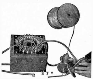
Fig. 8,216.—Chapman universal armeter used with carbon contact resistance soldering leads. Connect pair of No. 8 flexible leads to say O and 5V terminals.
