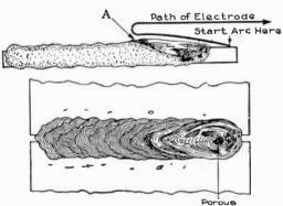
Figs. 8,098 and 8,099.—Section of deposited metal showing penetration and crater.
