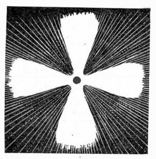
Ftg. 8.420.—Plan view of direction in which illumination is desired at street intersections and along streets and how prismatic globes direct the rays.
