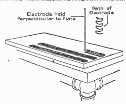
Figs. 8,072 and 8,073.—Lesson 2. Three parallel beads. In this and all following lessons, the deposited metal should meet all the requirements of a good weld, uniformity of height and width, regularity of ripples, good penetra ion, and no overlap nor signs of porosity. These
