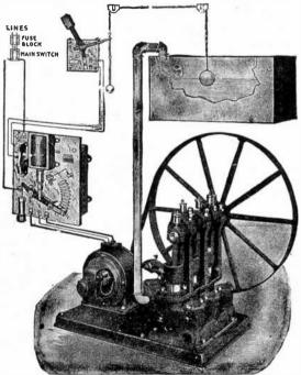
Fig. 8,852.—Automatic control for electric house pump, consisting of float switch, starter, and connection, as shown.
