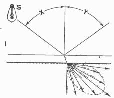
Fig. 8,380.—Effect of various media on light rays.  $F_{\mathcal{F}}$  reflection and transmission by etched glass.
