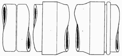
FNS. 8,166 to 8,168.—Various pipe joints for welding. Fig. 8,166, butt weld; fig. 8,167, bell and spigot weld; fig. 8,168, bell and spigot weld with welding dam.
