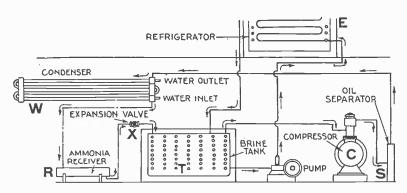
Fro. 8,661.—Ammonia compression system: 2, brine circulating method. In operation, ammonia is expanded through piping submerged in a brine tank, or through a special cooler or evaporator. The brine, after being reduced to a low temperature, is pumped through piping placed in the compartments to be chilled. C, compressor; E, refrigerator; R, receiver; S, oil separator; T, brine tank: W. condenser; X, expansion valve.
