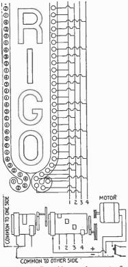
is obtained automatically by the alternate heating and cooling of the metal of the flasher, which causes it to expand and contract.
