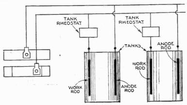
Fig. 8.263.—Two wire line connections.
