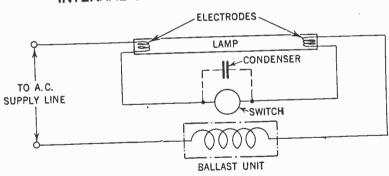
Figs. 9 and 10.—Glow switch starter and connection to lamp unit.
