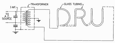
Fig. 6.—Typical wiring diagram showing radio interference suppressor in transformer primary.
