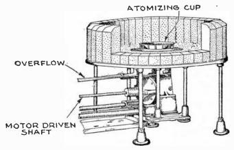
Fig. 8,706.—Motor driven centrifugal atomizing burner.
