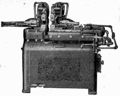
Fig. 8,118.—Thompson butt welder. Capacity.—Iron or steel. A cross section from .012? minimum to a cross section of ¾ sq. in. maximum continuously, or 1 sq. in. at long intervals. Rims 2½ ins. wide by ¼ in. thick by 10½ ins. minimum diameter. Rims 1¾ ins. wide or narrower and as small as 8 ins. diameter can be handled. Pipe or tubing up to 1 in. diameter extra strong; pipe or tubing 1¾ ins. diameter standard, can be welded by fitting contacts to size.
