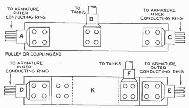
Figs. 8,255 and 8,256.—Connecticut terminals connected for two wire system. The bar K connects the two short blocks. Also note that on the pulley end the cables from the upper block lead to the outer conducting ring, while on the end opposite the pulley it is the lower block that is connected to the outer conducting ring. The two lugs B and F, should be connected to the main conductors leading direct to the work.
