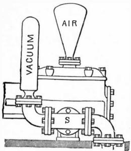
To avoid the air chamber and its defect just mentioned the author substituted a spring cushion on the high speed direct connected boiler feed pump of his marine engine, as shown in fig. 8,819, and further described in Chapter 52, Audels Engineers and Mechanics Guide No 4
