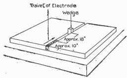
Fig. 8,055.—Method of reducing contraction by locking up the stresses produced. When welding long searns, the drawing may be reduced to almost nothing by the use of spacing blocks or wedges placed in the opening approximately 18 ins. from the section being welded, and toward the end of the seam to which the weld is progressing.
