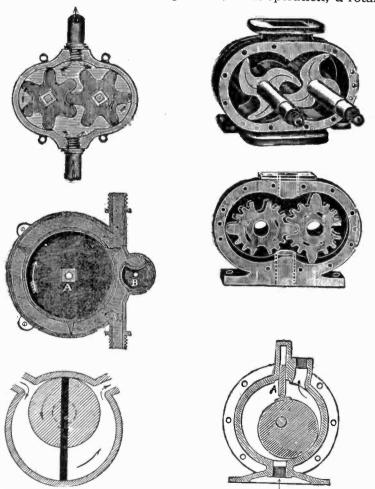
Figs. 8,900 to 8,905.—Various types of rotary pump.
