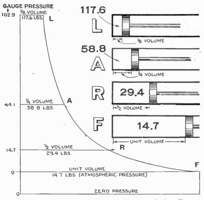
Figs 8,927 to 8,931.—Diagram and compression stroke progressively shown illustrating Boyle's law. As the piston travels from position F, to R,A,L, the pressures are 14.7, 29.4,58.8, 117.6 this absolute, respectively, being inversely proportional to the volume. The points F, R, A, L, on the compression curve correspond to the piston positions F, R, A, L as shown.
