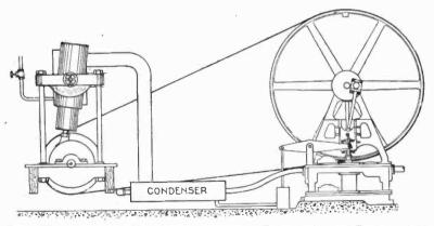
Fig. 8,920.—Graham jacketted, transfer expansion oscillating engine, and Dunham power pump with belt transmission. It must be evident that this arrangement permits the engine and pump to work under the most favorable conditions for economy. Hence by proper proportion of pulleys, the engine may run at high speed, thus reducing the size of the cylinder and loos by condensation, leakage, etc., and the pump may be run at slow speed, thus eliminating water hammer, slamming of valves, etc.
