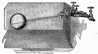
Fig. 8,745.—Butfalo automatic make up and quick filler. The required water level in the tank is automatically maintained by the float valve here shown. This allows constant operation of the pump at uniform suction head. It is also essential that provision be made for rapid filling of the tank after cleaning, and this is provided for ty the extra flanged pipe inlet, which also serves as a hose connection.
