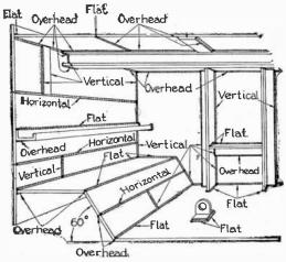
fig. 7,981.—Various positions of weld.
