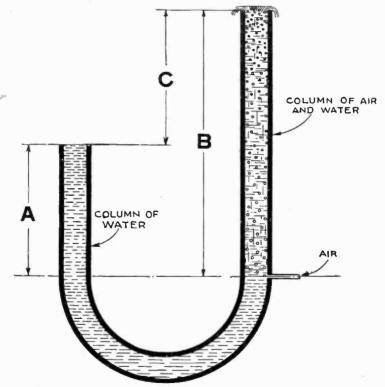
Fig. 8,925.—Principle of air lift. The injection of air at the point indicated produces a column of mixed air and water B, which has less weight than the solid column of water A. Thus the weight of the column A, causes the water to rise the distance C, and overflow.
