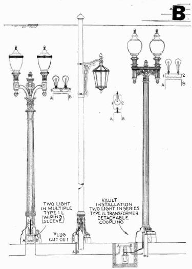
Fig. 8,346 to 8.349.—General Electric Novalux series street lighting system. Section B.
