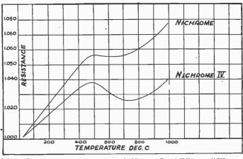
Fig. 8,217.—Temperature coefficient curves of "Nichrome" and "Nichrome" IV here shown represent wire slowly cooled from 1000° C. as specified by the American Society for Testins Materials. Slight variations from this curve may be expected due to variations in methods of annealing of different sizes of wire.
