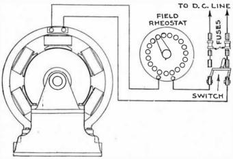
Fig. 8,262.—Connecticut separately excited dynamo. In this machine the field is excited from a separate source of d.c. of the same voltage as that stamped on the name plate following the word excitation. A separately excited machine is always supplied with a field rheostat and the connections should be made as here shown. By the use of the field rheostat the voltage can be lowered to a small value with stability.
