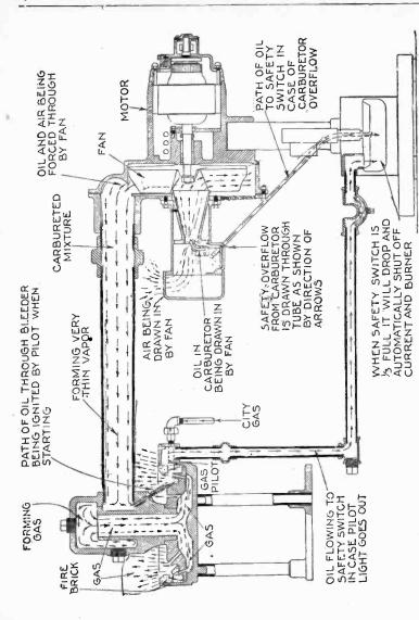
Fig. 8,702.—Crystal mixing vaporizing burner. Sectional view showing operation.
