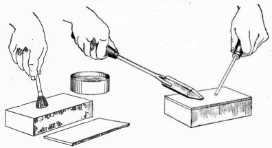
Figs. 8,209 to 8,212.—Sweating. When two surfaces are to be united by sweating, first see that the surfaces are perfectly clean, then flux as in fig. 8,209. Put a piece of tinfoil over one surface and the other surface on top. They should be held firmly together by a clamp or other means and heated as in fig. 8,212 by a hot bit, or if the metal have considerable thickness by a torch, until the solder melts. When cool, the surfaces will be found to be firmly united.
