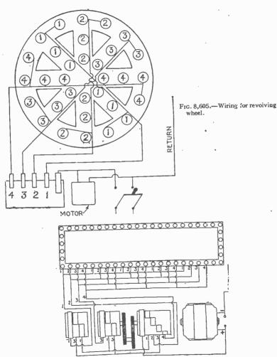
Fig. 8,606.—Standard reversing traveling or running border. It travels first to the right, then to the left, reversing approximately every three seconds. Requires four brush speed flasher with four controls.
