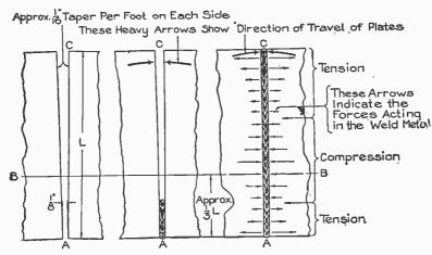
Figs. 8,051 to 8,053.—Locked-in stresses in a weld due to contraction. When the joint is completed, the transverse contraction stresses along the joints will be greatly concentrated at the ends A and C. The stresses impair the quality of the weld and, in many cases, develop a fracture on cooling. When a fracture develops where this method is used, it usually occurs at the end where the joint is finished.
