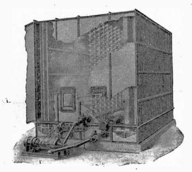
Fig. 8,734.—Carrier humidifier equipped with rotary strainer. In operation, air enters at right, through the baffle plates, passes through the spray chamber and leaves at the left through the washer eliminator plates. The parts are, R, rotary strainer; E, ejector heater P, pump; M, pump motor, S, pot strainer
