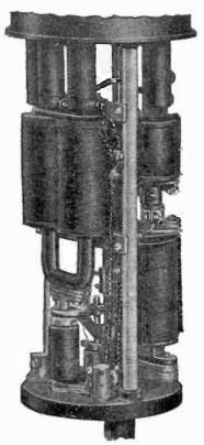
Figs. 8,326 and 8,327.—Views of mechanism of General Electric luminous arc lamp. The arc is struck between a stationary copper upper electrode and a movable magnetite lower electrode and burns under normal updraft conditions. In construction: The lower electrode is carried on a rod actuated by the standard type of shoe clutch mechanism. The current is carried to the electrode by means of a flexible spiral connection contained in a tube which is
