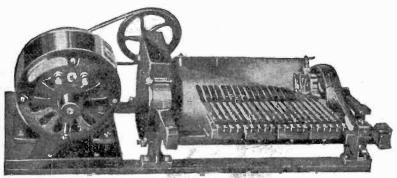
Fig. 8.575.—Betts & Betts script flasher. This machine is used to produce a smooth, advancing flow of light such as is required in writing letters or words one lamp at a time, for rockets, shooting stars, etc.
