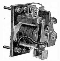
Fig. 8,567.—General Electric jack mounted fire relay. This fire type or remote off relay is exactly the same as the standard relay except for a third set of silver contacts which close when the relay is de-energized. The flasher relay is identical in all features with the standard relay except that different connections are made to the jacks.
