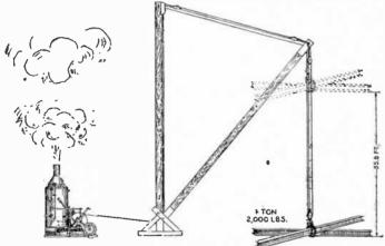
Fig. 8,631.—The fusion of ice, illustrating the work done when the pound of ice at 32° Fahr, is melted or converted into water at the same temperature. The latent heat of fusion being 143.57 heat units, and since one heat unit is equivalent to 778 ft. lbs. the work done during the fusion of one pound of ice is 778×143.57 = 111,698 ft. lbs. This is approximately equivalent to the work done when a hoisting engine hoists 2,000 lbs. a distance of 55.8 ft. as shown in the illustration.
