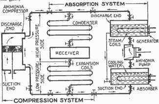
FIGS. 8,665.—Elementary combined compression and absorption machines showing that each system has in common a condenser, receiver and expansion coils.
