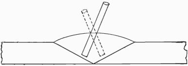
Fig. 8,056.—Best theoretical welding angle.
