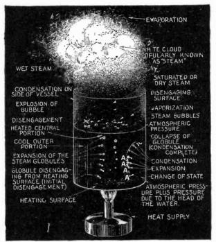
Fig. 8,635.—Vaporization or the process of boiling as illustrated by the boiling of water.
