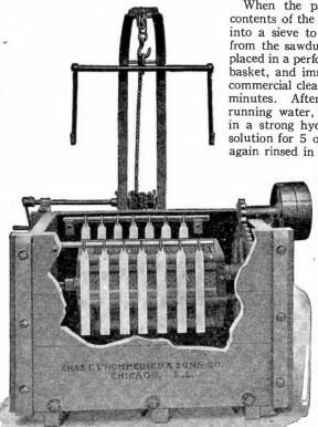
When the parts are clean the contents of the barrel are dumped into a sieve to separate the parts from the sawdust. Then they are placed in a perforated metal or wire basket, and immersed in a boiling commercial cleaning solution for 15 minutes. After rinsing with cold running water, they are immersed in a strong hydrochloric acid dip solution for 5 or 10 minutes and again rinsed in cold running water
