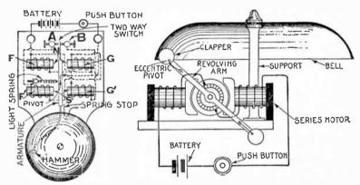
Fig. 8,457.—Elementary double acting bell. In operation, magnets F,G', and F',G, are alternately energized. Assuming the current to flow first through F,G' and then through G F', F and G', will have N and S poles, and G and F',S and N poles; these will induce unlike poles in the ends of the armature attracting it at both ends.
