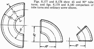
Figs. 8,182 to 8,184.—180°, 90° and 45° tube turn fittings. The dimension letters refer to the dimensions in the accompanying table.
