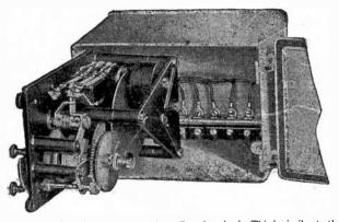
FIG. 8,559.—General Electric synchronous timer (interior view). This is similar to the standard induction timer except that a synchronous motor drive is used in place of the induction motor drive. The motor speed, is, of course, fixed for a given frequency and therefore the time of the complete cycle cannot be readjusted except by replacement of the driving gears.
