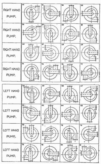
Figs. 8,860 to 8,891.—Various patterns of centrifugal pumps.
