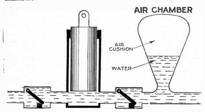
Fig. 8,818.—Elementary boiler feed pump with air chamber. In small sizes these are sometimes direct connected to the engine and often run at high speeds. Obviously some form of cushion against water hammer is necessary. Fig. 8,819 shows a better and more up to date method of cushioning water hammer.
