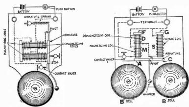
Fig. 8.450.—Elementary differentially wound vibrating bell. In operation, when the battery circuit is closed: 1, Current flows through the magnetizing winding and energizes magnet; 2, magnet attracts the armature; 3, contact maker closes circuit through demagnetizing coils; 4, demagnetizing coils demagnetize the magnet; 5, armature spring pulls armature back against the stop, while, 6, the contact maker breaks the circuit through demagnetizing coils.
