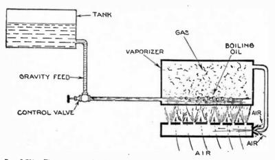
Fig. 8,701.—Elementary gravity feed induction mixing vaporizing burner. In operation, oil flows from tank to vaporizer, regulated by the control valve. The flame from the burner vaporizes the oil entering the vaporizer producing a gas which passes out to the mixer. The gas is injected through a nozzle into the mixer sucking in air, the mixture passing out and igniting at the top.
