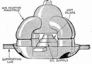
Fig. 8,699.—Casting which constitutes a simple gravity feed, vaporizing type burner
