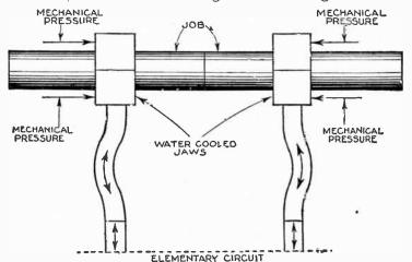
Fig. 8,117.—Circuit diagram for butt welding.
