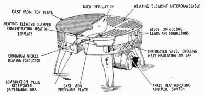
Fig. 8,219.—Electric disc stove. Adapted to laboratory and other industrial purposes. The maximum surface temperature is 750° Fahr.
