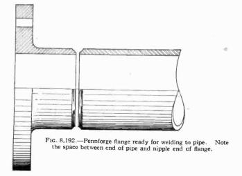
When welding flanges, the flange and pipe are clamped in a fixture, or to a companion flange, to line them up correctly.
