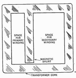
Fig 1.—Outline of neon sign transformer core.
