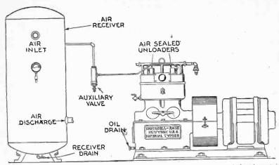
cig. 8,961.—Piping diagram for Ingerso'l-Rand stationary direct connected electric motor driven air compressor arranged for constant speed operation.
