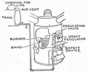
Fig. 8,710.--A simple manually controlled vaporizing burner installation in a warm air furnace.
