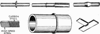
Fig. 8, 119 to 8,124.—Various examples of butt welds. Fig. 8,119, flash weld; fig. 8,120, tool weld; fig. 8,121, upset weld; fig. 8,122, high speed steel weld; fig. 8,123, pipe weld; fig. 8,124, tee weld.
