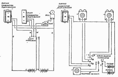
Fig. 8,479.—Partrick & Wilkins return call system using combination buzzers or buzzer pushes and buzzer or bulb separate.
