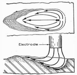
Fr3s. 8,091 and 8,092.-Diagrams showing flow of welding metal when welding.
