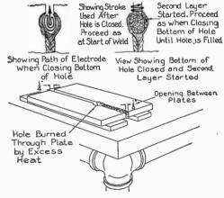
Figs. 8,088 to 8,090 .- Method of filling hole in butt weld caused by arc melting through.
