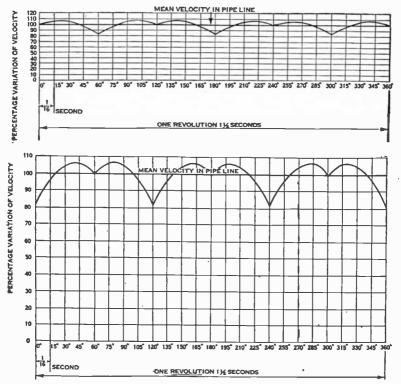
Fig. 8,840.—Diagram showing rate of delivery of single acting triplex pump expressed in percentage of mean velocity in pipe line.
