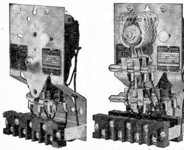
Fig. 8,568.—Leland speed border flasher; unit type for four circuits. The usual practice is to divide the display into four circuits of groups or circuits, and order the flasher for 1-2-3-4 wiring; or I to 4 wiring. The masher then turns on the four circuits in succession and repeats interminably, each circuit going dark before the one preceding it is lighted up, so that there is always one or two circuits dark out of each set of four.
