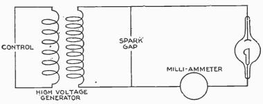
Fig. 8,984.—X-ray circuit diagram snowing primary and secondary winding ct induction coil, spark gap for measuring voltage and milli-ammeter.
