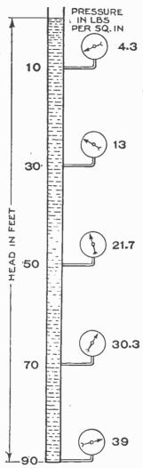
Fig. 8.803.—The pressure of water due to head increases with the depth.
