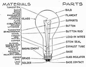
Fig. 8,294.-Materials and parts of an incandescent lamp.
