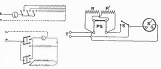
Fig. 8,234.—Arrangement of internal circuits for heaters in which each resistance section if controlled by a separate switch.
