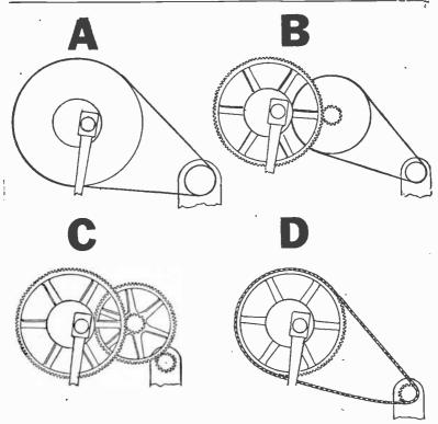
Figs. 8,842 to 8,845.—Various forms of drive for power pumps. A, belt, single reduction; B, combined belt and toothed gear, double reduction; C, tooth gear, double reduction; D, chain, single reduction.
