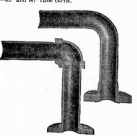
Figs. 8,179 and 8,180.—Comparison of tube turn and ordinary screw elbow. Note the easy curve of the tube turn as compared with the shoulders of pipe in the screwed assembly. Also contrast the modern, high hub butt welding flange with the old fashioned flange.
