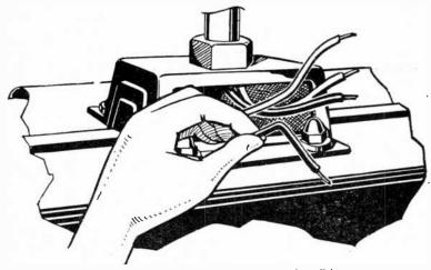
Fig. 15.—Splice box with cover removed, showing wires ready for splicing.
