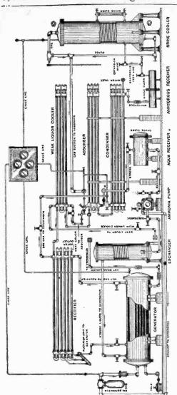
Fig. 8,669.—Carbondale double pipe type absorption refrigeration machine.
