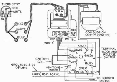
Tro. 8,728.—Minneapolis Honeywell connection diagram for motor switch; 110-220 volts, 6th cycle a.c.
