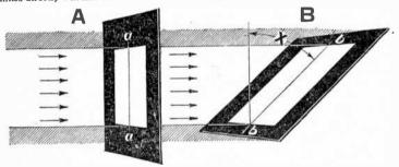
Fig. 8,363.—Illumination of perpendicular and inclined surfaces. If instead of being perpendicular to the beam of light as at A a plane is tilted at the angle X, as at B, the same amount of light is spread over a greater area: The illumination on B is to A inversely as the length bb is to as or as cosine X. Thus if  $\cos X = .7$ , and the foot candlage on A is 1, the illumination on B would be .7 foot candle.
