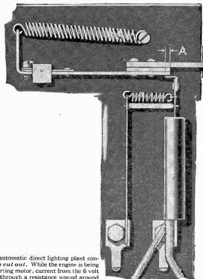
Fig. 8.787.—Delco automatic direct lighting plant control. 6. Cranking cut out. While the engine is being cranked by the starting motor, current from the 6 volt battery is passing through a resistance wound around one of the thermostat blades. As the resistance wire
