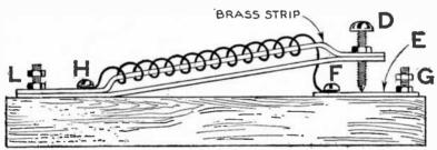
Fig. 8,586.—Elementary thermo flasher to illustrate principle of operation as explained in the text. D, adjustable contact; E, contact plate; H and F, winding terminals; G and L, external circuit connections,
