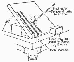
Fig. 8,082.—Lesson 5. Laying three parallel beads, 45°. Instructions: Similar to Lesson No. 1. The plate may be rested against a brace or welded to the bench top by a weld about ½ in.
