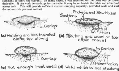
Figs. 8,066 to 8,069.—Cross section of beads deposited under different conditions.
