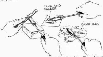
Figs. 8,204 to 8,206.—"Tinning" the bit. Fig. 3,204, cleaning bit by filing working surfaces with an old file; fig. 8,205, rubbing the bit on the flux and solder, which may be conveniently placed on a piece of sheet tin as shown; fig. 8,206, removing surplus solder by giving each ride of the bit a quick stroke over a damp rag.
