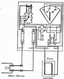
Fig. 8,237.—Control panel with switches, fuses and thermostat for the automatic regulation of heat.
