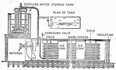
Fig. 8,671.—Detail of freezing tank of an Eclipse ice plant, showing the arrangement of the cans with covers, also the brine agitator. The agitator is in the shape of a propeller which keeps up a continuous circulation of brine between bottom and top of tank.
