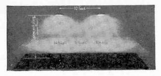
Fig. 8,386.—Illumination of vertical surfaces. Spacing between luminaires should not exceed 1½ times the mounting height above the work plane—uniform illumination (foot candle values based on 200 watt units).
