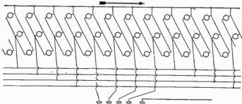
Fig. 8,599.—An arrangement for border and speed effects where a heavy border is necessary or where dark colors are used. Many variations and novel effects are possible by special arrangement of lamps and connections.
