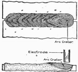
Figs. 7,974 and 7,975.—Longitudinal section of deposited metal showing penetration and are crater. Correct penetration will make certain that the metal of the plate is melted and in condition to receive the metal projected from the electrode, and also that the area of the crater will be sufficient to receive all of the metal from the electrode and not permit any of the deposited metal to overlap on the solid metal of the plate where it will not stick.
