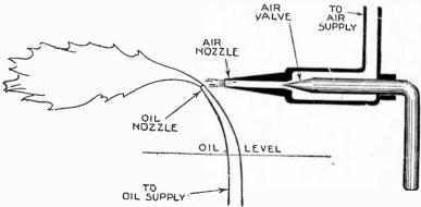
Fig. 8,708,—Atomizing oil by air iet or spray.
