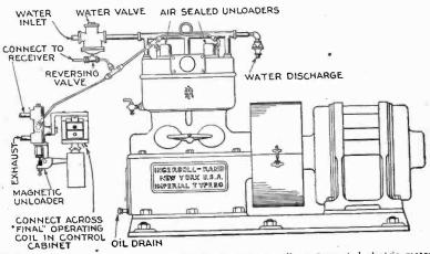
Fig. 8,962.—Piping diagram for Ingersoll-Rand stationary direct connected electric motor driven compressor arranged for automatic start and stop control.
