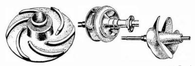
Figs. 8,897 to 8,899.—Three forms of vane. Fig. 8,897, straight type: fig. 8,898, Francis mixed flow: fig. 8,899, impeller or screw, axial flow.
