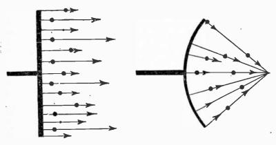
Figs. 8,981 and 8,982.—Flat and circular cathode or negative terminal showing direction of the cathode rays.
