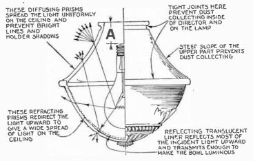
Fig. 8,419.—The refraction of light due to prisms in a globe. The prisms redirect the rays and pass them out in the planes desired; this is important in street illumination as it is desired to reflect all or nearly all to the street surface.
