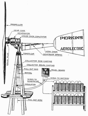
Fig. 8,791.—Aerolectric generating mechanism with gear case cover removed, showing transmission between wheel and dynamo. This is a wind mill suitably geared to a dynamo forming a unit for charging a storage battery, the latter being used as current source for house lighting.
