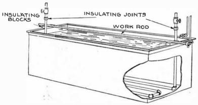
Fig. 8,276.—Cleaning tank. Typical installation of steam heating coils for heating plating solutions and cleaners. Approximate length of pipe needed for each 10 gals. of solution: 3½ stranded pipe, 4 lineal ft.; 1 in. stranded pipe, 3 lineal ft.; 1½ in. stranded pipe, 2½ lineal ft.; 1½ in. stranded pipe, 2 lineal ft.
