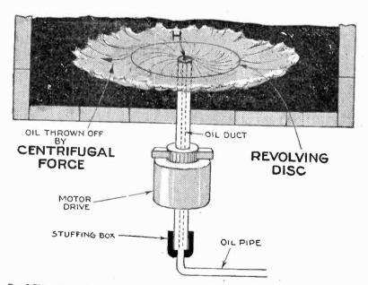
Fig. 8,700.—Elementary centrifugal force atomizing burner. The oil flows through the hollow spindle of a disc which is rotated at high speed by a motor. The oil overflowing at H, onto the disc at its center is hurled oif the disc by centrifugal force, and ignited by a torch or oilot light, produces a ring of flame.
