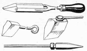
Figs. 8,194 to 8,197.—Various soldering bits, or so called "irons." Fig. 8,194, ordinary edge bit; figs. 8,195 and 8,196, hatchet bits; fig. 8,197, pointed bit.
