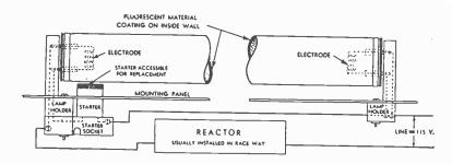
Fig. 6.—Assembly of typical fluorescent lamp showing auxiliaries and connections.
