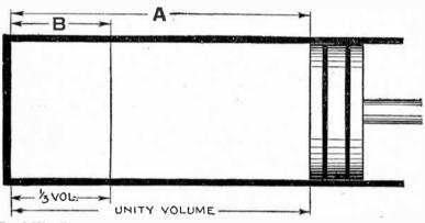
Fig. 8,938.—Elementary air compressor illustrating the phenomena of compression as stated in Boyle's and Charles' laws and explained in the accompanying text.
