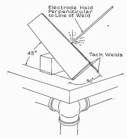
FIG. 8,085.—Lesson 7. Right angle butt weld inclined 45° to horizontal. This is the same as Lesson No. 6, except that, after tacking the plates as shown in fig. 8,083, they are placed so the weld makes an angle of 45° with the horizontal. The end having the ½ in. opening should be at the top. Begin at the lower end, and weld upward and away from the operator, as shown.
