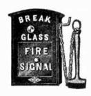
Figs. 8,517 to 8,519.—Partrick & Wilkins break glass fire alarm signal boxes or open circuit, with vibrating bells. Fig. 8,517, No. 1 signal, breaking of glass automatically closed circuit. For low voltage only; fig. 8,518, flush type for low voltage; fig. 8,519, type for 110 volts or less.
