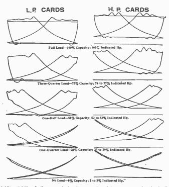
Figs. 8,971 to 8,980.—Indicator cards showing operation of clearance control at tive load points.
