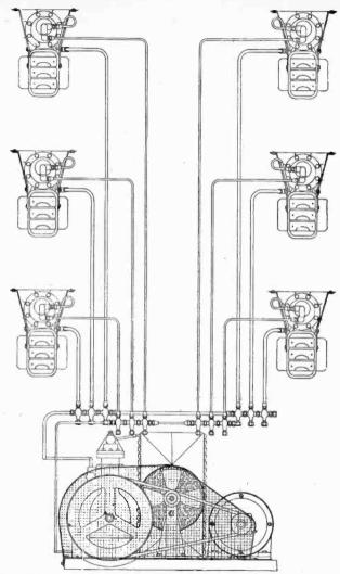
Fig. 8.693.—Servel apartment house installation using the manifold system.
