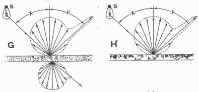
Figs. 8,378 and 8,379.—Effect of various media on light rays. G, reflection and transmission of opal glass; H, reflection from porcelain enameled steel.
