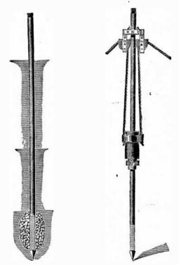
Fig. 8,909.—Driven well, showing pipes and perforated well point.
