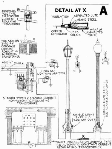
Fig. 8,339 to 8,345.—General Electric Novalux series street lighting system. Section A.
