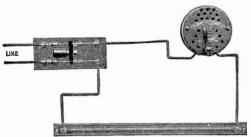
Fig. 8.229.—Cutler-Hammer space heater with rheostat heat control.
