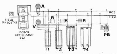
Fig. 8.280.—Diagram of two wire system showing method of connecting dynamo, tanks, plating barrel, volt meter, ammeter and rheostat. A, ammeter; V, volt meter; S, ammeter shunt; R, tank rheostat; T-1, two rod tank, one row work; T-2, three rod tank, one row work; T-3, five rod tank, two row work; T-4, electric cleaner, steel tank; PB, reliance plating barrel; N, insulator; 1, No. 1 brass connections; 2, No. 2 brass connections; 7, No. 7 brass connections.
