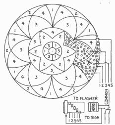
Fig. 8,608.—Chromatic or kaleidoscopic effects. These are usually wired in five circuite as shown.
