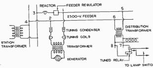
Fig. 8,426.—Diagram of substation bus with single feeder. The control currents are produced by the alternator G. This is a rotating machine of a standard type driven by a two speed induction motor or by a single speed induction motor with a two speed gear shift. The two speed motor runs at 1,200 and 1,800 r.p.m., while the single speed motor runs at 3,600 r.p.m.
