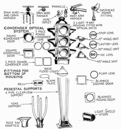
Figs. 8,525 to 8,553.—Parts of General Electric pendant and pedestal signals.
