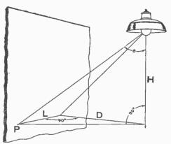
Fig. 8.388.—Illumination of vertical surfaces. In calculating the illumination at the point P on a vertical surface the distance H (vertical), D (horizontal), and L (horizontal to the surface)
