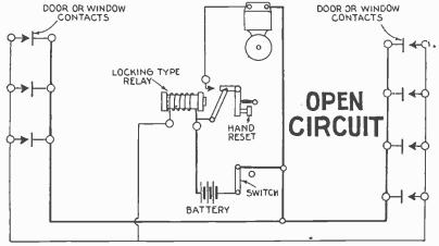
Fig. 8,498.—Open circuit burglar alarm system to be operated in parallel. In hook up there must be: 1, one common wire to one side of all window or door springs, switch and better
