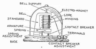
Fig. 8,449.—Sectional view of a buzzer. In construction, the armature is pivoted to the lower part of an upright soft iron shield or standard from the top of which the magnet is firmly suspended. The armature being pivoted to the shield, vibrates between the magnet and wooden base and is regulated by adjusting screws underneath. The mechanism is enclosed in a bell or brass shell.
