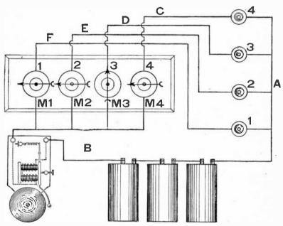
Fig. 8,489.—Method of wiring an annunciator; diagram shows the various circuits, bell, battery, push button, drops, etc.
