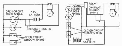
Figs. 8,500 and 8,501.—Open and closed circuit diagrams of Edwards' burglar alarm systems. These show the window and door contact springs of the open and closed types, the constant ringing drop to make the bell ring continuously when once started, and the actuating relay to close the bell circuit on the closed circuit system.
