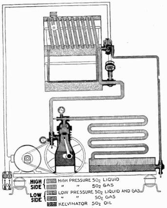
Fig. 8,681.—Kelvinator dry system cycle
