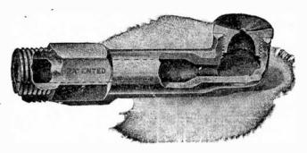
Fig. 8,733.—Carrier spray nozzle. The water entering through the small circular chanter tangentially, acquires a whirling motion and is discharged through a small orifice in the center of the cap. The approach to the orifice is conical in shape, so that the rotation, or whirling speed of the water is greatly increased at the instant of discharge
