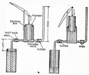
Figs. 8,813 and 8,814.—Elementary single acting plunger pump showing essential parts. The distinction between a plunger and a piston should be carefully noted. In operation during the up stroke water fills the cylinder, inlet valve opens, and outlet valve closes, as shown in fig. 8,813. During the down stroke, the plunger "displaces" the water in the barrel, forcing it through the discharge valve against the pressure due to the head.
