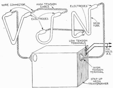
Fig. 8,338.—Neon tubes showing wiring connections.
