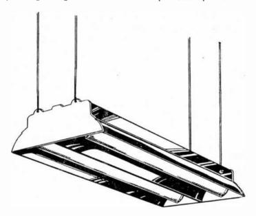
Fig. 16.—Typical two-unit fluorescent lamps assembled with reflector.
