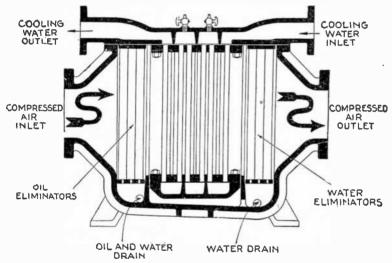
Fig. 8,953-Sullivan air or gas after cooler.
