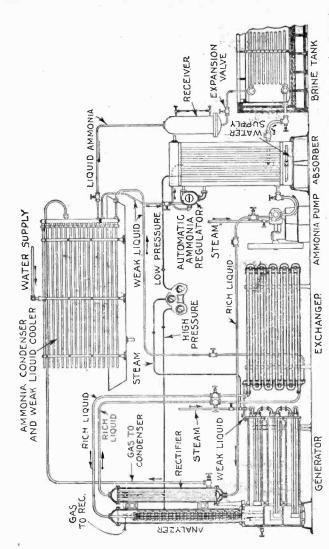
Fig. 8,666,—Large absorption plant. In this system the rich líquor is circulated through the rectifier before passing through the exchanger, thus some of the heat which would otherwise be carried off in the condensing water is saved.
