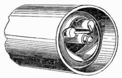
Ftg. 0.704.—Oil-Electric draft tube, air diffuser and spray nozzle showing location of spark in  $\nu$  ation to spray nozzle.
