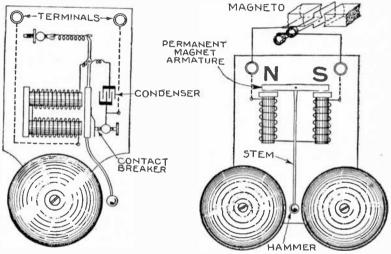
Fig. 8,452.—Elementary heavy duty high voltage bell. The winding is of fine wire to secure enough resistance to keep down the current to proper value. Sparking is avoided by connecting a condenser across the contact breaker as shown.
