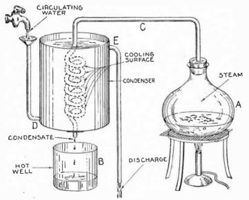
Fig. 8,646.—Experiment illustrating condensation. If water for instance be hoiled in a flask. A, and the steam thus produced led off through pipe C, having a coiled section surrounded by cold water, it will here be cooled below the boiling point and will therefore condense, the condensate passing out into the receptacle B, as water. The cooling or "circulating" water enters the condenser at the lowest point D, and leaving at the highest point E.
