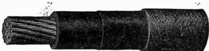
FIG. 5,075.—Automobile starting and charging cable. Used for connecting the batteries to the starting motor and dynamo, of a gasoline propelled car. One conductor, sizes 2 to 00 A.w.g. stranded. Insulation, "Black Core" rubber compound. Intermediate covering, one overlapping strip of varnished cambric. Overall covering, one (2 coat) varnished braid, 1-64th in. thick.
