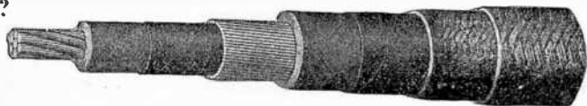
FIG. 5,095.—Concentric mine cable. This is used for the reels of gathering reel locomotives and for cutting machines. It has the advantage of being round and of small diameter. Two conductors. Stranding of center conductor, flexible. Stranding of outer conductor, ring of wires having total cross sectional area equal to that of center conductor. Covering of center conductor, rubber filled tape. Covering over outside conductor, belt of "Black Core" rubber compound. Covering over belt, rubber filled tape. Covering over tape, two extra tight water proof braids.
