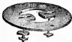
FIGS. 5,603 and 5,604.—Austin "Economy" old work hanger. Application: The plaster is opened only large enough to permit the stud to pass through. The stud is then slipped up the end of the bar as shown and the assembly slipped through the hole. When the box is in a horizontal position, the wire leader is drawn through the stud. This slides the bar into position and centers the stud on the bar. The outlet box is fastened to the stud with a locknut and secured tightly in place.
