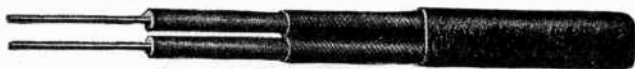
FIG. 5,083.—Solid twin (flat) code house wire. Used for the same purpose as stranded twin code house wire. Two conductors, sizes 6 to 14 A.w.g. Insulation on each conductor, "Black Core" rubber compound. Covering over insulation, one saturated braid. Grouping of conductors, parallel. Covering overall, one saturated braid.
