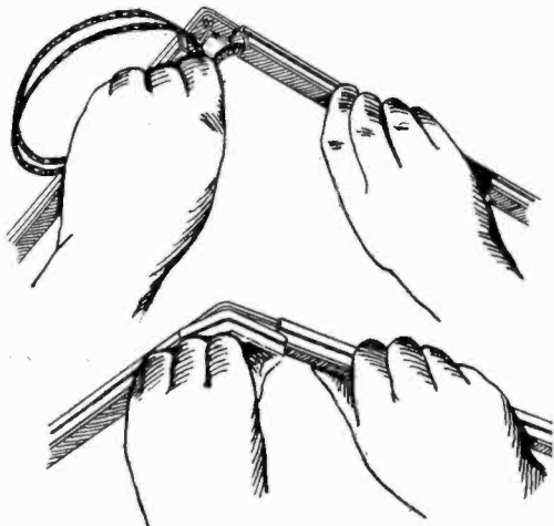
FIGS. 5,357 to 5,359.—Method of making a 90° turn with a Wiremold flat 90° elbow. First assemble coupling tongues in base plate as in fig. 5,357, being careful that the coupling tongue goes outside the moulding base. After fastening the base plate to the wall with wood screw or toggle bolt, push in or fish in the wires as in fig. 5,358. Finally, snap on the elbow cover, breaking off the crescent shaped twistouts in the ends for use with the four wire moulding. Do not put covers on any of these fittings until wiring is completed.
