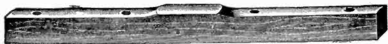
FIG. 5,809.—Cross arm which carries the insulator pins. The standard cross arm is 3\frac{1}{4} \times 4\frac{1}{4} ins., double painted, and bored for 1\frac{1}{2} in. pins and two \frac{1}{2} in. bolt holes. Telephone arms are 2\frac{3}{4} \times 3\frac{3}{4} ins., bored for 1\frac{1}{4} in. pins and two \frac{1}{2} in. bolts.
