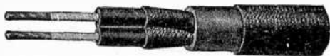
FIG. 5,100.—Reinforced cord. Used in dry places for portable lamps, fans, heavy pendants and other electric devices for which type C Lamp Cords are inadequate. Two untinned conductors, sizes 10 to 18, A.w.g. , bunched. Separator, soft cotton wind. Insulation on each conductor, "Black Core" rubber compound. Covering over insulation, one soft cotton braid. Grouping of conductors, twisted. Insulating belt, "Black Core" rubber compound. Covering over belt, one glazed cotton braid.
