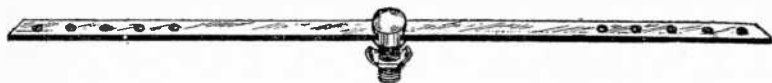
FIG. 5,615.—Austin straight bar hanger and stud. The stud is slotted allowing free movement along the bar, yet may be easily tightened by the locknut in any selected place, making it possible to set box at desired spot although conduit may bear a little off length.
