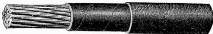
FIG. 5,072.—Apparatus Cable. Used for connecting machine terminals to brush holders, for transformer leads and similar purposes where great flexibility is required and the working pressure does not exceed 750 volts. One conductor. Sizes up to 2,000,000 c.m. Stranding, extra flexible. Insulation, varnished cambric or rubber compound. Thickness of insulation, same as code standard for 0-600 volt rubber. Covering over insulation, one dry cotton braid. (Sometimes a weatherproof braid is specified.)
