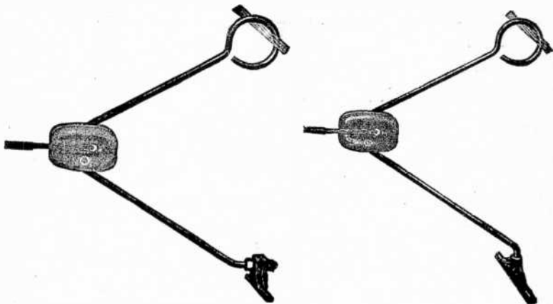
FIGS. 5,950 and 5,951 — Catenary materials 7 . Ohio Brass Co. pull off hangers. Used in curve construction where it is necessary to pull messenger and trolley into position. Consists of a \frac{1}{2} in. steel rod shaped as shown. The upper end is formed into a loop which gives a flexible connection with the messenger and the lower end is equipped with a malleable iron clamp which will fit 2-0 to 4-0 grooved trolley wire or an extruded ear which fits 4-0 grooved wire. Rod can be installed in a porcelain strain insulator as shown, before clamp is installed.
