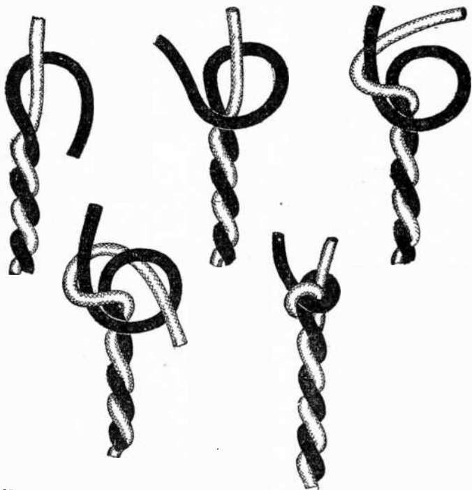
Figs. 5,265 to 5,269.—Method of making the "Underwriters Knot" progressively shown.
