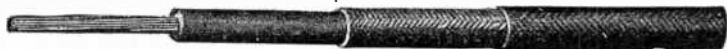
FIG. 5,074.—Automobile lighting wire. Used for connecting automobile lights with the switch and source of current supply. One wire 10 to 14 A.w.g. stranded. Insulation, "Black Core" rubber compound. Covering over insulation, one varnished soft cotton braid 1-64th in. thick. Outside covering one (2 coat) varnished braid, 1-64th in. thick.
