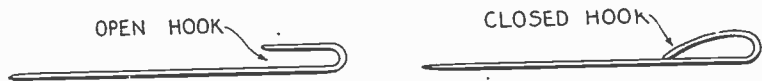
FIGS. 5,647 and 5,650.—Open and closed snake hooks. The open hook is used in hooking one snake to another. The closed hook is used for fishing.
