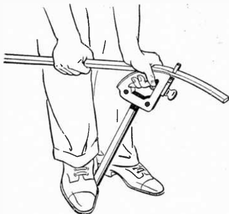
FIG. 5,327.—Correct use of bending tool in bending National moulding. In bending , the force should be applied near the bending tool; and when a screw hole comes within the length of the two wire two piece moulding to be bent, the pressure should not be exerted too suddenly.
