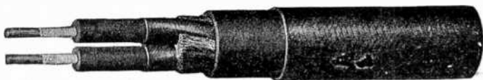
FIG. 5,086.—Deck cable is a portable cable for rough usage in damp places. Two (untinned) conductors, sizes 10 to 18 A.w.g. , bunched. Separator, soft cotton wind. Insulation on each conductor, "Black Core" rubber compound. Covering over insulation, one saturated braid. Fillers, dry jute. Grouping of conductors, twisted. Insulating belt, "Black Core" rubber compound. Thickness of b.lt., \frac{3}{4} ". Covering overall, one saturated braid.
