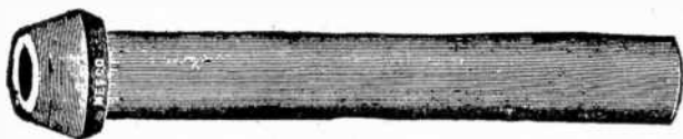
FIG. 5,372.—Porcelain tube as used in knob and tube wiring. The standard tube as used in house wiring comes in all lengths and is \frac{1}{8} in. in diameter.
