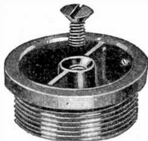
FIG. 5,699.—National type B plug. When adjusted it protrudes very slightly above top rim of duct outlet. This shallow plug is intended for use where duct is installed under wood or marble, as it is impracticable to cut a number of holes in the underside or through these materials to fit over a type A plug protruding above level of concrete fill; when the type B plug is used, holes need be cut only where duct outlet is to be used for service. Other outlets are located by marker screws, or by measurement.
