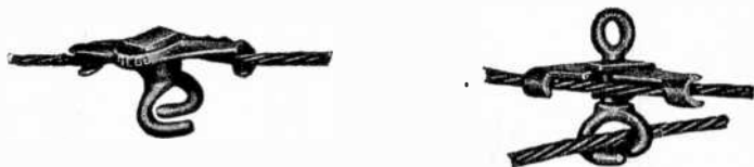
FIGS. 5,937 and 5,938.— Catenary materials 2. General Electric span wire messenger supports. They are used for the attachment of the messenger cable to the cross span and are used throughout tangent and curves in cross span construction, except when replaced at anchorages by anchor clamps. The supports are arranged for adjustment to any angle between the messenger and span wires. Fig. 5,937, shows the support which is intended for use in ordinary line construction, and fig. 5,938 a support which is especially adapted for use in yards where many tracks are spanned, the regular cross span wire being picked up at the messenger supports and attached to another cross span wire located above. Both supports are arranged for \frac{3}{8} inch span wire and \frac{3}{8} inch to \frac{1}{2} inch messenger wire.
