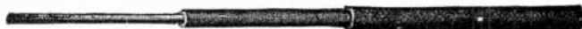
FIG. 5,085.—Fixture wire. Used in wiring electric light fixtures. One conductor, standard sizes, 16 and 18 A.w.g. , solid or stranded. Insulation, "Black Core" rubber compound. Covering over insulation, one saturated braid, at least \frac{1}{4} " thick.
