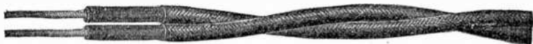
FIG. 5,089.—Lamp cord. Used for pendants in dry places and also for portables in dry places where the usage is not hard. Two untinned conductors, sizes 10 to 18 A.w.g., bunched. Separator, soft cotton wind. Insulation on each conductor, "Black Core" rubber compound. Covering over insulation, one silk cotton, or mercerized cotton braid. Grouping of conductors, twisted pair. The braid is made in all standard colors.
