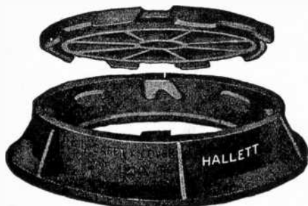
FIGS. 6,018 and 6,019.—D & D manhole cover. The cover does not rest on top of the lugs, but on the 45° angle side of the lugs and is held in place by the 85° side. The cover is opened by using two short bars which can be operated by one man by simply prying first on one bar and then reversely on the other until the cover leaves its seat and can then be carried off without any trouble. Another method is to insert a large cold chisel in the keyhole of the cover, and strike it a few heavy blows with a hammer which will loosen the cover in a few minutes even in below zero weather.
