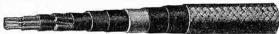
FIG. 5,076.—Basket weave armored cable. It consists of a wire braid similar in construction to the ordinary cotton braid, used for covering wires. It is usually made of galvanized soft steel wire, but it is sometimes made of brass or copper. The warp and woof of this fabric, each consists of between five and fourteen ends, depending upon the size of cable, the usual size of wire being .0126" diam. The strands or ends are laid closely together, flat and parallel, firmly binding the core. Basket weave is used for two purposes. First as a mechanical protection, and second, as a means of grounding the outside of high voltage cables, in order to prevent static disturbances. The former application is by far the more important.
