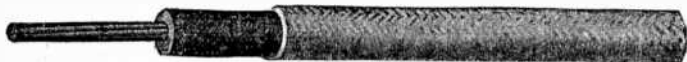
FIG. 5,087.—Flame proof cable. Used about power houses in the vicinity of switchboards and apparatus where special fire proof protection is desired. This method of protection consists essentially in impregnating the braided covering with a flame proof paint, and may be used in connection with any conductors having braided covering, when so specified.
