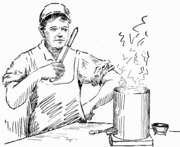
FIG. 5,186.—Method of judging the heat of a soldering bit by holding it near the face.
