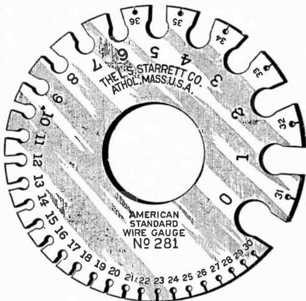
FIG. 5,069.—Brown and Sharpe (B. & S.), or American Standard wire gauge. This gauge was adopted by the brass manufacturers Jan., 1858. The cut is full size, and therefore shows the actual sizes corresponding to the gauge numbers.
