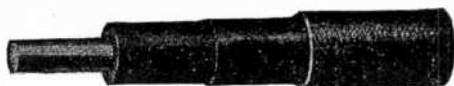
FIG. 5,082.—Single conductor code house wire. Used in pairs for house wiring or with twin wires for the neutral of three wire systems. One conductor, sizes, 0000 to 14 A.w.g. , solid. Insulation, "Black Core" rubber compound. Covering over insulation one saturated braid, two saturated braids or rubber filled tape and one saturated braid.
