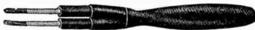
FIG. 5,079.—Canvasite cord is a type of lamp cord specially adapted to rough usage. Two conductors. Range of sizes, 10 to 18 A.w.g. , bunched. Separator, soft cotton wind. Insulation on each conductor, "Black Core" rubber compound. Covering over insulation, one saturated braid. Grouping of conductors, twisted. Covering overall, one saturated braid.
