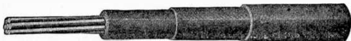
FIG. 5,081.—Car lighting wire. Used for wiring railroad cars illuminated by axle driven dynamos. One conductor. Standard sizes, 0 to 16 A.w.g. Insulation, 30 per cent hevea rubber compound. Covering over insulation, 16 to 8 A.w.g., one saturated braid, 6 to 0 A.w.g., two saturated braids.
