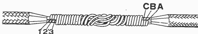
FIG. 5,171.— Multiple wrapped splice 3. Wrap tightly the strands of one cable around the laid up portion of the other cable. Similarly wrap the strands of the other cable.
