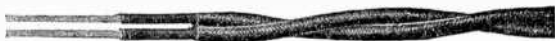
FIG. 5,078.—Brewery cord. Used for extension lights in damp places and differs from ordinary lamp cord only in that the braids are weatherproof instead of dry glazed cotton. Two conductors. Range of sizes, 10 to 18 A.w.g. bunched. Separator, soft cotton wind. Insulation on each conductor, "Black Core" rubber compound. Covering over insulation, one saturated braid. Grouping of conductors, twisted pair.
