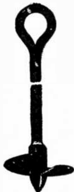
FIG. 5,823.—Stombaugh guy anchor. It is made of cast iron and can be screwed into the ground like an auger.
