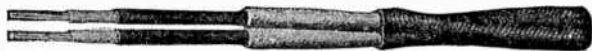
FIG. 5,088.—Heater cord. Used for the wiring of domestic heating apparatus, such as heaters, stoves, etc., requiring over 250 watts. Two untinned conductors, sizes 10 to 18 A.w.g., bunched. Separator, soft cotton wind. Insulation on each conductor, "Black Core" rubber compound. Covering over insulation, one asbestos braid. Grouping of conductors, twisted. Covering overall, one glazed cotton braid.
