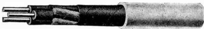
FIG. 5,092.—Three conductor lead covered cable, solid. Used for three-phase circuits under the same conditions of service as single conductor solid lead covered wire. Three conductors, sizes to 14 A.w.g. solid. Insulation on each conductor, "Black Core" rubber compound. Covering over insulation, one rubber filled tape. Grouping of conductors, twisted. Fillers, jute. Covering over jute, one rubber filled tape. Covering overall, lead sheath.
