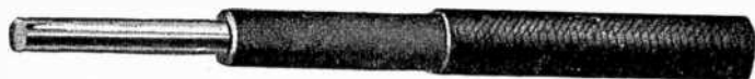
FIG. 5,099.—Rubber insulated signal wire for 660 volts or less. One or two conductors, sizes 0 to 18 A.w.g. , solid. Insulation on each conductor, Railway Signal Association compound. Covering over insulation, one cotton braid, \frac{3}{16} " thick, weather proof.
