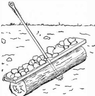
FIG. 5,822.—Guy anchor log in position.
