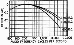
FIG. 8-Typical radio receiver, fidelity characteristics.
