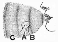
FIG. 7,4F0.—Microscopic view showing molecules of air at 1, in fig. 7 478. In a spoken word, or it. any musical sound, the molecules dance back and forth as in fig. 7,481.
