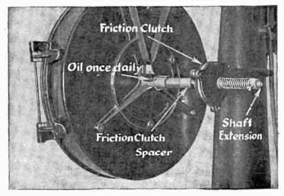
FIG. 7,914 .- Pacent friction clutch spacer with oiling indications.
