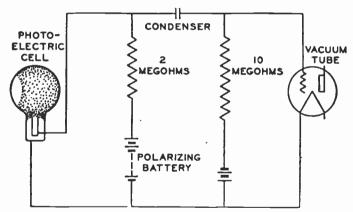
FIG. 7,830.—Photo-electric cell. The characteristic of this device is that when it is polarized by a proper voltage and is used within proper limits the current through it is proportional to the incident light.
