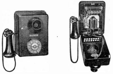
FIGS, 7,634 and 7,635.—Kellogg common battery telephone; enclosed gong wall type arranged for automatic dial. Fig. 7,635 open view showing interior construction.
