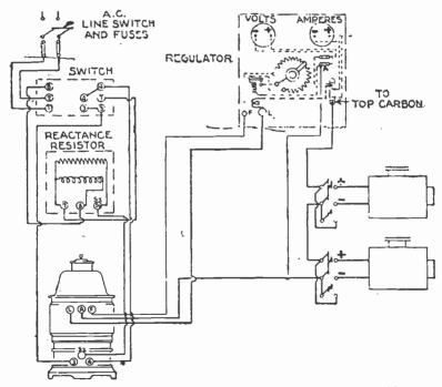
FIG. 7,931.—Wiring diagram of double arc single phase series arc transverter with control panel. To start throw the handle of the switch to the position marked start. Fold there until unit comes up to speed, then throw over to position marked ran. The starting time is approximately 20 to 30 seconds.
