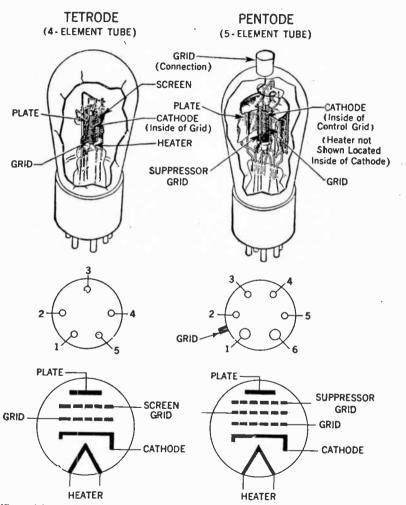
Views of four and five element vacuum tubes, showing arrangement of prongs and wiring symbols.
