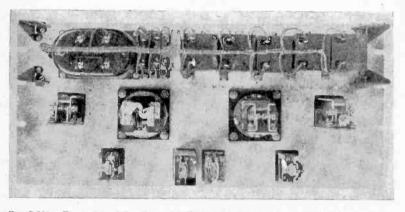
FIG. 7,5%0.—Front view of signaling unit. When the switchboard operator presses the ringing key at the switchboard, ringing current of 20 cycles is applied to this unit which causes by modulation spurts of the carrier current to be sent out over the toll line to the distant switchboard which is equipped with a similar unit. The signals at the receiving end are demodulated and a series of relays operate in the similar signaling unit causing the tamp associated with the toll line to light.
