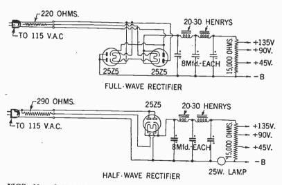
FIGS. 12 and 13—Illustrates two transformerless power supplies, for fullwave and half-wave rectification respectively. Here a line cord resistor is utilized to drop the line voltage to that necessary for the filaments of 25Z5 tubes. The third element in the line cord resistor brings the full line voltage for the plate of the tubes. Power Supply Units
