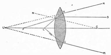
FIG. 7,769.—Virtual focus in double convex lens. In the figure, L is the position of the luminous source between the principal focus and the lens; I' is the principal focus, and L', the virtual focus corresponding to the position L of the luminous source.
