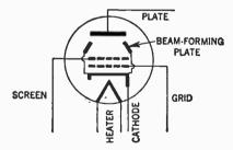
FIG. 12.-Conventional representation of beam power tube.
