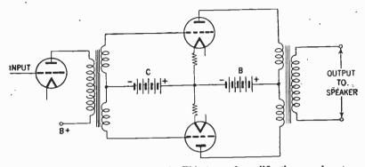
FIG. 15—Push-pull amplifier circuit. This type of amplification requires two identical tubes in each stage. The grids of the tubes are not connected together, as in the case of parallel operation, but are connected to opposite ends of a mid-tapped transformer secondary. The mid tap is used as a common connection for making connection to the negative bias voltage of the grids.
