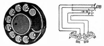
FIGS. 7,632 and 7,633 .- Assembled dial and wiring diagram.
