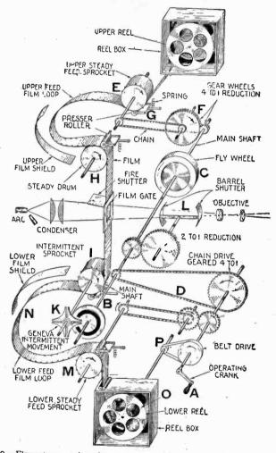
Fig. 7,7°0.—Elementary moving picture machine without case showing essential parts arranged to illustrate plaunly the motion system.
