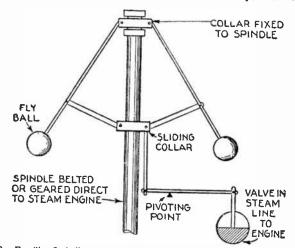
F16. 7.902.—Familiar fly ball steam engine governor showing how sensitivity may be changed by moving the pivoting point to the left or right.
