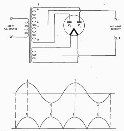
FIG. 5.-Connection diagram and deniction of the action of a full-wave rectifier tube.
