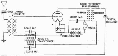
FIG. 28—Diagram showing typical reflex circuit.
