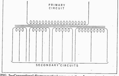
FIG. 2-Conventional diagrammatical representation of power transformer for 5 to 9 tube sets.
