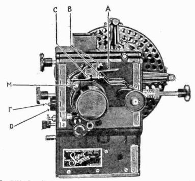
FIG. 7,824.—Super-Simplex projector; view showing adjusting leter, threading and framing lamp, etc. To replace lamp: Loosen screws which hold switch assembly and lamp socket in lacquered barrely use entire assembly may then be removed and a up readily replaced
