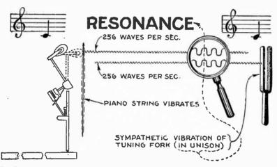
FIG. 7.182.—Sympathetic vibration of tuning fork with struck piano string when tuned to same pitch, illustrating the wave theory of radio.
