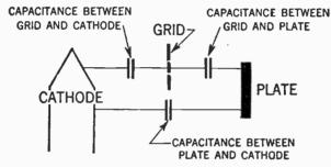
Fig. 9.-Diagram showing inter-electrode capacitances in a triode.
