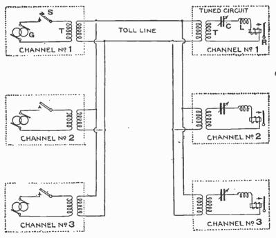
FIG. 7,575.—Simolified Multiplex circuit, consisting of three channels, each equipped alike and arranged to opera e si nultaneously over the same toll line. Each sending station is equipped with a high frequency generator G, a sending key S and a repeating coil T. Each receiving station is equipped with a repeating coil T, a variable condenser C, an inductance L, and a sounder relay R.
