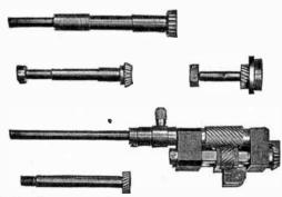
Frcs. 7,79? to 7,796.—Simplex gears. The bevel and intermediate gears are made of formica, which material absorbs noise and damps the ring of metal gears.
