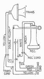
FIG. 7,524.—Wiring of desk stand. FIG. 7,525.—Coin box telephone.
