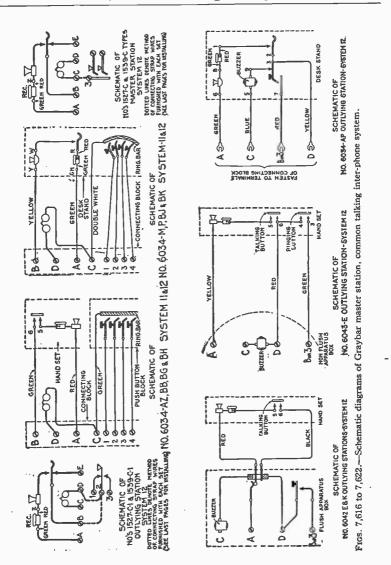
In operation, when a push button is depressed marked with the name or number of the outlying station wanted, the bell at that station only will ring.
