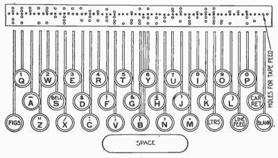
FIG. 7,739 .- Teletype keyboard and corresponding code combination.
