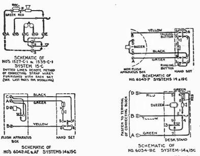
FIGS. 7,59? to 7,595—Schematic diagrams of Graybar code ringing, common talking interphone system.
