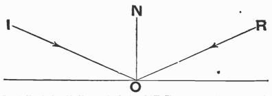
FIG. 7,75).—Angles of incidence and reflection. LAW: The angle of reflection is equal to the angle of incidence. The ray IO is called the incident ray; OR, reflected ray; angle ION, angle of incidence; angle NOR, angle of reflection; NO, normal or perpendicular to the reflecting surface.
