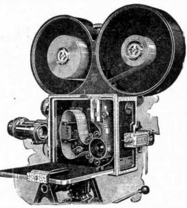
FIG. 7,787.—Bell & Howell motion picture camera; view showing camera and magazine interiors exposing film movement mechanism and threading of film.
