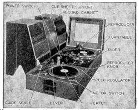
FIG. 7,876.—Non-synchronous double turntable cabinet for disc reproducing where records are not synchronized with the film. Each turntable is provided with a pick up and means for locating it accurately upon a record, and a fader to make possible continuous playing. The same amplifier and loud speakers are used as for the synchronized speech and music.
