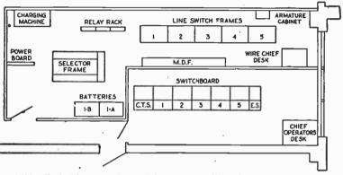
FIG. 7,686.—Typical floor plan of three digit step-by-step Private Branch Exchange.
