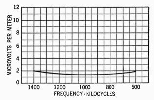
FIG. 7-Typical radio receiver, sensitivity characteristics.
