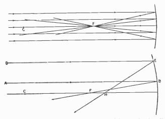
Ftgs. 7.763 and 7.7°4.—The principal focus. By definition. it is that point where all the mays parallel with the principal axis meet after reflection, as, for instance, the mays from a source of light at a minimite distance for a the mirror. The sum is so fur distant that is mays are practically parallel. When there are reflected upon a concave mirror they are reflected to the principal focus F; forming a point of intense light and heat.
