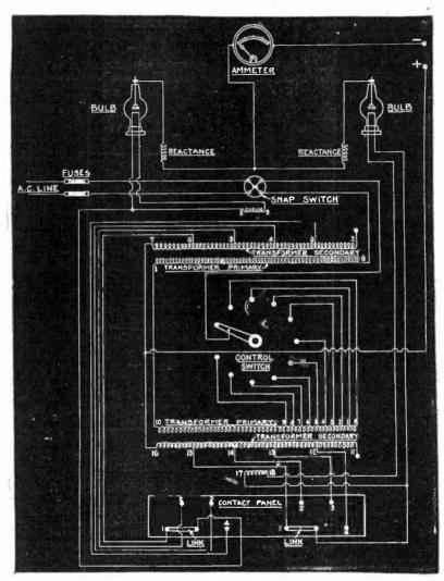
FIG. 7,933 .- Wiring diagram of Forest M. P. 30 rectifier.
