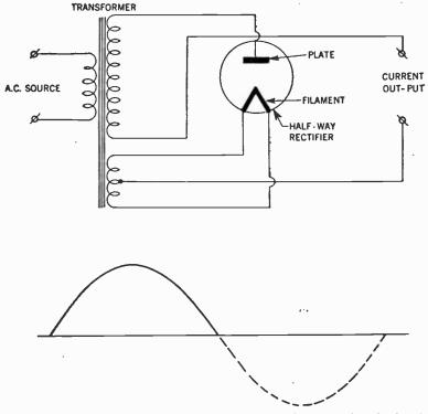
FIG. 4.—Connection diagram of the half-way rectifier. The rectified current is depicted on the upper half of the wave diagram.
