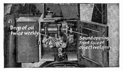
FIG. 7,917 .- Pacent optical chamber with oiling indications.
