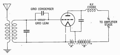
FIG. 26-Detector circuit grid-leak and condenser method.
