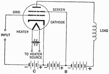
FIG. 10.-Connection of electrodes of a screen gride tube.
