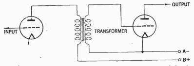
FIG. 32-Method of inter-stage connection of *transformer coupled* audio ferguency amplifier.
