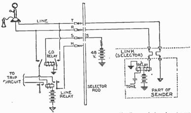
FIGS. 7,664 and 7,675.—Line finder brushes stopped at calling line terminals and sender connected. The calling telephone receives the "dial" tone.
