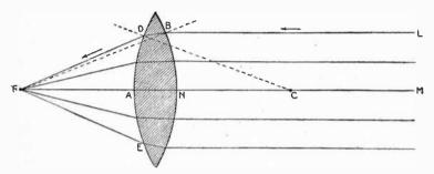
FIG. 7,765.—Principal focus in double convex lens. CASE I: Rays from luminous sources parallel with the principal axis.
