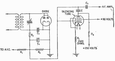
FIG. 14--Automatic tone control circuit.
