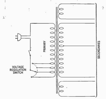
FIG. 3-Power transformer circuit showing voltage regulation switch.
