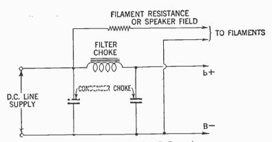
FIG. 9-Conventional filter system used on D.C. receivers.
