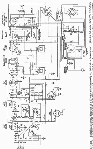
I.f. frequency 456 kilocycles. Line voltage 117 volts a.c. 50 to 60 cycles. FIG. 7,335.—Schematic circuit diagram of a 12-tube superheterodyne, 3-band radio receiver. 12-S-245, 12-S-265, 12-S-266, 12-S-267, 12-S-268.) *I.f.* frequency 456 kilocycles. Line v. Power consumption 110 watts.
