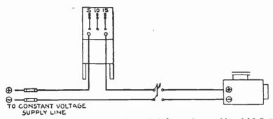
FIG. 7,923,—Hertner wiring diagram showing method of connecting type AA, and A ballast rheostats.
