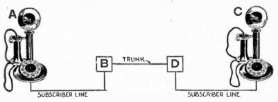
FIG. 7.628.—Simplified dial telephone system. A, telephone subscriber with number ATLantic 2357; B. Atlantic central office; D, Maytlower central office; C, telephone subscriber with number MAYtlower 7348.
