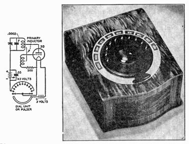
FIGS. 10 and 11—Fig. 10 shows circuit diagram of the portable control box. Impulses sent out from the box are picked up by the five tube unit (fig. 12) and amplified to the proper degree to actuate the tuning mechanism shown in fig. 13. All control boxes are adjusted to use one of the five frequencies specified above.
