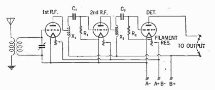
FIG. 13-Two stage impedance coupled radio frequency amplifier.
