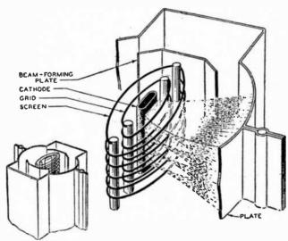
FIG. 13 .- Internal structure of beam power tube.
