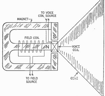
FIG. 5-Simplified diagram of dynamic speaker units shown in fig. 4.
