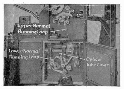
FIG. 7,394.—Pacent projector head and sound head showing proper size for lower normal running loop between constant speed sprocket and take up sprocket.
