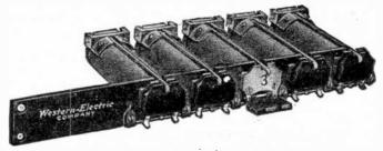
FIG. 7,528.—Mounted trunk drops. Tubular trunk drops are mounted on a metal strip each being held by two small screws underneath the drop shutter. The tubular casing of each drop is soft iron inside of which is the drop winding; the ends of the coil wires terminating at lugs which protrude fron the casing and are insulated therefrom. The drop shutters are then screwed fast to the metal strip and adjusted so that they may fall easily when the armature is held up by the magnet.
