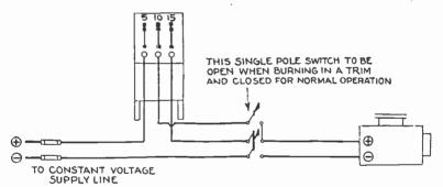
FIG. 7,929.—Hertner wiring diagram showing method of connecting types J, K and L, ballast rheostats.
