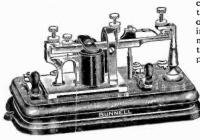
closed, the coil A-D be opened, as in fig. 7,720, the core will be magnetized due to the presence of current in the coil A-C while no current exists in coil A-D, the latter no longer neutralizing the magnetic effect of the former. The armature, therefore, is attracted and held in the "closed" position as shown in fig. 7,720.
