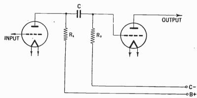
FIG. 80--- finterstage coupling in a resistance coupled audio frequency amplifier.
