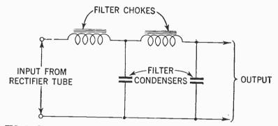
FIG. 6-Choke-input filter.
