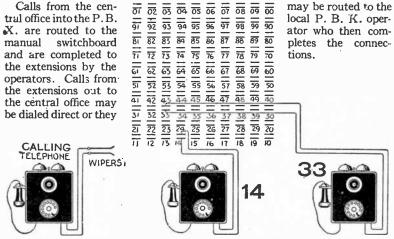
FIG. 7, 687.—Diagram of line bank contacts, associated with each connector and numbering system of the telephone lines of which they are the terminals. The number of any set of terminals can be determined by noting the number of vertical and sidewise steps the wipers must be given to reach that set, remembering that ten steps are always represented by zero. Thus six vertical steps and ten rotary steps would cause the wipers to reach contact No. 60.
