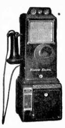
The operator in the Central Office can either collect or return the coin by operating a *collect* or *return* key.
