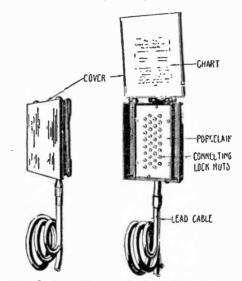
FIGS. 7.526 and 7.52<sup>°</sup>.—Outdoor cable connecting box. This device is placed in a back yard in cities, or on a pole in the country, and accommodates the two line wires for each telephone in a block or street.
