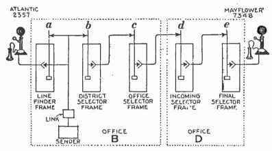
FIG. 7,531.—Panel dial system—routing of a call. a, line finder; b, district selector; c, office selector; d, incoming selector; e, final selector.
