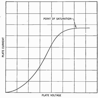
FIG. 6 .- Characteristic curve of a diode.
