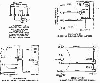
FIGS. 7,628 to 7,631.—Schematic diagrams of Graybar master annunciator common talking interphone system.
