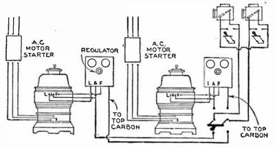
FIG. 7,934.-Wiring diagram for two double arc transverters connected for emergency use.
