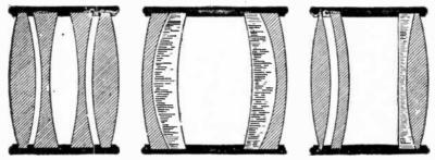
FIGS. 7,780 to 7,782.—, acious achromatic lenses. FIG. 1,780 and fig 7,781 are types usually used in photography, and fig. 7,782, a combination used in motion picture and stereopticon projection.
