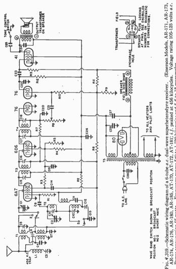
AR-174, AR-176, AR-180, AR-185, AT-170, AT-172, AT-181; *i.j.* peaked at 456 kilocycles. Valtage rating 105-125 volts a.c. Power consumption 55 watts. Frequency ranges 540 to 1,730 kilocycles and 5.6 to 18 megacycles.
