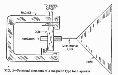
Magnetic Speakers.—In this type the moving iron driving type is employed. The principle of operation is based on the varying of the magnetic polarity of the armature. These variations are caused by the electrical impulses flowing through the coil winding which encircles the armature. The movement to the armature is effected by the induced magnetism, causing it to oscillate between the two poles of the permanent magnet.
