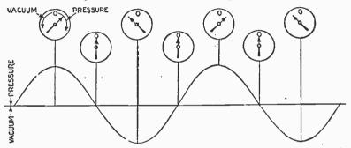
FIG. 7,843.—Diagram illustrating pressure variations due to sound waves. It should be noted that the type gauges shown, register pressure above atmospheric when the pointer moves to the right of the vertical, and vacuum or pressure below atmospheric when it moves to the left of the vertical.
