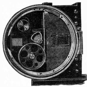
FIG. 7, 89.—Bell & Howell camera. Front view with turret plate and shutter removed showing focusing and photographing apertures; shuttle operating cam, part of brake mechanism and opening for mounting focusing magnifier above focusing aperture.
