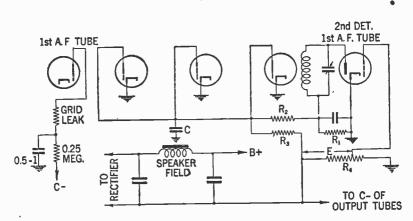
FIGS. 42 and 43—Grid bias method when receiver is equipped with automatic volume control.
