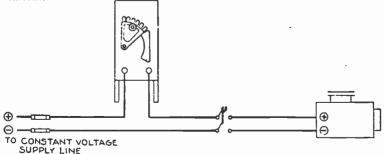
FIG. 7 925.—Hertner wiring diagram showing method of connecting types B, C and D, balast rheostats. 2. The lens system;
