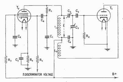
FIG. 4-Typical control circuit diagram.
