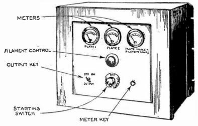
FIG. 7,916 .- Western Electric type 46-B amplifier.
