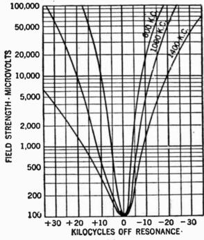
FIG. 5-A typical radio receiver selectivity curve.
