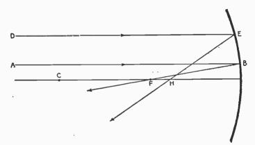
FIG. 7,777.—Spherical aberration. The reflected rays of concave spherical mirrors do not meet at exactly the same point. For instance, the ray AB, will be re-acted to F, but DE will be reflected to II, a point closer to the mirror. This is called *spherical aberration*. It has been observed that the reflected rays only pass through a single point when the aperture of the mirror does not exceed 8 or 10 degrees.
