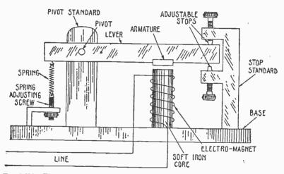
FIG. 7,696 .- Elementary sounder showing essential parts.
