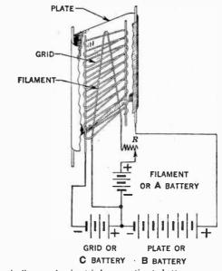
FIG. 7.-Schematic diagram showing triode connection to battery.
