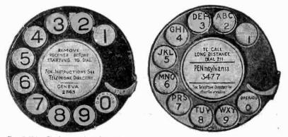
FIG. 7,636.—Single central station stops. FIG. 7,637.—Multi-central station dual showing central station letters, and numerals.
