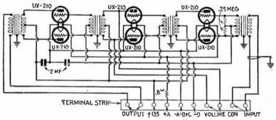
FIG. 7,953 .- Wiring diagram for voltage amplifier.
