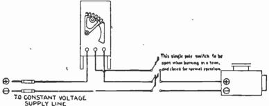
FIG. 7,924.—Hertner wiring diagram showing method of connecting types G and H ballast rheostats.
