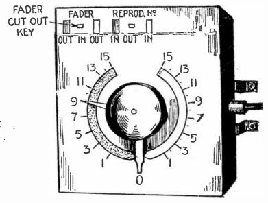
FIG. 7,915 .-- Western Electric fader.
