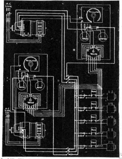
FIG. 7,957 --- Wiring diagram showing installation of two multiple arc units in parallel and control panel. Ans.—Fuses may be omitted where an extremely short tap from a No. 10 main is connected by No. 14 wire to a cut out or wherever the fuse in the larger wire will protect the smaller wire.
