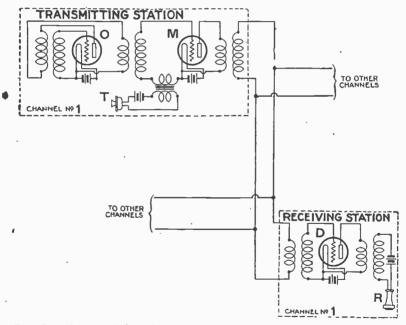
FIG. 7,576.—One channel of a carrier current telephone circuit the transmitting station consists of: O, vacuu 1 tube oscillator circuit, which generates the high frequency carrier current; M, vacuum tube m dualator circuit, which impresses the voice currents on the carrier current; T, transmitter. T is receiving station consists of: D, vacuum tube demodulator circuit, which separates the voice currents from the carrier current wave; R receiver which reproduces the speech.
