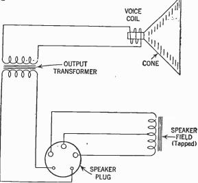
FIG. 7.—Schematic diagram of connections to speaker by means of plug-cable arrangement.
