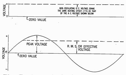
FIG. 44-Illustrating comparative values of r.m.s. and peak voltage in an alternating current.
