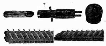
FIGS. 7,553 to 7,557.—Miniature electric lamp and parts. The lamp fig. 7,553 tits into socket, fig. 7,555, and the lamp cap fig. 7,555 fits at end of lamp socket. The glass of the lamp cap may be white opalescent, red, or green, or it may be marked with black bars or a dot. Figs. 7,556 and 7,557 shows hard rubber strips fitted with lamp sockets similar to the one of fig. 7,554.
