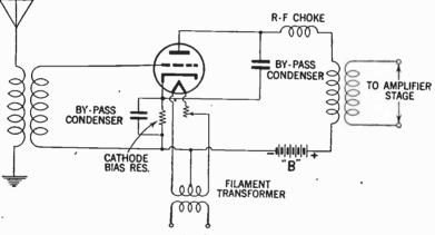
FIG. 25-Grid-biased detector circuit.
