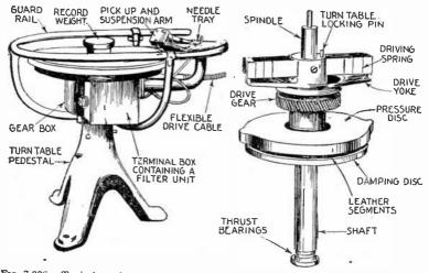
FIG. 7,885.-Typical synchronous turntable showing construction.
