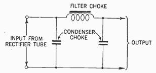
FIG. 7—Condenser-input filter.
