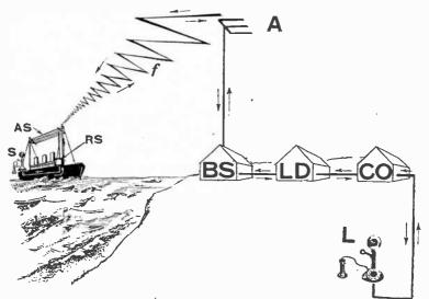
FIG. 7,531 —Ship to shore communication; simplified diagram showing how a telephone conversation is established between a ship at sea and a land station. L, telephone station in a residence or in an office; CO, local telephone central office; LD, long distance telephone exchange; BS, radio sending and receiving station on land; A, aerial on land; f, radio wave; AS, aerial on ship; RS, radio receiving and sending set on ship; S, telephone station on ship.
