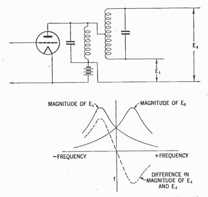
FIG. 2—Diagram and plotted curves illustrating how the potentials at either end of secondary are 180° out of phase.
