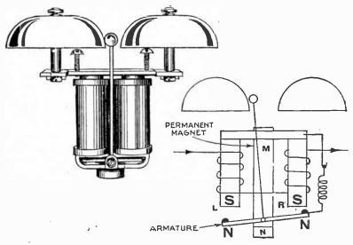
FIGS. 7,516 and 7,517 .- Ringer and diagram of its operation.
