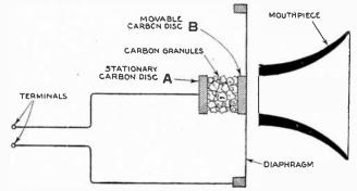
FIG. 7,479 .-- Simple electric telephone transmitter.
