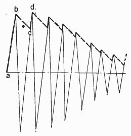
FIG. 22-Diode detector characteristics.
