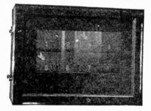
**FIG.** 7,6°5.—Graybar master annunciator, common talking system electric reset annunciator. The drop indicator is a white arrow which points directly at a white drop number; it can be seen from any angle. The audible signal is a new type double adjusting buzzer.
