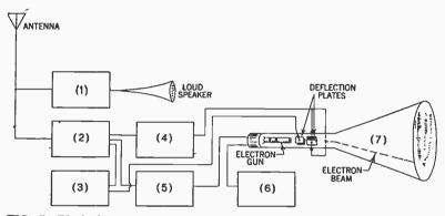
FIG. 7—Block diagram indicating fundamental unit that makes up a television receiver.
