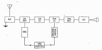
FIG. 1-Conventional block diagram of an automatic radio frequency control circuit.
