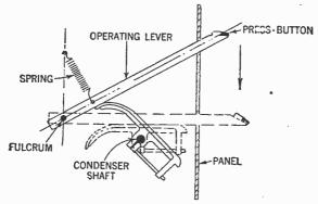
FIG. 9—Method of condenser control by lever system. When pressing the lever it contacts the rounded portion of control bar and so turns the condenser until the flat position is purallel with the lever.
