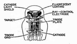
FIG. 34—Internal construction of electron ray indicator tube. (Courtesy R.C.A. Mfg. Co. Inc.)
