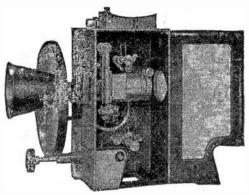
FIG. 7,912.—Superior projector. Head mechanism, film side showing new rear shutter, new framing device, mask on aperture to cut of sound track in connection with sound film.
