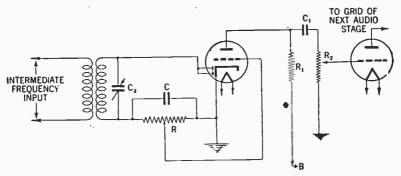
FIG. 23-Diode-biased detector circuit.
