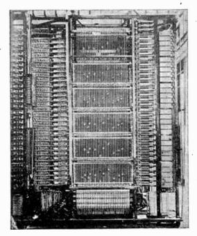
FIG. 7,654.—Panel type selector frame.
