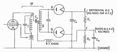
FIG. 3-Automatic radio frequency control detector diagram.
