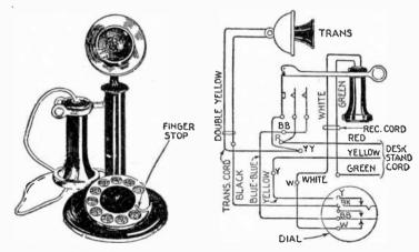
FIGS. 7,629 and 7,630 .- Telephone with dial and circuit diagram.
