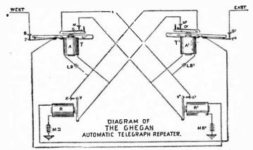
FIG. 7,717.—Diagram of Ghegan automatic repeater. Its principle of operation is oased upon the fact that an armature, on being drawn toward a magnet becomes itself magnetic by induction, and that the closer it approaches the magnet core, the stronger the magnetism becomes. The circuits and operation are further explained in the accompanying text.
