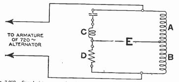
FIG. 7.903.—Sound picture governing circuit proper. Voltage E, shifts 180° in phase as the speed changes from any value below 1,200 r.p.m. to any value above it.
