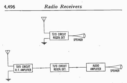
FIGS. 1 and 2-Block diagrams showing essential units of a regenerative and a tuned radio frequency regenerative circuit respectively.
