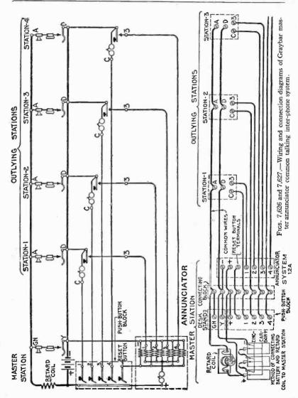
Master Annunciator: Common Talking System.—This system meets the requirements of school service. The system consists of an annunciator for use in the principal's office for registering the calls from the class rooms, also a desk stand and a push button block for calling each class room inter-phone.
