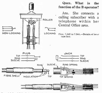
FIGS. 7,545 to 7,517—Jack and plug details showing how connections are made by inserting a cord plug into a jack. Each jack has three contacts known as tip, ring, and sleeve, and the cord plug has tip, ring and sleeve to correspond. Hard rubber is used for insulation of the contacts.
