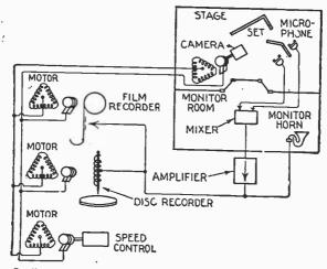
FIG. 7,854.—Studio sound recording system in its simplest form. The essential parts of such a system consist of micropno.e pick ups on the stage, a mixer and volume control in the monitor room, system and monitor amplifiers, recording machines, and a synchronous motor system for synchronizing the recorders with the cameras.
