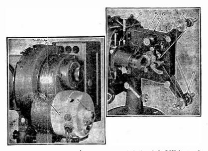
FIGS. 7,920 and 7,921.—Victor Cine projector with oiling indications. In fig. 7,920, locate and oil. 1, main bearing oil tube; 2, front motor bearing tube. Slide cover aside to expose hole: 3, rear motor bearing; in fig. 7,921, locate and oil; 4, cam bearing tube; 5, gear shaft (directly behind lens mount), 6, sprocket shaft tube; 7, upper reel shaft; 8, lower reel shaft; 9, rewind pulley hub.
