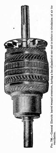
that provision be made to carry off some of this heat to prevent excessive rise of temperature.
