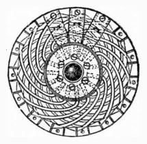
Ftg. 806.—Siemens' bar armature; end view. *Each inductor* in the form of a bar is connected to the next by means of two evolute spiral copper strips, one bending inwardly, the other outwardly, their junction being in some cases secured to a block of wood upon the shaft. Their outer ends are attached to the bars by rivets or silver solder.
