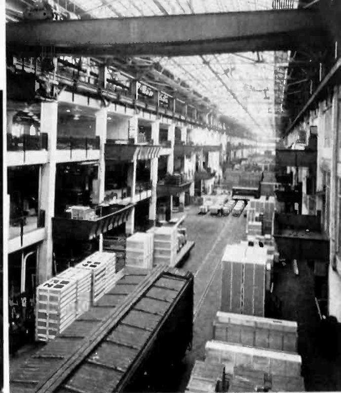
"Crane Court" gets its name from the huge travelling crane which distributes materials.
