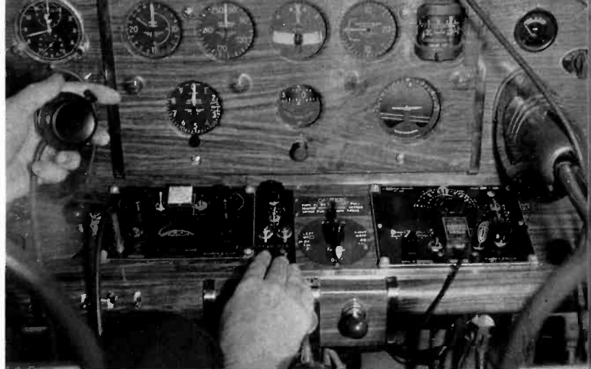
Two sets of Western Electric transmitters and receivers on police planes operate over intermediate... ultra-high frequency bands
