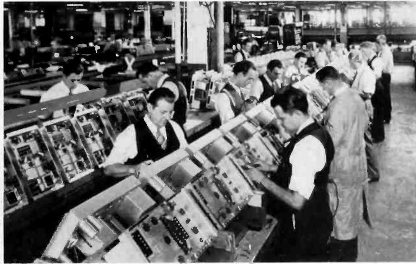
Here's a long line of 118 type amplifiers being assembled and wired on a production basis. The finished units are thoroughly tested before shipment.
