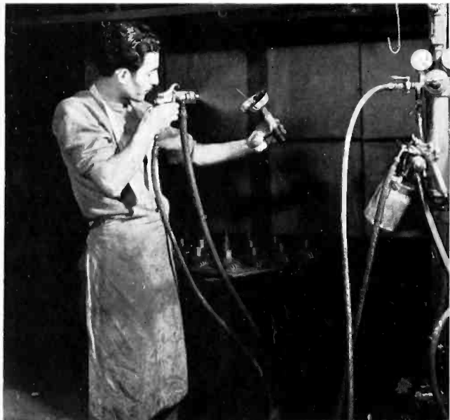
Three layers of lacquer are applied to 639A microphone cases. Transparent lacquer is used for final coating.
