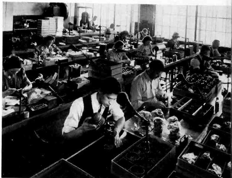
Assembling cardioid microphones in a special double-sealed, air conditioned between operations instruments being assembled are protected by transparent
