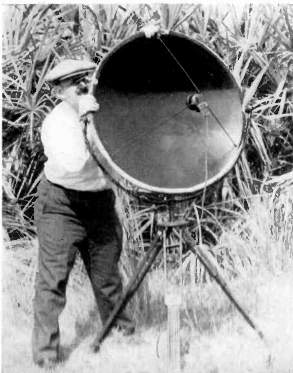
Recording a bird song by means of a Western Electric Microphone attached to a sound concentrator.
