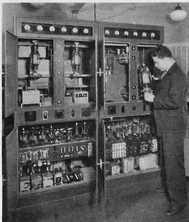
Inspecting one of the 279A Vacuum Tubes used in the 1,000 Watt Western Electric Transmitter which is installed at New York Police Headquarters.
