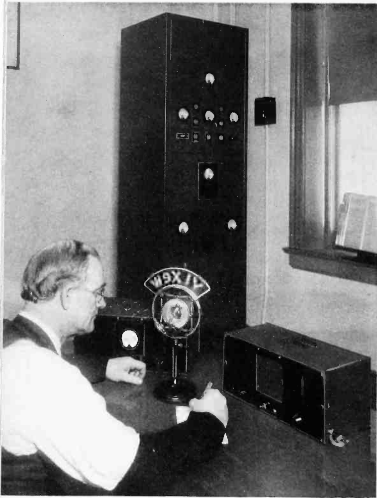
Above: Sergeant Rufus Page operates the 50 Watt Ultra-High Frequency Transmitter. Below: The patrol cars showing the flexible antennas. The men are, left to right, Burt Splitthoff, Chairman of Elgin Police Board, Mayor Myron Lehman and Joseph G. Huber, Chief of Police.
