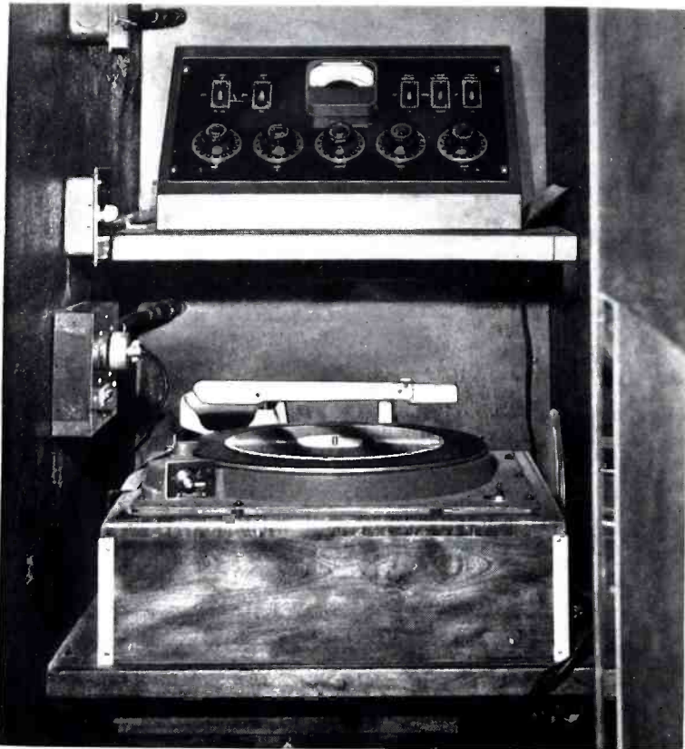
Celestron programs originate at this transcription turntable in main room, or at two additional tables in power room below ground level. Input controls are above turntable.
