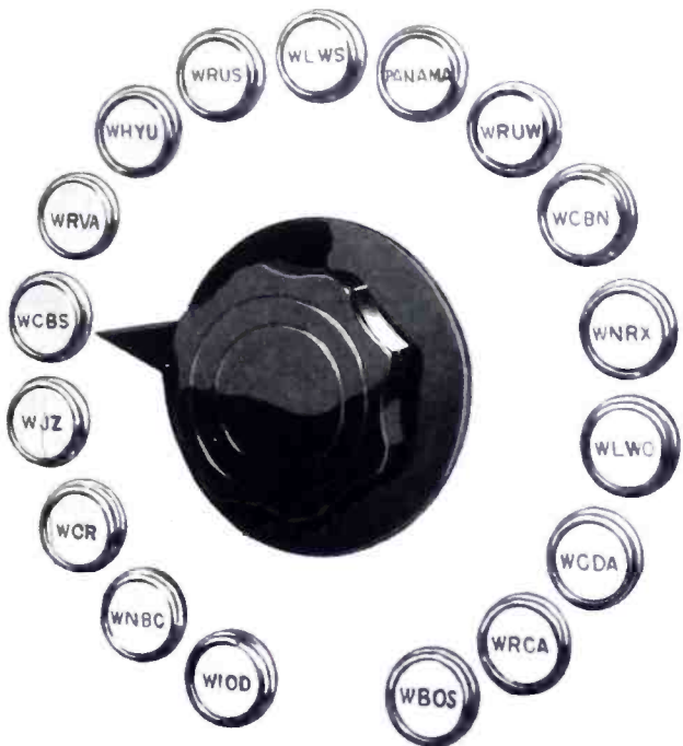
The station selector dial on the control rack for automatic radio tuning. Note shortwave stations on right beginning with "Panama."
