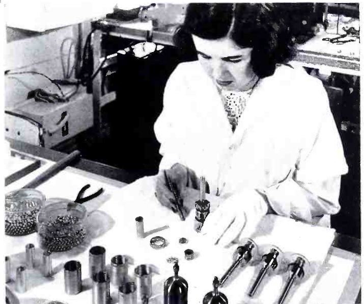
Above: Another view of assembly shows white-gloved worker inserting silvered ball bearings in the rotor of rotating anode X-ray tube, one of the most ingenious and precisely designed electron tubes developed by Machlett.
