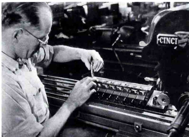
Below: Milling of cathode heads is done to tolerances as close as one ten-thousandth of an inch, to provide the sharply focussed electron beam necessary in certain X-ray tubes.
