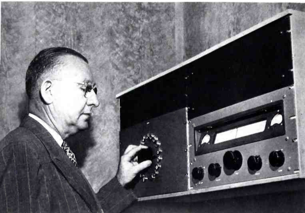
Two views of control center for sound system: left, Publicity Director Wessner adjusting fixed-tuned AM radio, installed next to FM tuner; right, making a store-wide announcement, with switching unit that controls the whole system at his left elbow. Transcription turntable is readily operated from same position.
