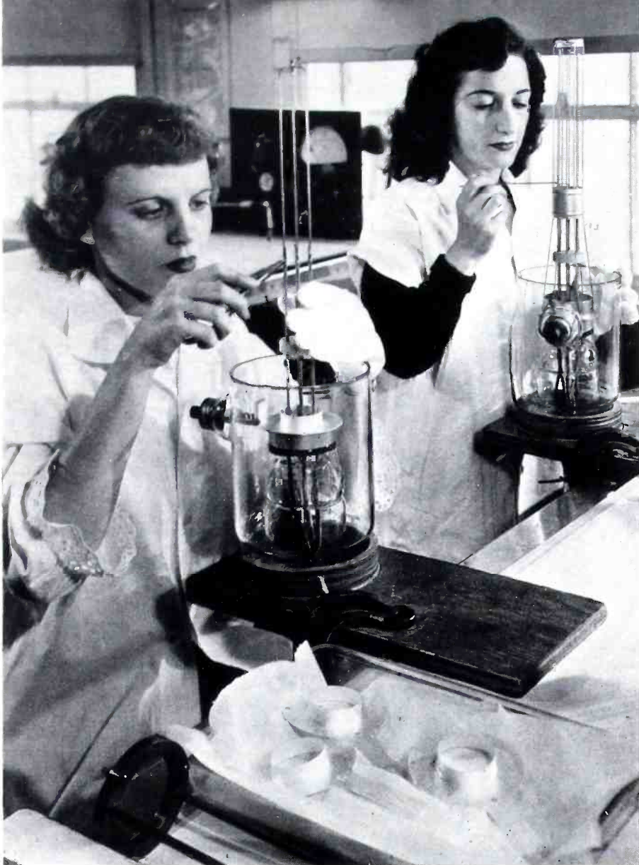
Grid structure is added to high power r-f tube by Machlett workers who maintain strict cleanliness of tube parts. Assembly shop in which girls work has close control of temperature, humidity, all dirt removed from air.
