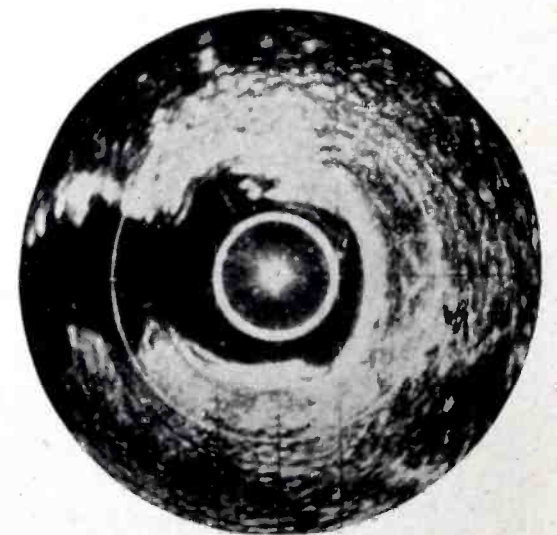
Pinpoint on Tokyo: unretouched photograph of radar PPI scope showing area including Nippon capital.
