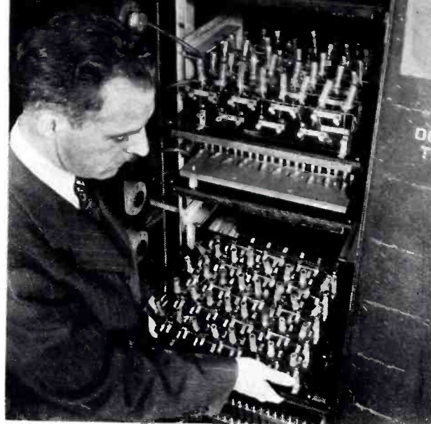
Thermistor aging: racks of Western Electric thermistors are here being placed in aging cabinet in manufacturing process.
