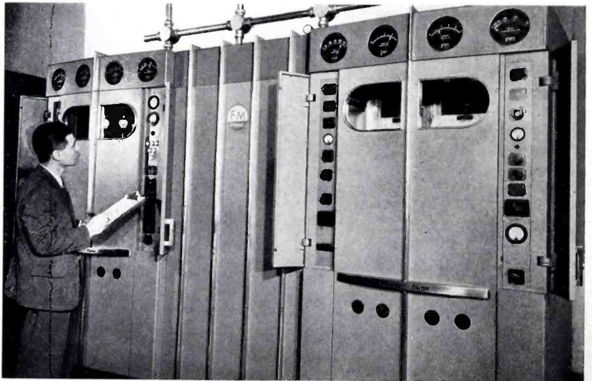
Synchronized frequency control is a feature found only in Western Electric's FM transmitters. This is the 10 KW transmitter, which consists of a high and low power supply and control unit (left); a 10 KW power amplifier (center); a one KW driver and synchronized frequency control unit (right).
