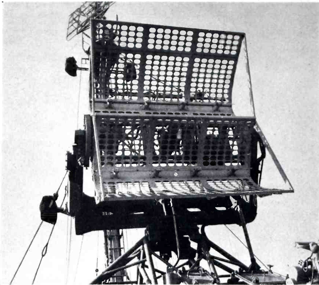
Close-up of one type of antenna used in Western Electric fire control radar systems which point the guns of Navy ships from destroyers to battlewagons. Western Electric supplied more than 6,000 shipboard radars.
