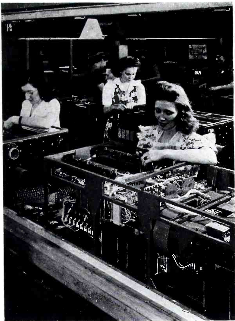
Production of the highly intricate Mark 20 anti-aircraft radar. This is assembly and inspection line of the step-by-step converter unit.
