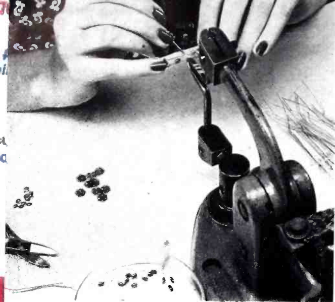
Skilled hands weld bead leads to the wire mount in an intricate operation in thermistor manufacture.
