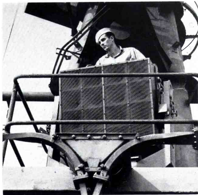
take-offs and landings. Left: Amplifiers and control panels. Above: Movable bull horn, for talking to other ships, can be aimed like a searchlight.
