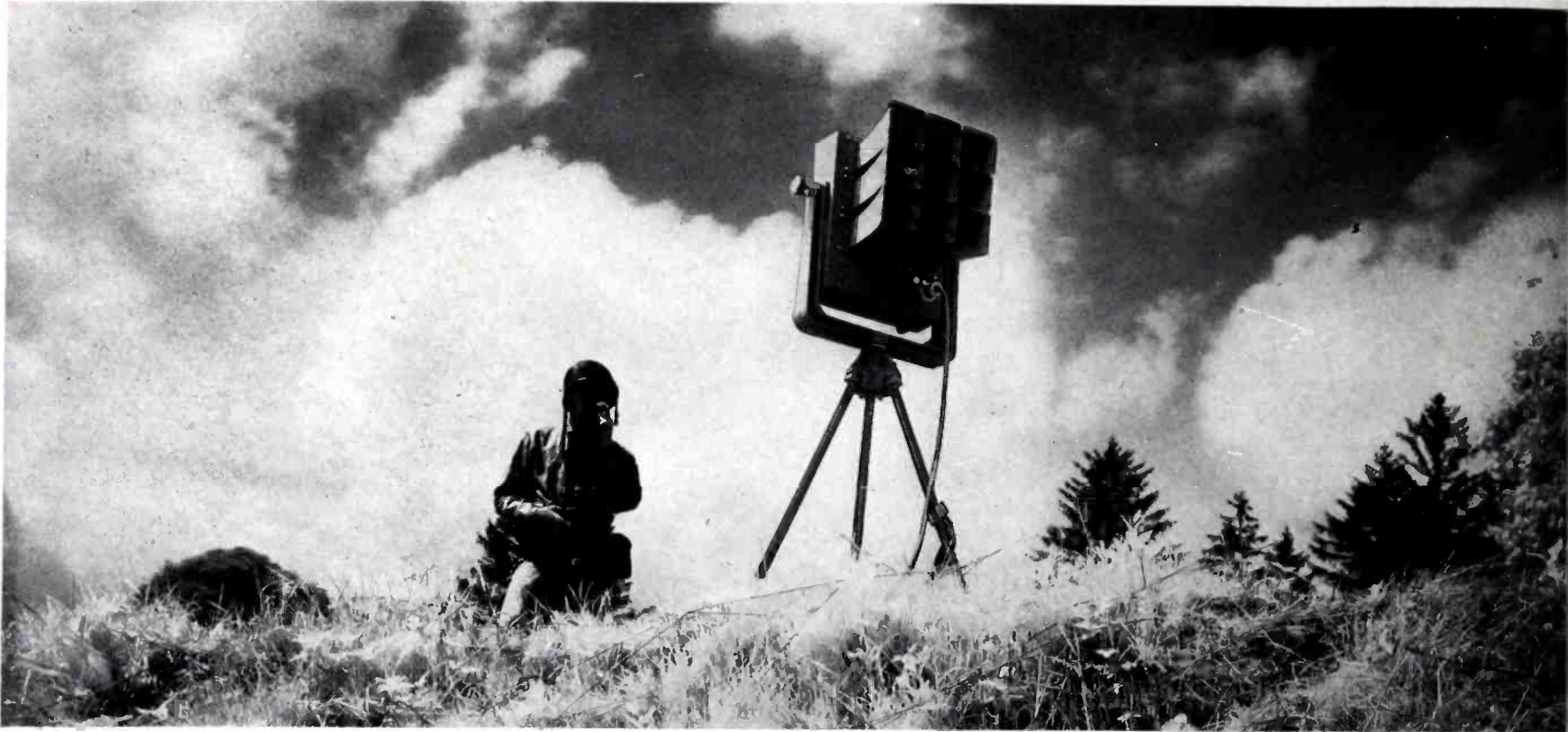
Used on invasion beaches of the Pacific, the Western Electric Beachmaster Announcing System landed with the first waves of fighters. Packaged in six
