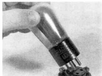
After 1930, tube bases lost side pin, could no longer be bayonet mounted. "Push-in" installation became the standard.
