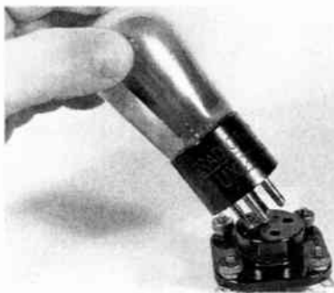
Long contact pins on UX base slid into matching holes in the tube socket.
