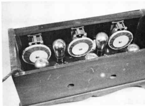
TRF circuitry required the use of three r.f. coils, each tuned by a separate variable capacitor.
