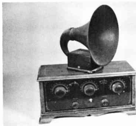
The "3-dialers" offered speaker volume, improved selectivity. They were made in great quantities.
