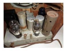
I determined the audio and IF stages worked using a signal generator. With that, I concluded, "Uh Oh, bad oscillator coil," and I was right.
