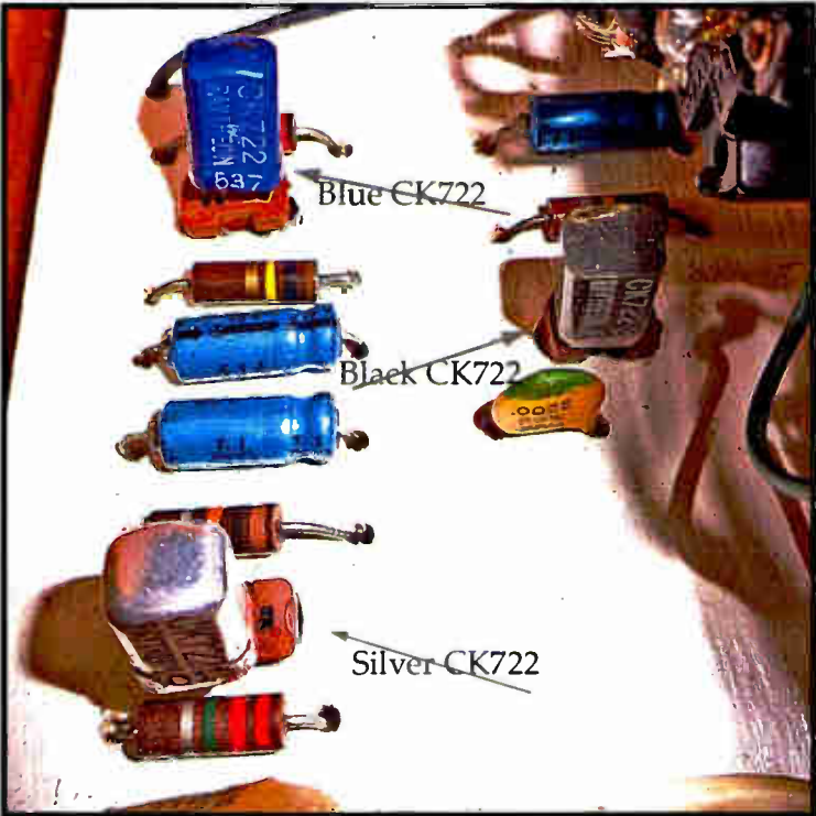
Operating on a single "C" cell battery, this version of a vintage transistor receiver drives vintage headphones with considerable volume.
