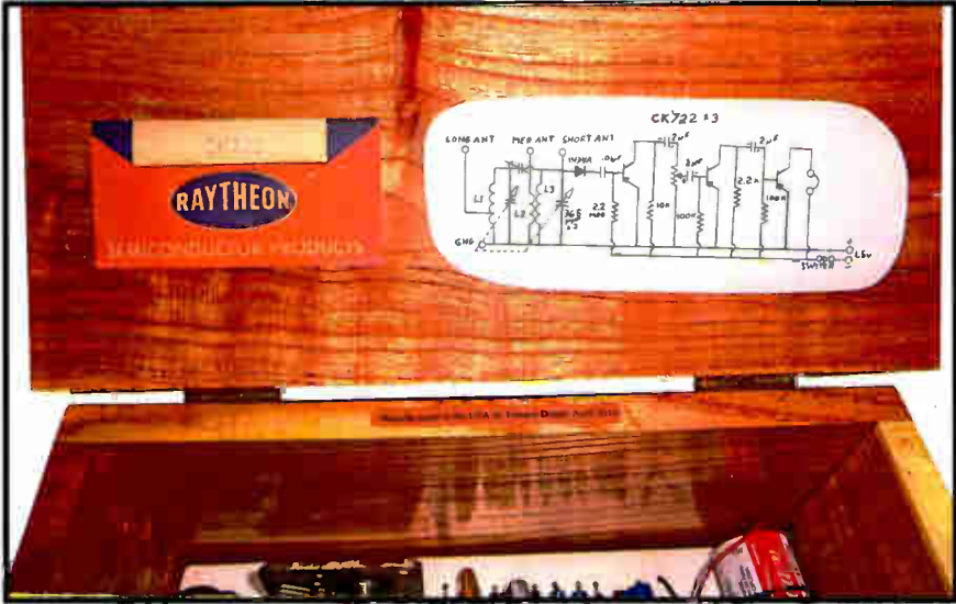
Operating on a single "C" cell battery, this version of a vintage transistor receiver drives vintage headphones with considerable volume.
