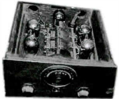
A 1926 Magnavox "Works in a drawer" with ganged tuning capacitors.
