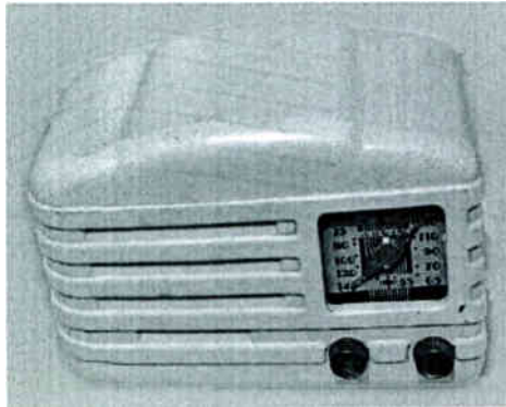
1940, 41 Model 522, chassis RE-76, 5 tubes Color ivory Lighted dial
