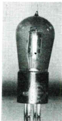
An Arcturus 28. A 15VAC filament four pin triode.
