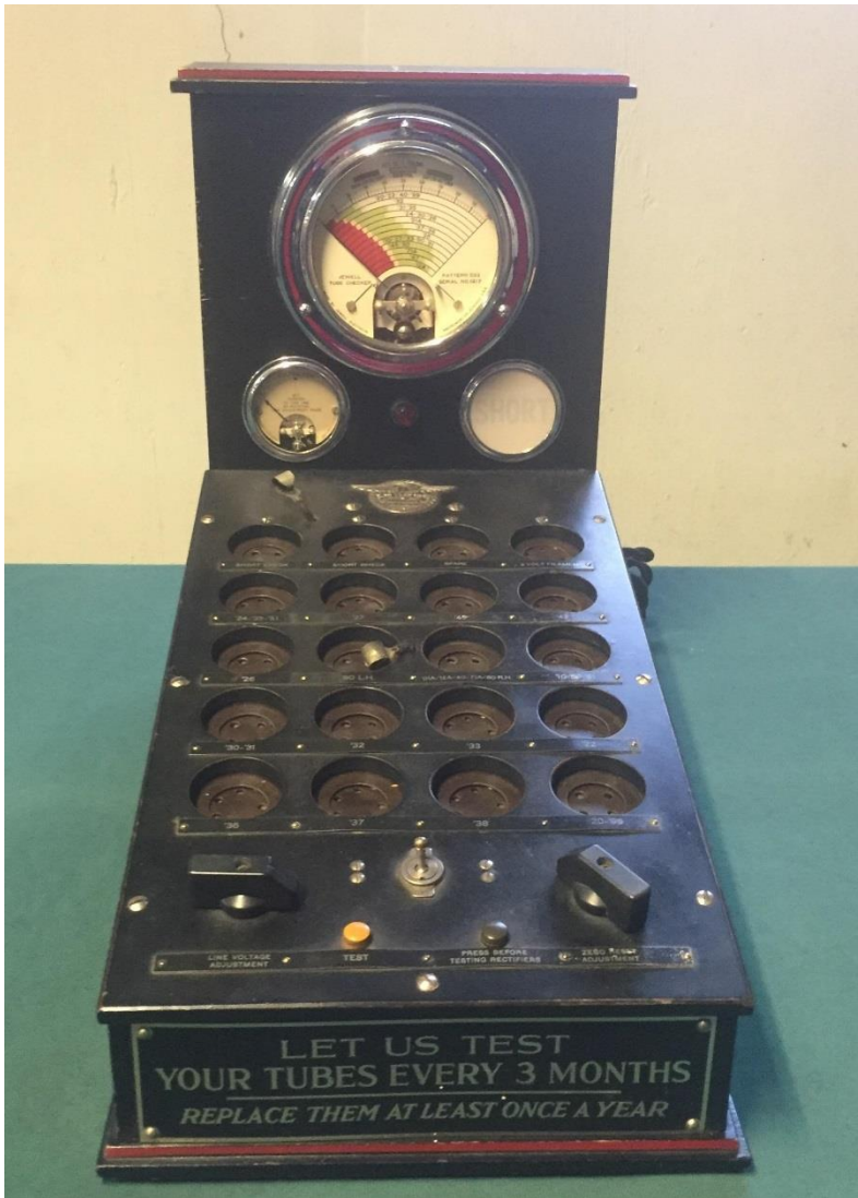
Radio City 310 tester with the post-war upgrade to test miniature and peanut/pencil tubes Larry Osborne Ph.D. (Ret.) K17UFC
