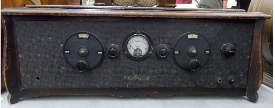
Washington brand battery set. Sold by the D.S. Radio Corp of Seattle. A panel in the top opens up for access to the tubes.
