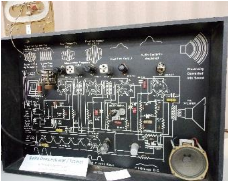
Radio Demonstrator / Trainer – A complete tube radio built into a shadow box! Blake Dietze
