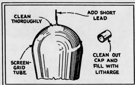
FIG. 10—The loosened cap of a screen-grid tube may be cemented back into place, quite satisfactorily, in the manner shown.
