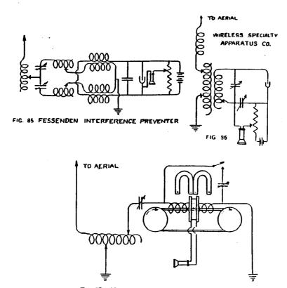
Fig. 87.—Magnetic Detector—Marconi.
