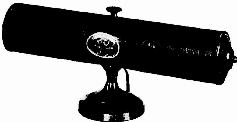
Fig. 2: Antenna with portion of outer covering cut away. Knob for rotating antenna eliminates need to grasp device in region sensitive to hand capacity
