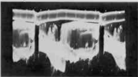
FIG. E. 100 v p-p, vert. freq. CRT input compressed. Source:..... Video input to CRT (cathode) Polarity:..... Sync positive going Amplitude:.. 140 v peak-to-peak
