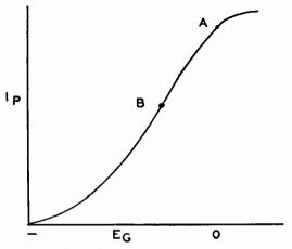
Fig. I. The Eg-Ip characteristic of a typical tube. Point A is the zero-bias point and point B is the normal operating point.
