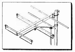
Fig. 4. Telrex "Duplex" yagi for UHF.
