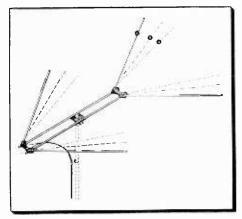
Fig. 5. Ward's U-Vee Antenna. Dotted lines show the different positions into which the elements can be assembled.
