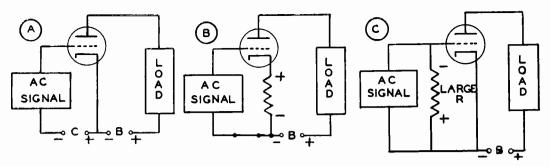
Fig. 2. The three bias methods most frequently used. Explanations are given in the text.
