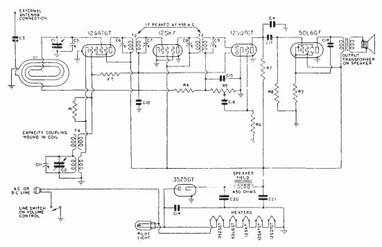
Fig. 1. A typical AC-DC Receiver, the Emerson Model EC.
