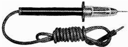
Figure 3. A high voltage multiplier probe that enables you to read voltages as high as 30,000 volts with the Model 45 NRI Professional Volt-Ohm-Mil-Ammeter. Such a probe may be obtained from the NRI Supply Division.
