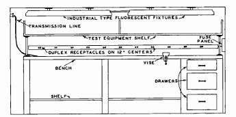
Fig. 3. This is an elevation view showing the television laboratory workbench. Also shown are the test equipment shelf, power facilities, and lighting facilities provided.
