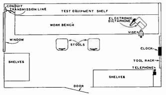
Fig. 2. This is a plan view showing the arrangement of the TV laboratory.
