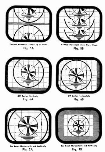
is too small both horizontally and vertically, it may not completely fill the mask as shown in Fig. 7B. In this case, the height control (sometimes called the vertical size or vertical gain control) is adjusted until the proper vertical size is obtained. The width control (sometimes called horizontal size or horizontal gain control) is adjusted until the picture fills the mask horizontally.
