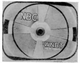
Fig. 3. Rotated pattern-due to improper tube or deflection yoke position.
