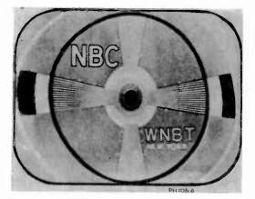
Fig. 11A. Test pattern obtained with horizontal linearity control misadjusted.
