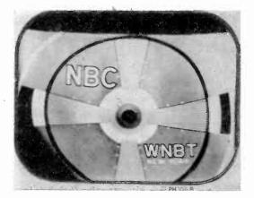
Fig. 2. Test pattern obtained with ion trap magnet and focus coil improperly adjusted.
