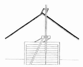
Fig. 9. One type of support used for mounting antenna at peak of gable.
