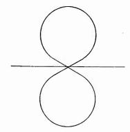
Fig. 3. Antenna pattern for half-wave dipole.
