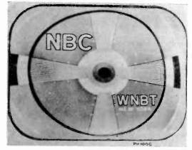
Fig. 11B. Test pattern obtained with horizontal drive control turned too high.
