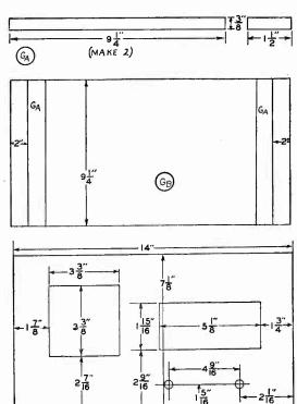
Sketch H (Above). 1/4" 3-ply panel (make 1). Note: Holes for control shafts should be 1/2" diameter.
