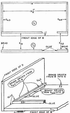
Sketch Fc (Above). Although small nails (brads) are used to reinforce the glued strips, these brads do not show anywhere on the outside of the cabinet.
