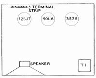
Fig. 4. Parts location—top of master station chassis.
