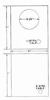
Fig. 3. Front and back panels of remote unit.
