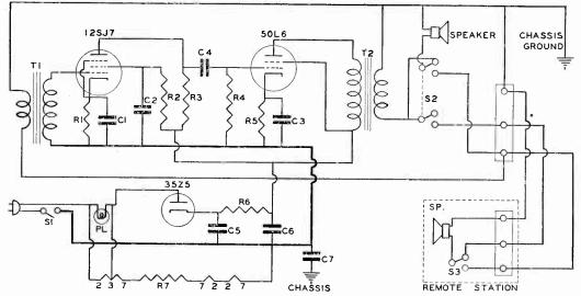
Fig. 1. Schematic diagram of complete "Intercom" System.
