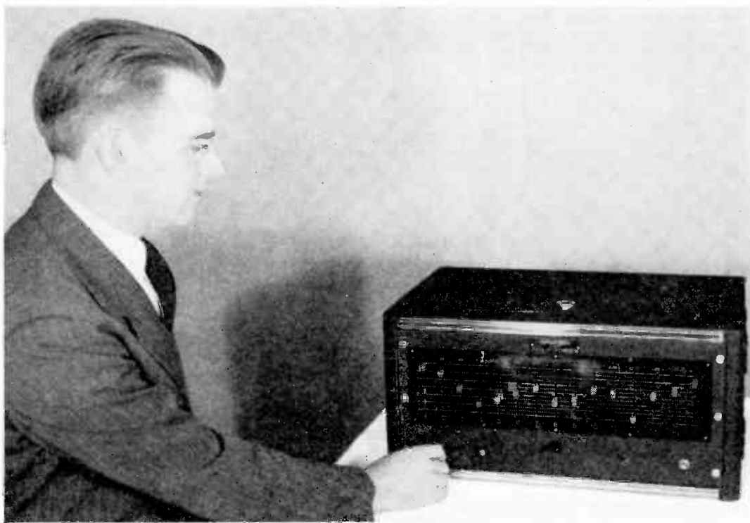
Fig. 8. Paul H. Thomsen, developer of the Tonalizer, demonstrates his latest 15-channel model. The channels are controlled by vertically-sliding levers arranged so the ends of the levers trace out the response curve to which the Tonalizer is set.
