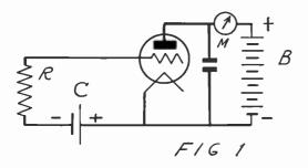
Now consider an ordinary radio stage, using a vacuum tube. Here we have a circuit to which we can apply a voltage and obtain a change in plate current. The ordinary grid circuit can be made to have extremely high resistance and but a small amount of capacity. Hence, if we can arrange this circuit so that it will cover the desired voltage range, we will have our desired instrument.
