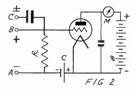
to the voltage and we can now calibrate our meter to read A.C. as well as D.C.
