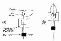
FIG. 4. Egg-shaped cam and plunger mechanism used in the mechanical automatic tuning systems of some Philco receivers.
