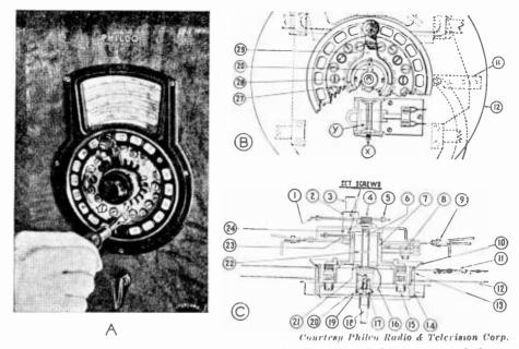
FIG. 2. Three views of an automatic tuning system used on a number of Philco receivers which also have A.F.C. The numbered parts on these diagrams are all identified in the Philco service bulletin on automatic tuning.
