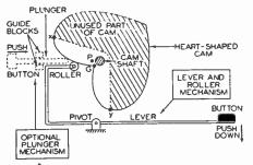
FIG. 3. Operating principles of direct push types of mechanical automatic tuning systems employang a cam with either a lever and roller or a plunger. Pressure on the button in the direction indicated by the heavy arrow serves to rotate the gang tuning condenser (geared to the cam shaft) to the correct setting for the station assigned to that button.
