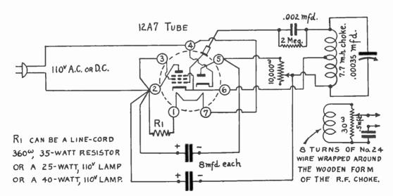
FIG.48C. LOW FREQUENCY MODULATED OSCILLATOR 100-300 K.C.
