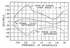
Fig. 2. Comparison of performance of a noisereducing system with conventional antenna of same dimensions.
