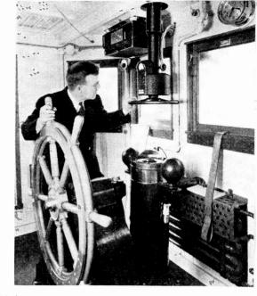
Marine compass installation. Operator has left hand on wheel which rotates the loop installed on the roof of the pilot house. (Photo Western Electric)
