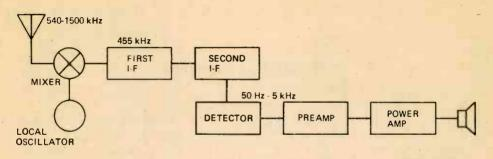
FIGURE 1. SIMPLIFIED BLOCK DIAGRAM OF A TYPICAL AM RECEIVER.
