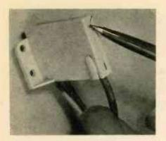
FIGURE 5. THE CRACKS IN THIS FOCUS VOLTAGE DIVIDER INDICATE THAT IT HAS FAILED.
