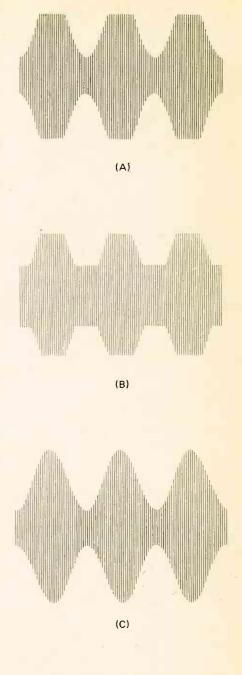
FIGURE 3. (A) NEGATIVE PEAKS OK, (B) BOTH PEAKS CLIPPED, AND (C) NORMAL MODULATION.
