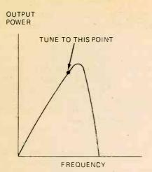
FIGURE 1. PROPER POINT FOR TUNING THE SYNTHESIS OSCILLATOR COIL IN GEMTRONICS GTX-36.
