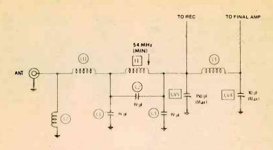
FIGURE 4. RF OUTPUT NETWORK OF GTX2300.
