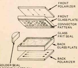
END SOLDER SEAL (ALSO FORMS ELECTRICAL CONNECTIONS BETWEEN PLATES)
