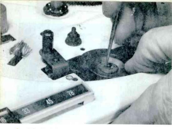
Figure 6. The idler wheel is usually held on its shaft with a small "C" clip which you can remove with the point of an ice pick. Don't lose the clip! Remove the idler wheel and carefully inspect the condition of the rubber drive surface. If it is hard and cracked, it should be replaced. If the surface is hard and slick, but otherwise in good condition, you can rough up the surface with a small file to restore the unit. This is what I did for this particular changer.
