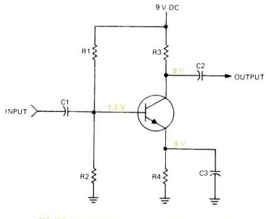
FIGURE 4. A NONCONDUCTING (CUT OFF) TRANSISTOR.
