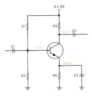
FIGURE 3. A SATURATED TRANSISTOR.
