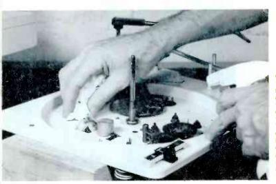
Figure 5. Now go over the top side of the changer with the spray detergent and a paper towel. Do the entire top of the changer base and the tone arm itself. This won't make the changer work any better, but the customer will surely appreciate the neat, almost-new look the cleaning will impart to the machine.
