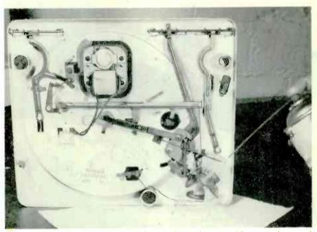
Figure 4. With most of the dirt removed, spray the moving parts with a tuner cleaner and lubricant to remove any deep-down dirt and lint. This will also remove caked grease if done properly.
