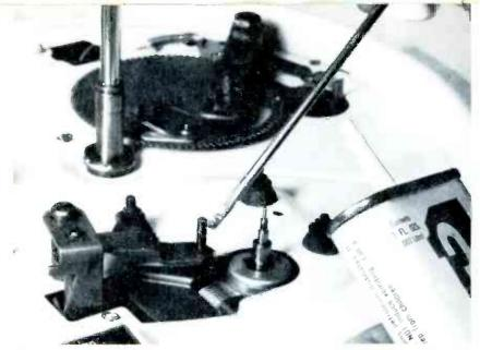
Figure 7. Clean both the hole in the idler wheel and the shaft on which it revolves with your tuner cleaner and then lightly oil both the shaft and the hole in the wheel. Reinstall the idler wheel and the "C" clip and spin the wheel to make sure it turns freely.
