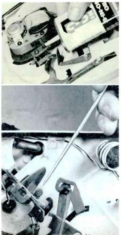
Figure 11. Parts that slide freely should be given a drop of oil. Give the various springs a drop of oil to prevent the formation of rust. Some moving parts should not receive any type of lubricant at all. One such part is the clutch pad being pointed to with the ice pick. While you have the oil and grease out, be sure to put a little of both on the turntable shaft as well as in the hole of the turntable (see Figure 3).
