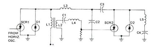
FIGURE 3. SIMPLIFIED SCHEMATIC OF HORIZONTAL SWEEP.
