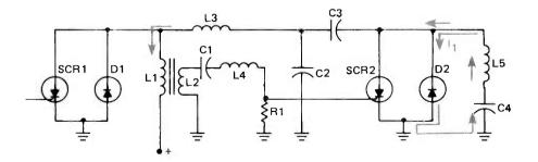
FIGURE 5. CURRENT FLOW THROUGH YOKE AND D2 AT T1.
