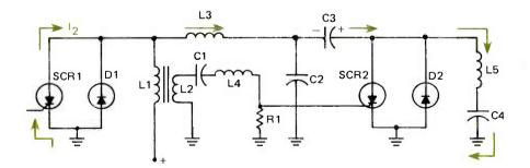
FIGURE 9. CURRENT FLOW DURING THE INTERVAL T5 TO T6. NOW ONLY SCR1 IS CONDUCTING.
