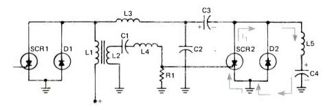
FIGURE 6. CURRENT FLOW AT THE START OF THE SECOND HALF OF THE TRACE CYCLE, JUST AFTER T2.
