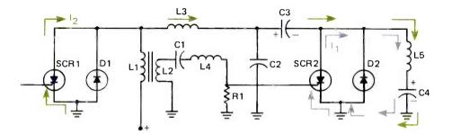
FIGURE 7. CURRENT FLOW DURING THE INTERVAL T3 TO T4 WHEN BOTH SCR'S ARE CONDUCTING.
