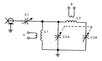
FIGURE 1. MULTIBAND COUPLER.
