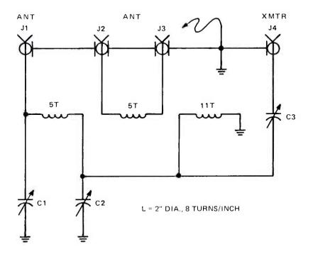
FIGURE 3. FINAL VERSION OF THE MULTIBAND COUPLER.
