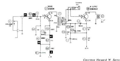
FIGURE 5. AUDIO SECTION OF SEARS MODEL 5024
