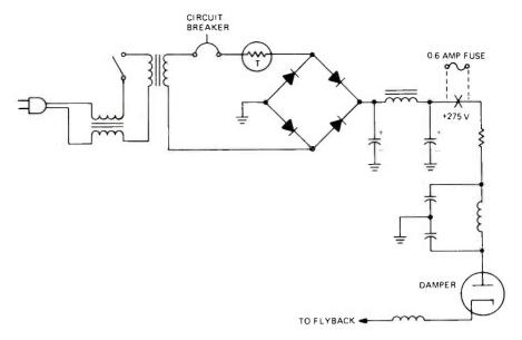
FIGURE 1. POWER SUPPLY AND DAMPER IN PHILCO 21ST90.
