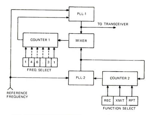
FIGURE 1. BASIC OPERATION OF PROGRAMMABLE FREQUENCY SYNTHESIZER.
