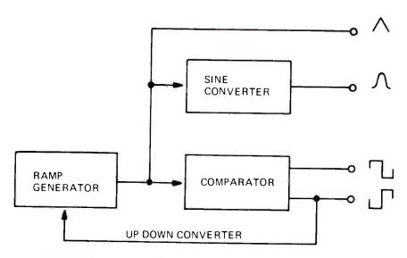
FIGURE 1. BLOCK DIAGRAM OF BASIC FUNCTION GENERATOR.
