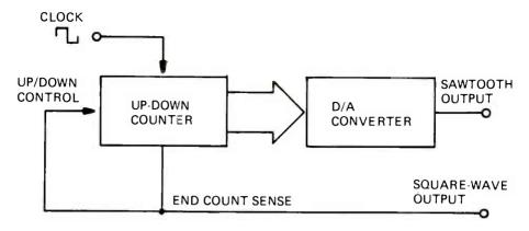
FIGURE 5. BASIC DIGITAL FUNCTION GENERATOR.
