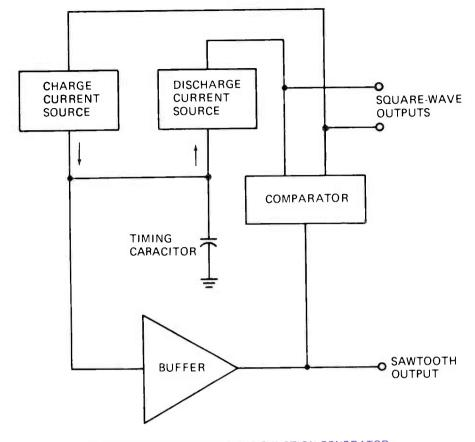
FIGURE 2. THE HEART OF THE FUNCTION GENERATOR.
