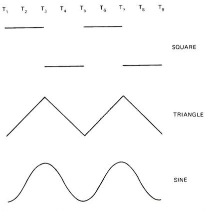
FIGURE 4. PULSE RELATIONSHIPS OF FUNCTION GENERATOR WAVEFORMS.
