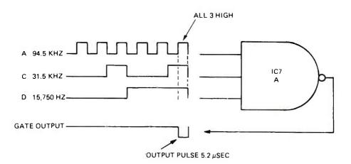
FIGURE 7. GENERATION OF THE HORIZONTAL SYNC SIGNAL.
