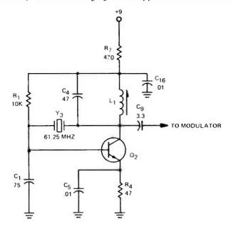
FIGURE 10. SCHEMATIC DIAGRAM OF THE CARRIER OSCILLATOR.
