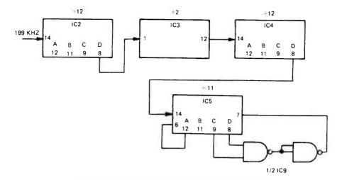
FIGURE 6. BLOCK DIAGRAM OF THE DIVIDER CHAIN.
