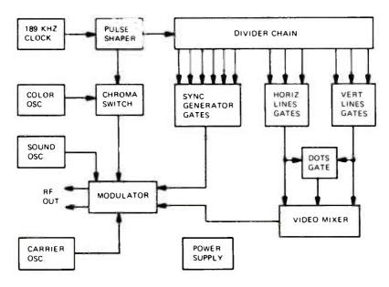
FIGURE 3. SIMPLIFIED BLOCK DIAGRAM OF THE TV PATTERN GENERATOR.
