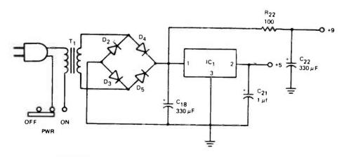
FIGURE 4. SCHEMATIC DIAGRAM OF THE POWER SUPPLY.
