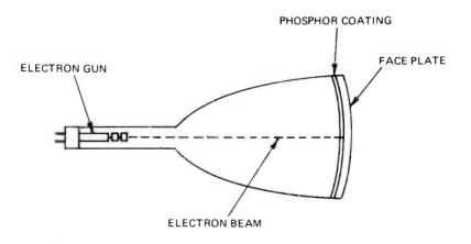
FIGURE 2. SIMPLIFIED DRAWING OF A TELEVISION PICTURE TUBE.
