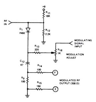
FIGURE 11. SCHEMATIC DIAGRAM OF THE DIODE MODULATOR.
