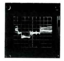
FIGURE 4. SAME SIGNAL EXPAN-DED TO 1 MICROSECOND/CM.
