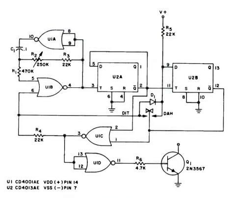
FIGURE 1. SCHEMATIC OF ORPP KEY.
