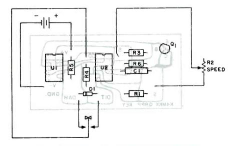
FIGURE 3. COMPONENT LAYOUT FROM TOP OF CIRCUIT BOARD.
