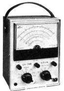
Performs all measurements with a single probe. Input Impedance of 11 megohms reduce loading effects. The AC range is usuable to 4MHz. Large meter face for easy reading.
