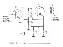
Fig. 4. Detail of Fig. 3, showing automatic shutdown circuit.
