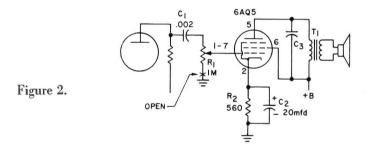
I found by looking at a diagram at the wholesalers (most will let you do this at no charge) that the volume control was 1 megohm. I got a suitable replacement and installed it, which reduced the grid-to-chassis voltage of the 6AQ5 to zero as expected.
