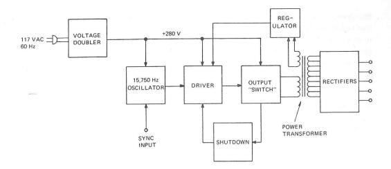
Fig. 3. Block diagram of power supply used in 1972 "QUASAR" by Motorola.
