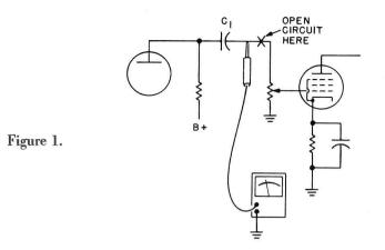
resistance of the 6AQ5 grid return was the same as that of the vtvm input resistance, 12.2 megohms. The grid return resistance should have been between 250,000 ohms and 1 megohm. The measured resistance was well over 200 megohms! An examination showed the circuit to be as shown in Fig. 2.
