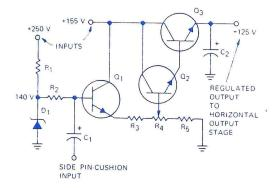
Fig. 1. Simplified diagram of +125V power supply used in Zenith solid-state color TV.
