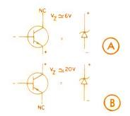
Fig. 8. Substitution of an ordinary transistor for a low-voltage Zener (A), or a high-voltage Zener (B).
