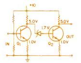
Fig. 6. Zener diode used as dc level shifter in direct-coupled amplifier.
