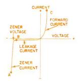
Fig. 1. Relationship between voltage and current in a Zener diode.
