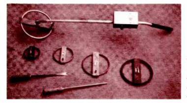
Fig. 2. A beatfrequency metal locater with interchangeable coils and digging-tool accessories. diagram of a typical unit is shown in Fig. 3. The oscillators are generally Colpitts or Hartley. The search coil is the inductive tuning component for one oscillator; the other is tuned by an adjustable rf coil. Sometimes a tuning capacitor is used to tune the oscillator instead of an adjustable coil. This, however, depends on the type of oscillator.
