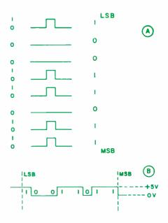
Fig. 1. Parallel (A) and serial representation (B) of the binary word 11011001.
