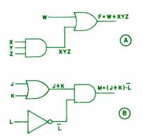
Fig. 5. Two examples of combined logic gates.
