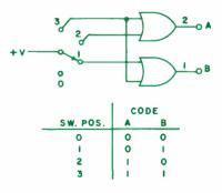
Fig. 8. An encoder that generates four 2-bit codes.
