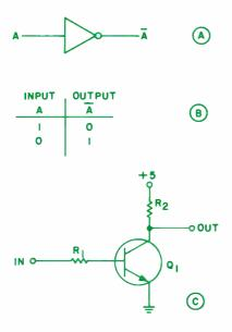
Fig. 2. Inverter symbol (A), truth table for the inverter (B), and a typical inverter circuit (C).
