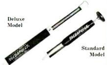
SOLDAPULLT is the best resoldering tool we've seen vet. This tool incorporates easy handling, swift vacuum action and a self cleaning feature. Soldapullt is loaded by pushing plunger knob down until it latches. Molten solder is drawn into its cylinder instantaneously with a high impulsive vacuum by release of the spring loaded piston.
