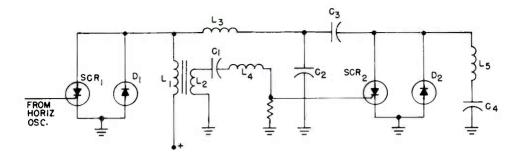
Fig. 3. Simplified schematic of horizontal sweep.
