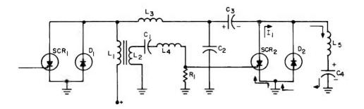
Fig. 6. Current flow at the start of the second half of the trace cycle, just after  $T_{2^{12}}$
