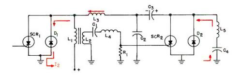
Fig. 10. Current flow during the interval  $T_6$  to  $T_7$  when  $D_1$  is conducting.
