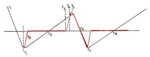
Fig. 4. The horizontal trace and retrace cycle.
