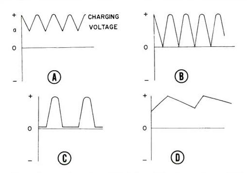
Fig. 2. Power supply waveforms. (A) Full-wave ripple with capacitor and load.
