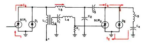
Fig. 8. Current flow during the interval  $T_4$  to  $T_5$  when  $SCR_1$  and  $D_2$  are conducting.
