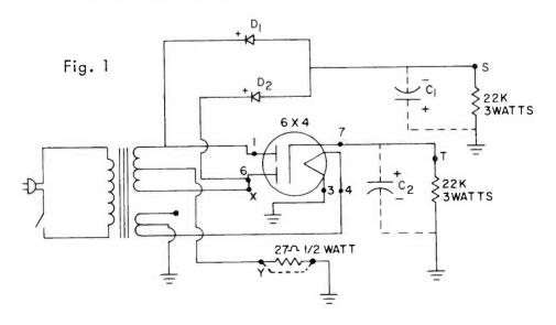
lead to the chassis and the probe to the ungrounded terminal of the .25 mfd capacitor. Turn on the equipment and wait 30 seconds or so for the 6X4 to warm up. Touch T with the lead you have soldered to the capacitor terminal and hold it there while you read the meter. It should read between 60 and 70 volts.
