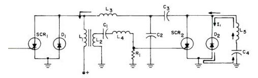
Fig. 5. Current flow through yoke and  $D_2$  at  $T_1$ .
