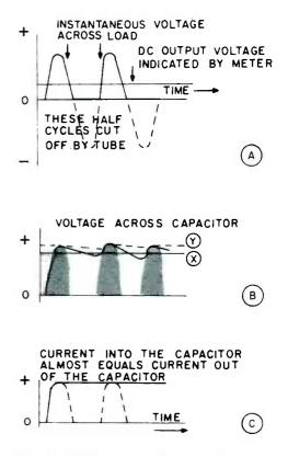
Fig. 3. Voltage waveforms at the output of a half-wave rectifier. (A) resistor alone is used; (B) load discharges the capacitor; (C) output capacitor fed through choke or resistor.
