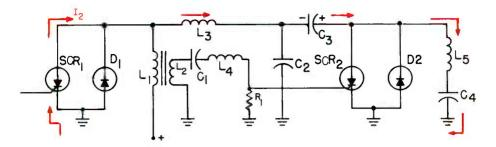
Fig. 9. Current flow during the interval T<sub>5</sub> to T<sub>6</sub>. Now only SCR<sub>1</sub> is conducting.
