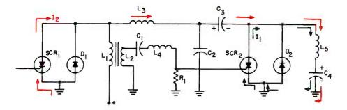
Fig. 7. Current flow during the interval  $T_3$  to  $T_4$  when both SCR's are conducting.
