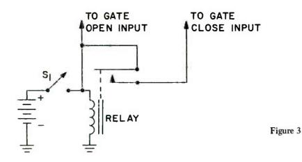
easily done with our time-interval circuit of Fig. 2. The exact setup may appear as shown in Fig. 3. When  $S_1$  is closed, the battery voltage will be applied to the relay coil. Due to the inductance of the coil, the current does not follow the applied voltage. There is a time lag between the initial application of coil voltage and the time where current increases to the point where the coil pulls the relay contacts closed.
