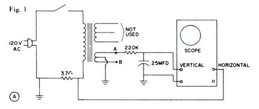
primary current can be disregarded. My first thought was to use a 5-ohm, .5-watt resistor, but my junk box came up with a 3.7-ohm, 5-watt resistor that worked just as well.
