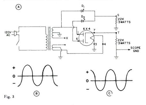
Now remove lead X from socket pin 6, and let's see how these pulses appear across the load after rectification. Set the scope Vertical Attenuator and the Vertical Gain control to 10X to produce a display about 2" high. The output will look like Fig. 3D, while the full-wave connection produces the waveshape shown in Fig. 3E.
