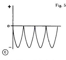
polarity of the rectified pulses by measuring between the chassis and points T and S with a dc voltmeter. You should measure between 50 and 60 volts dc in either case. However, you will find point T positive with respect to the chassis, while point S is negative.
